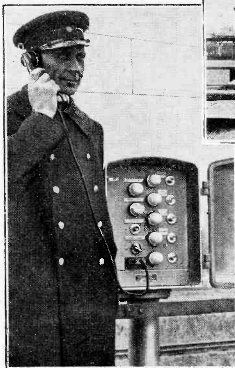
The transmitter is installed in a special housing alongside the track. On the left the shunting official is seen using one of the special control boxes to communicate with the engine-driver.
