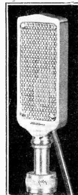
makes use of four parallel ribbons connected in series. It has a frequency response from 50-10,000 cycles and a sensitivity of -45 db. The transformer is designed to match a 200-ohm line.
