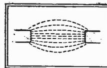
Fig. 2.—Illustrating the spreading of a magnetic field.
