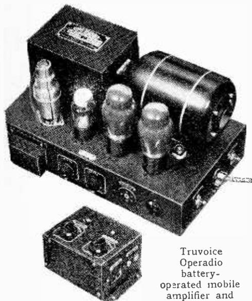
Truvoice Operadio battery-operated mobile amplifier and control unit.
