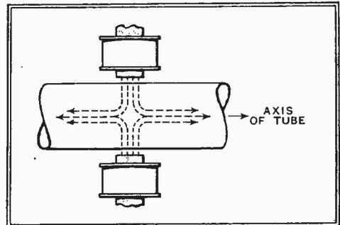
Fig. 5.—Illustrating de-focusing effect with push-pull deflection.
