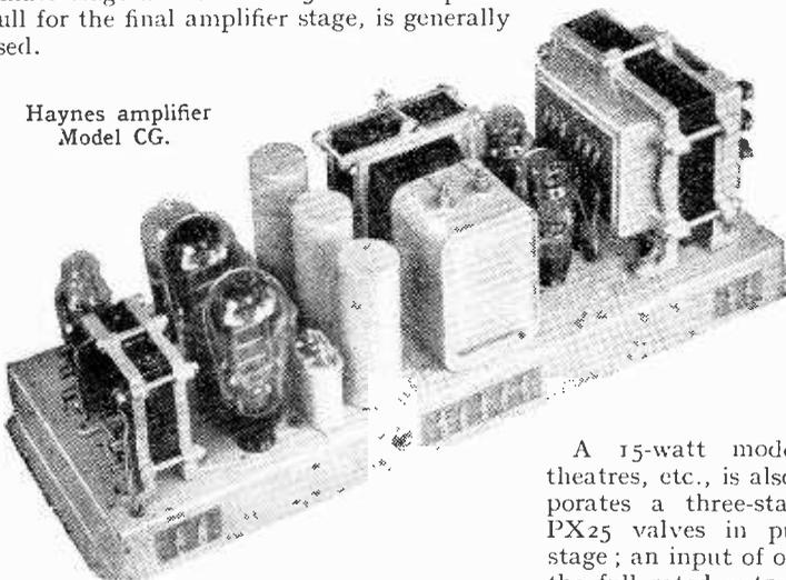
A general-purpose amplifier built in chassis form and fitted with two PX25 valves giving 14 watts output is made by Hartley Turner Radio, and this model will meet many of the requirements of PA work.
