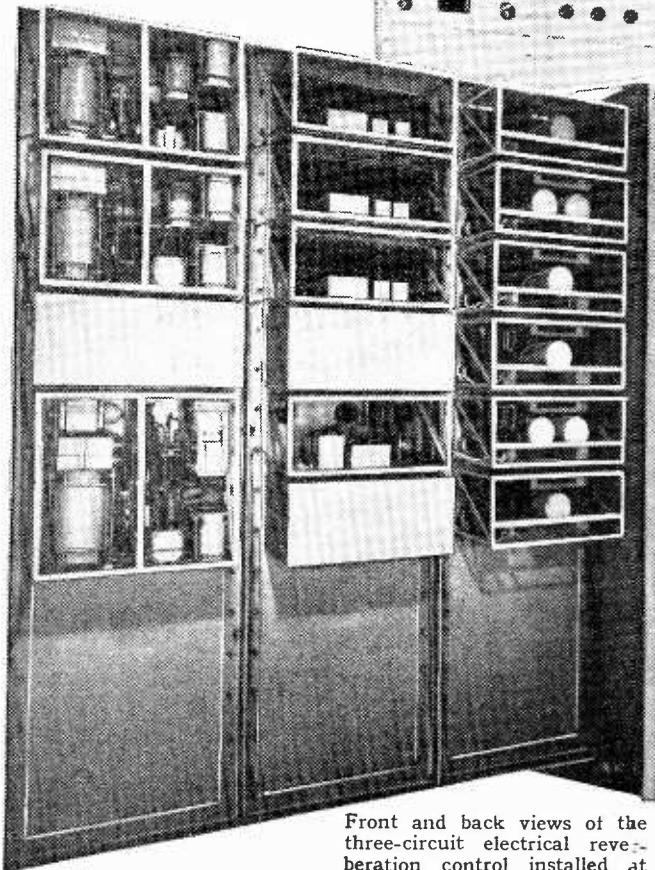
Front and back views of the three-circuit electrical reverberation control installed at Poste Parisien.
