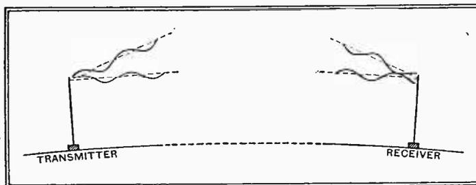
Fig. 1.—A transmitter is sending out identical waves in all directions; of these, two may find their way to a single receiving aerial, and it is a toss-up whether they arrive in such a way as to help one another or (as shown here) cancel one another out.
