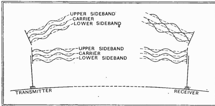
Fig. 2.—When even the simplest "programme"—a pure tuning note—is being radiated, there are three sets of waves of slightly different length. It is the differing lengths that make it possible for the sidebands to be reinforced and the carrier washed out (as here) or vice versa. The slight differences in wavelength between carrier and sidebands cannot be correctly indicated.
