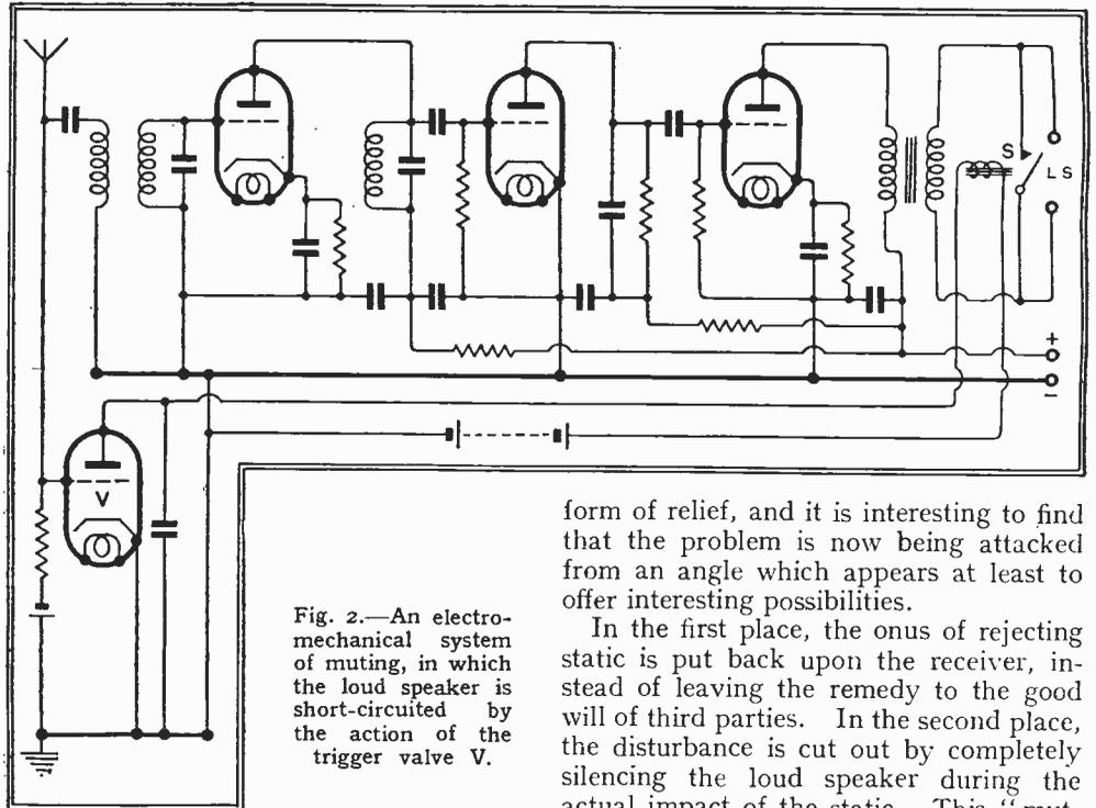
Fig. 2.—An electro-mechanical system of muting, in which the loud speaker is short-circuited by the action of the trigger valve V.
