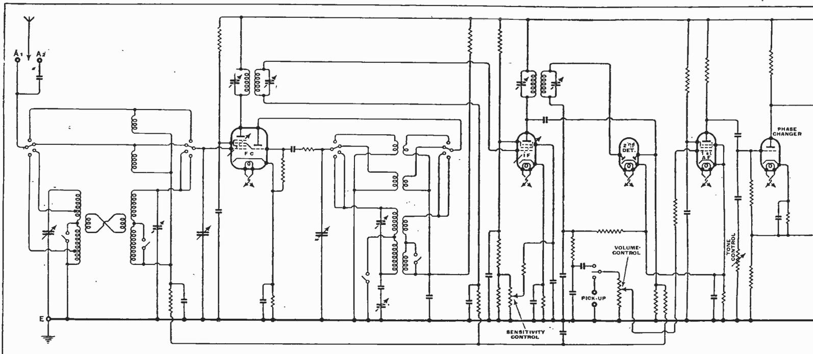
speaker which is connected through by-pass condensers in parallel with the primary winding of the main output transformer. The receiver is built on a light but rigid spot-welded steel chassis finished in grey enamel.
