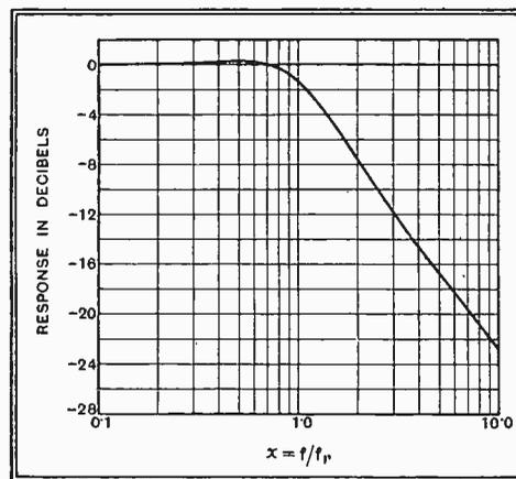
Fig. 10.—The response curve of the amplifier of Fig. 9 is shown here, the bottom scale being in frequency ratios.
