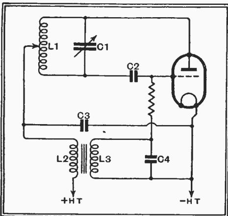
Fig. 1. Circuit of the modulated RF oscillator.
