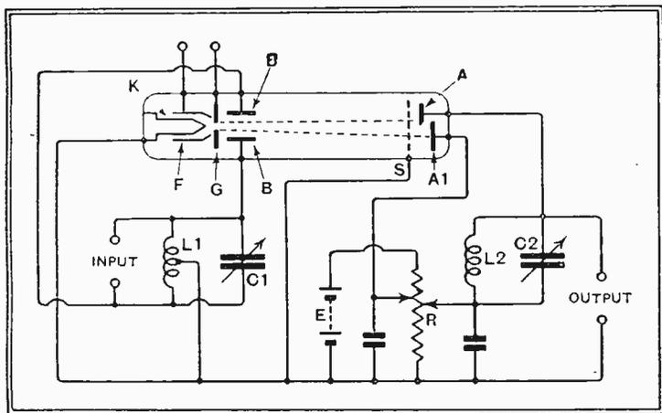
Fig. 1.—The simplest deflection valve circuit, as arranged for RF amplification.
