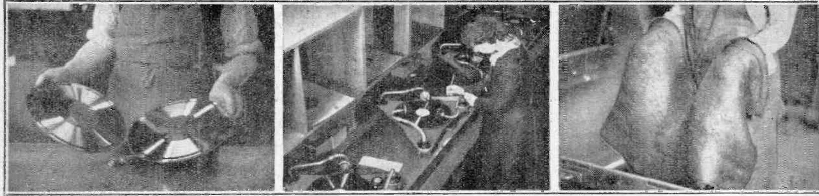
The new negative, which will be used for pressing records, is now stripped from the original positive, and sample records made from this are next tested for wear and passed through cooling conveyers preparatory to being cut into "biscuits" of the correct shape and size for 10-
