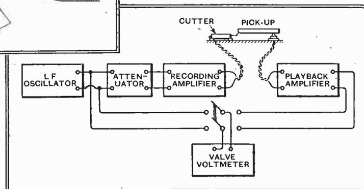
Fig. 2.—Connections of apparatus for measuring overall response.
