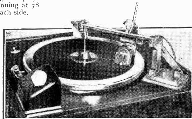
The Permarec Junior home recorder showing also the motor-unit and level indicator.
