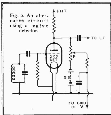
Fig. 2. An alternative circuit using a valve detector.
