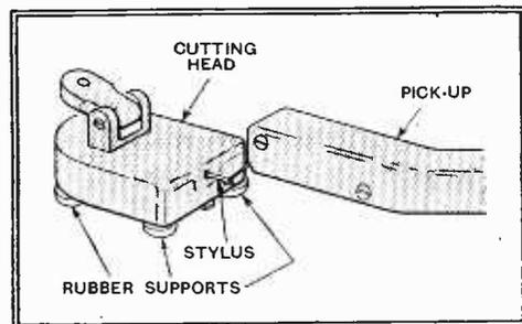
Fig. 1.—Details of set-up for measuring frequency characteristics.
