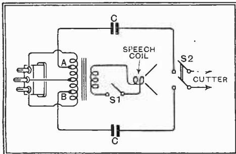
Fig. 2.—A ready change-over from loud speaker to cutter can be made by adopting these connections which are explained in the text.
