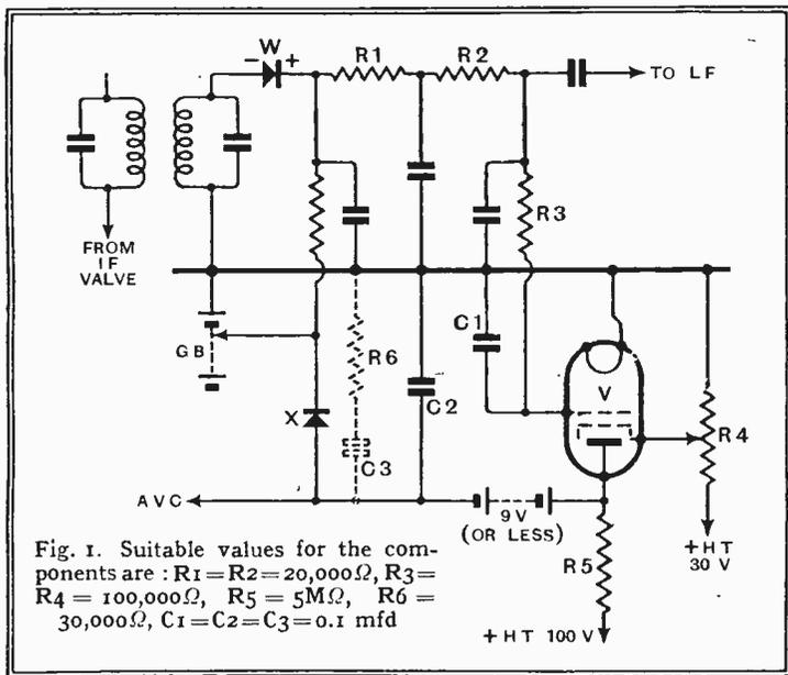
Fig. 1. Suitable values for the components are:  $R_1=R_2=20,000\Omega$ ,  $R_3=R_4=100,000\Omega$ ,  $R_5=5M\Omega$ ,  $R_6=30,000\Omega$ ,  $C_1=C_2=C_3=0.1$  mfd
