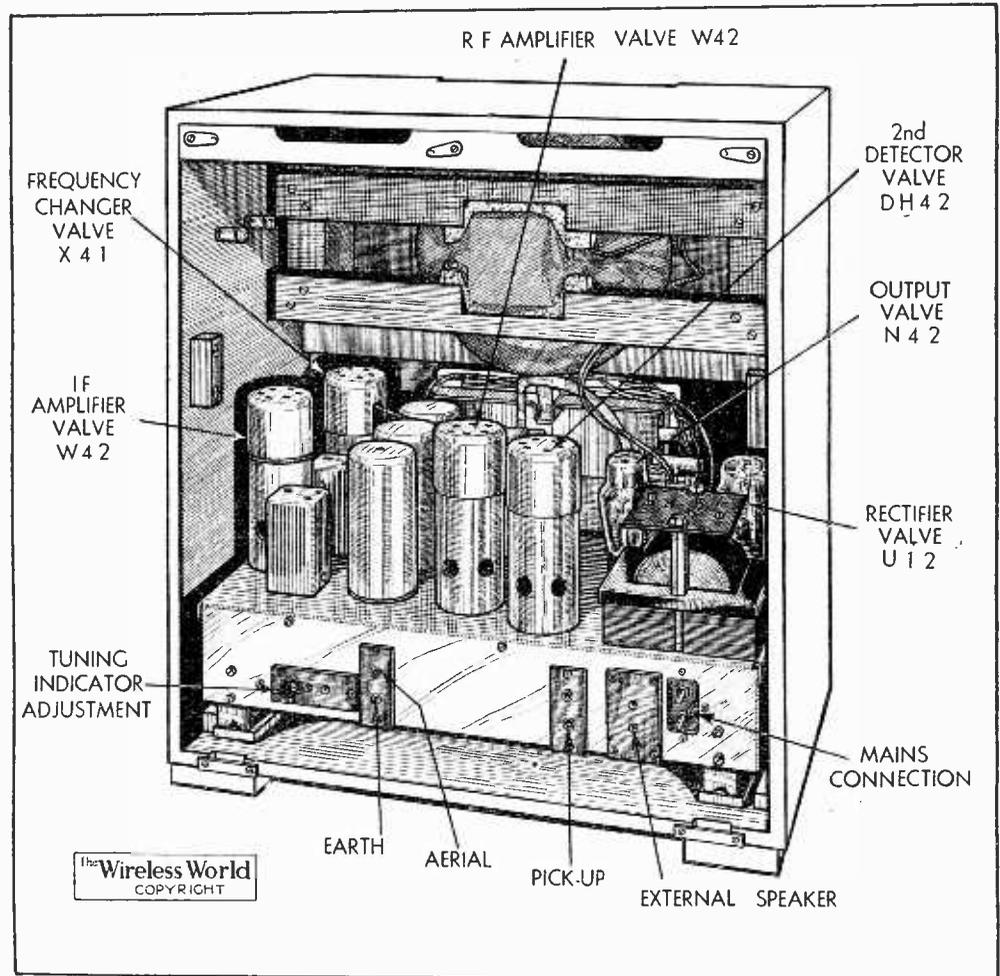
Both chassis and loud speaker are mounted on rubber to guard against microphony.
