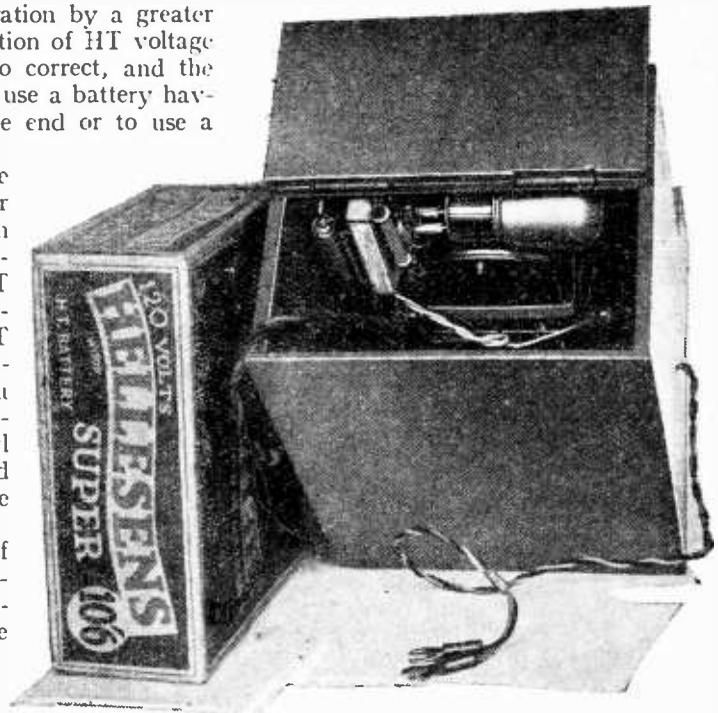
With the exception of the LT battery, the meter is self-contained. The components are secured to the top panel, and space is provided for the HT battery in the base of the container.
