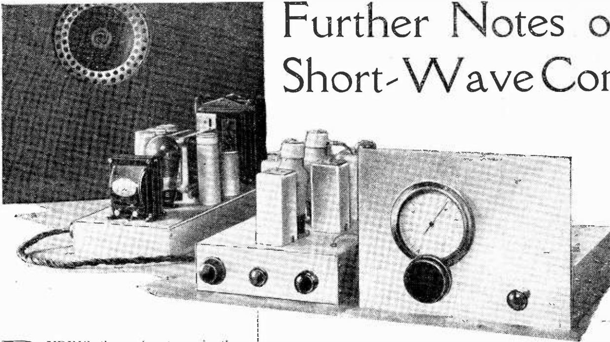
AC Short-Wave Converter arranged for use with the Experimenter's IF amplifier.
