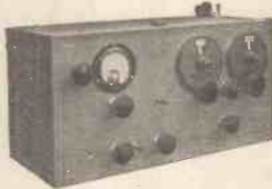
Belling-Lee noise measuring set to B.S.S. 727, fundamentally a 5 valve superheterodyne receiver. With variable alternators totalling 136 db. in 6 db. steps.
