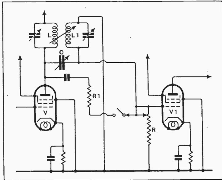
Circuit arrangement for control of selectivity in IF amplifier.
