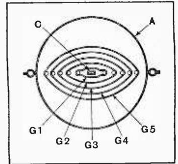
Electrode assembly for a frequency-changing valve.
