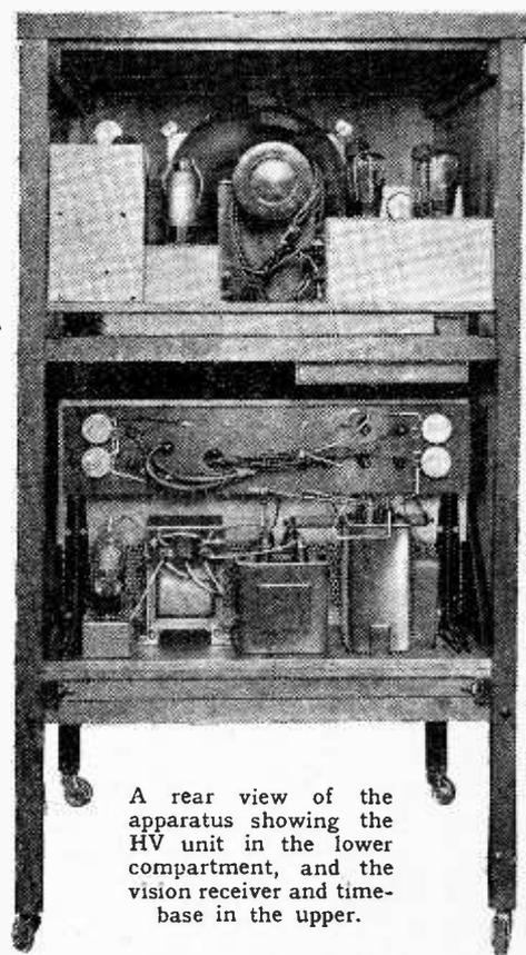
A rear view of the apparatus showing the HV unit in the lower compartment, and the vision receiver and time-base in the upper.
