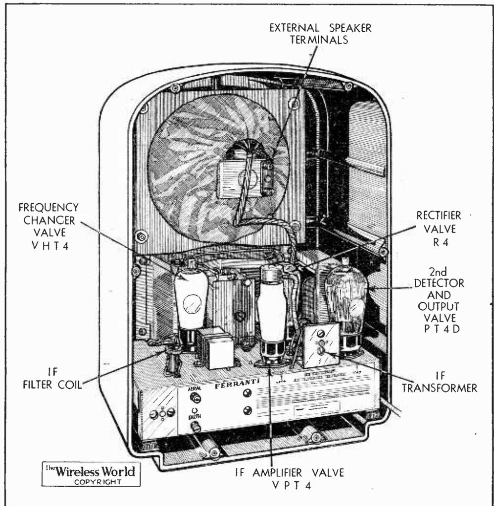
By careful disposition of the components above and below the chassis it has been found possible to dispense with screening cans for all coils, with a consequent increase in efficiency.
