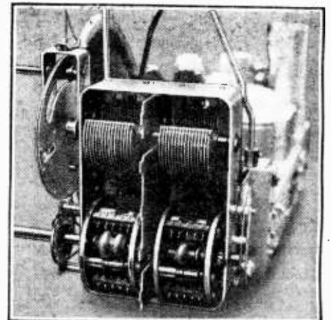
The Ondia tuning unit comprises a switch-coil "ensemble."
