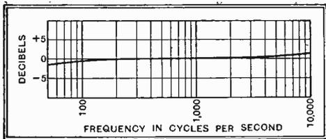
Fig. 5.—Overall frequency characteristic of amplifier.
