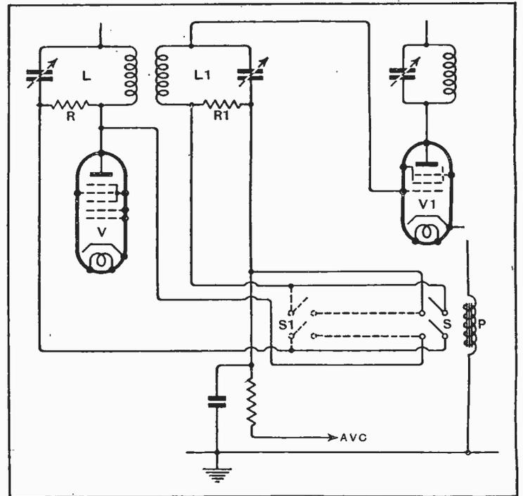
IF amplifier circuit for automatic and manual control of selectivity.
