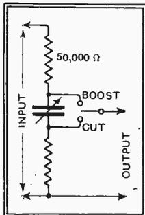
Fig. 2.—Circuit for bass control.
