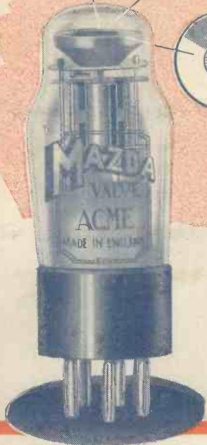
The Mazda AC.ME enables exceedingly accurate tuning of a receiver to be obtained by purely electrical means. It consists of an electrode system surmounted by a target coated with a fluorescent material. The area of glow on the target is controlled by the bias applied to the control grid of the electrode structure.
