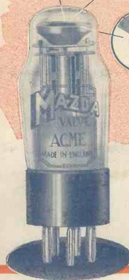
The Mazda AC.ME enables exceedingly accurate tuning of a receiver to be obtained by purely electrical means. It consists of an electrode system surmounted by a target coated with a fluorescent material. The area of glow on the target is controlled by the bias applied to the control grid of the electrode structure.
