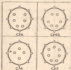
Four different types of Coil Bases, threaded and unthreaded, are available and all are moulded in "R.D.4" dielectric.
