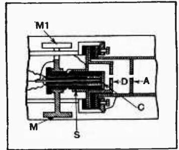
Constructional details of C.R. tube with adjustable cathode.
