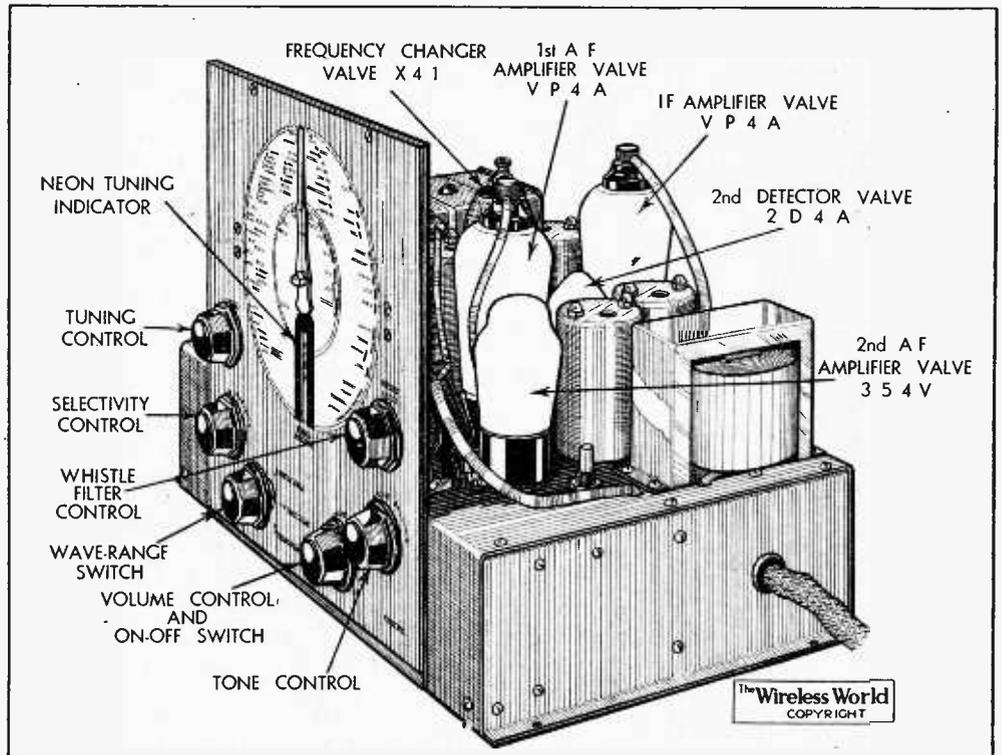
Controls are clearly marked and mounted on the large ivorine tuning panel.
