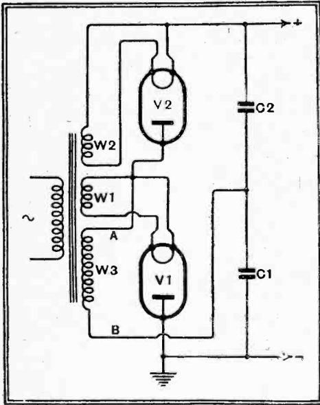
Fig. 35.—For a given output voltage, the lowest voltages between windings are obtained with the voltage-doubler circuit shown here.
