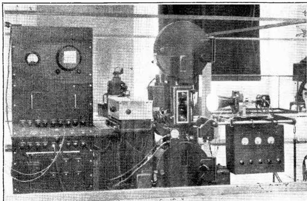
The Cossor film transmitter which is used to provide a signal for demonstrations when the Alexandra Palace is not operating.
