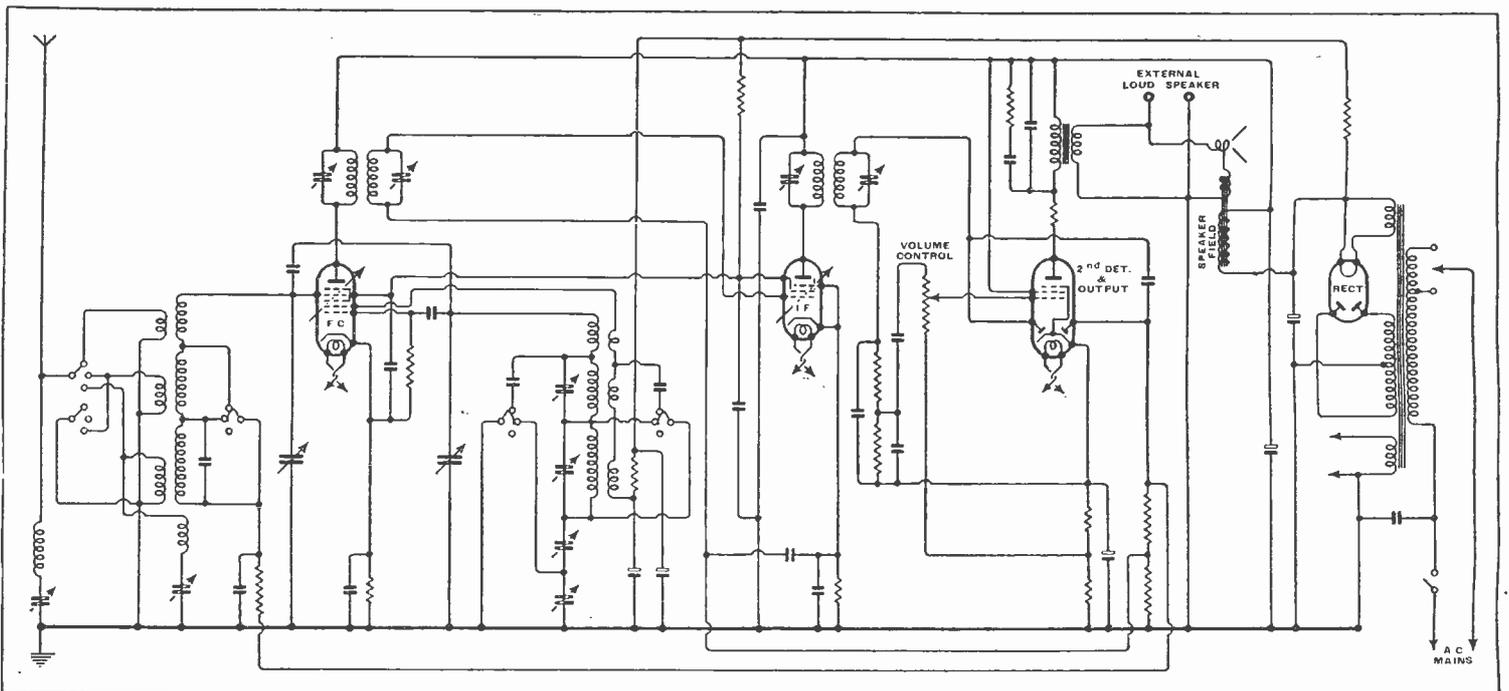
Although the superheterodyne circuit makes use of only three valves it has a remarkably efficient performance, particularly on long waves.
