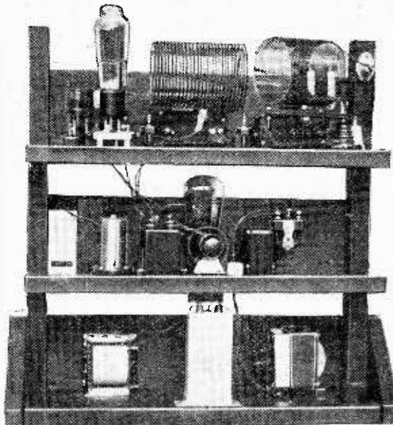
Rear view of the transmitter: immediately to the left of the oscillator valve on the top shelf is the combined grid coil and crystal holder; a valve base is used for this purpose.
