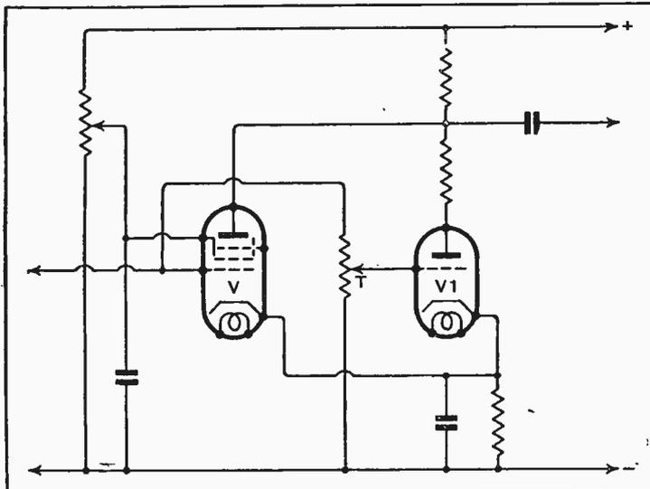
Arrangement of amplifying valves in television apparatus to correct for distortion.
