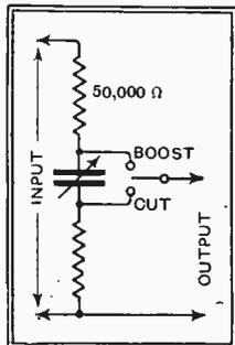
Fig. 2.—Circuit for bass control.
