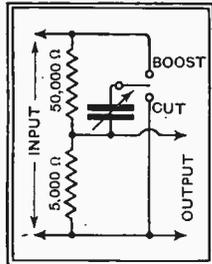
Fig. 1.—Principle of the simple tone-correction circuit discussed.
