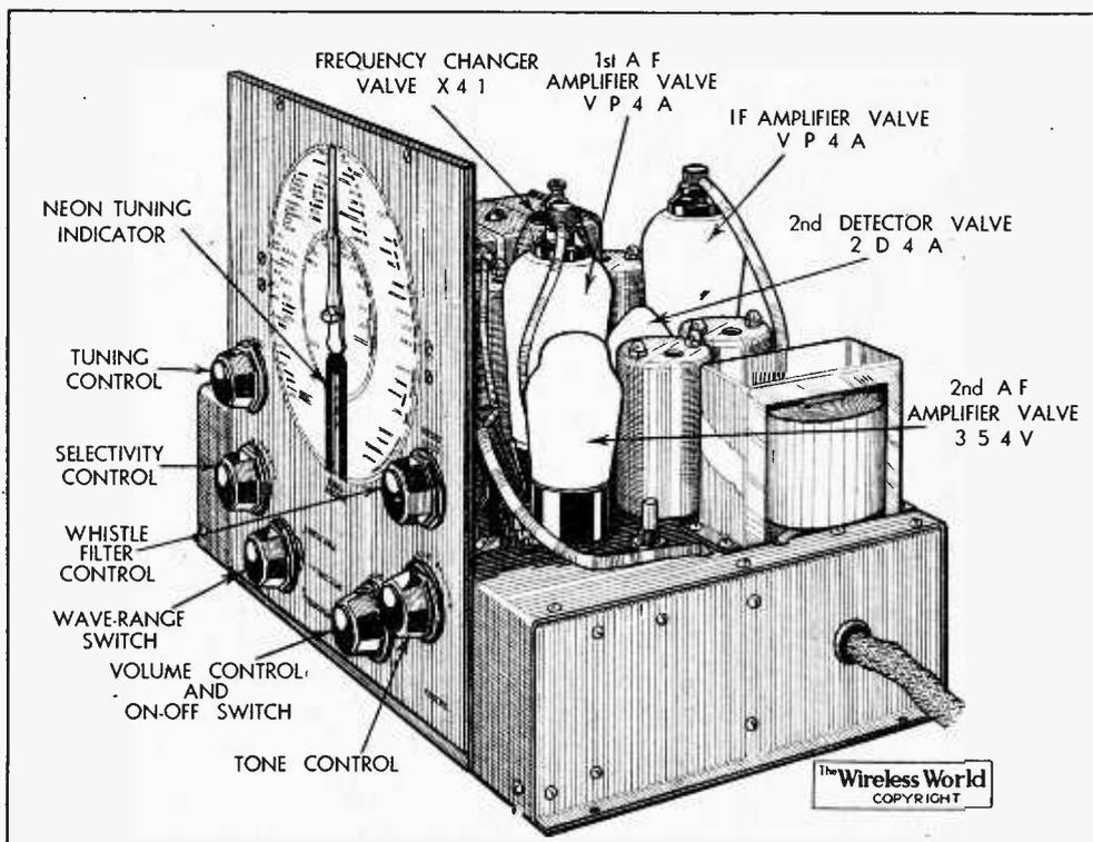
Controls are clearly marked and mounted on the large ivory tuning panel.
