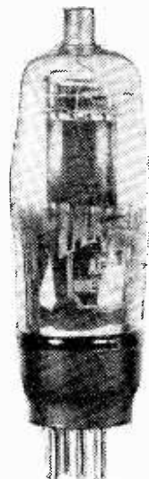
Mazda AC/P4 triode for time-base work.
