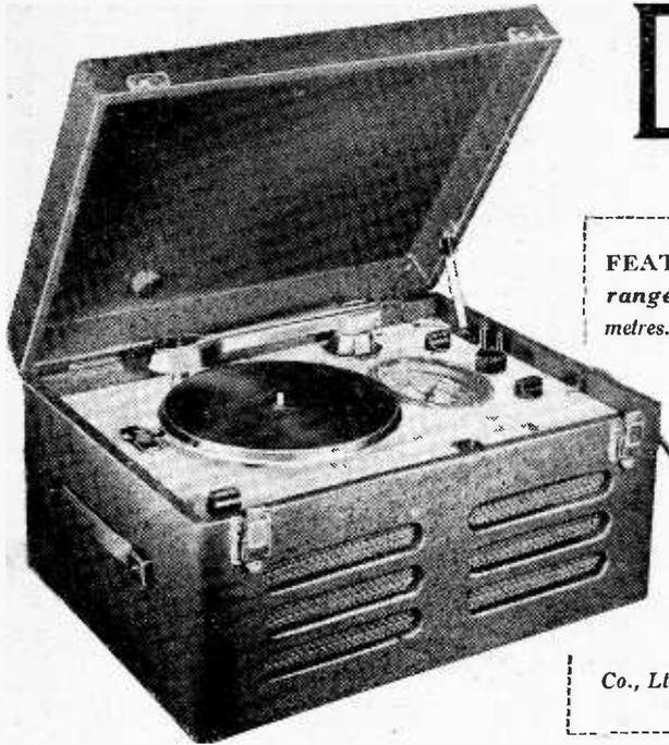
**FEATURES.** *Weight.*—27 lb. *Wave-ranges.*—(1) 19-49 metres. (2) 200-550 metres. (3) 1,000-2,000 metres. *Circuit.*—Triode-hexode frequency-changer—var.-mu pentode IF amplifier—double-diode second detector—pentode output valve. *Controls.*—(1) Tuning. (2) Volume and on-off switch. (3) Waverange. (4) Tone. (5) Motor switch. (6) Mains voltage adjustment. *Price.*—16½ guineas. *Makers.*—Decca Gramophone Co., Ltd., 1/3, Brixton Road, London, S.W.9
