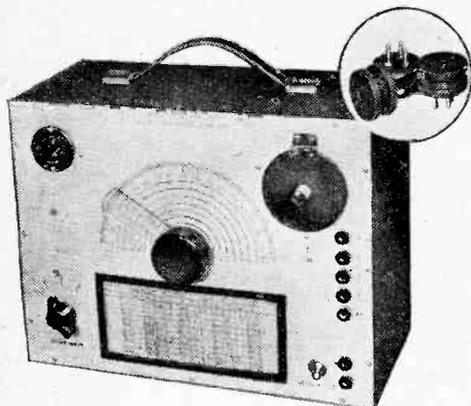
Wearite AC mains operated all-wave test oscillator. Note spare coils shown in inset.
