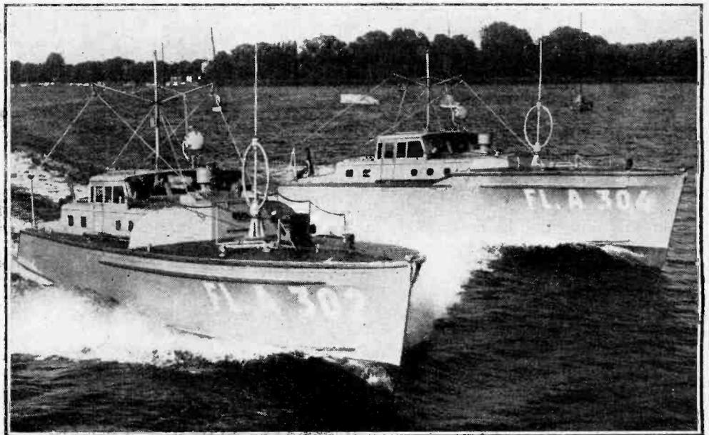
SEAPLANE TENDERS of the German Air Force have recently been fitted with medium- and short-wave transmitters (500-1000 and 50-100 metres) and direction-finding gear for use in locating aircraft in distress at sea. In the above photograph can be seen the DF loop and the transmitting and receiving aerials.
