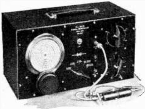
Compact battery-operated all-wave signal generator made by A. H. Hunt.
