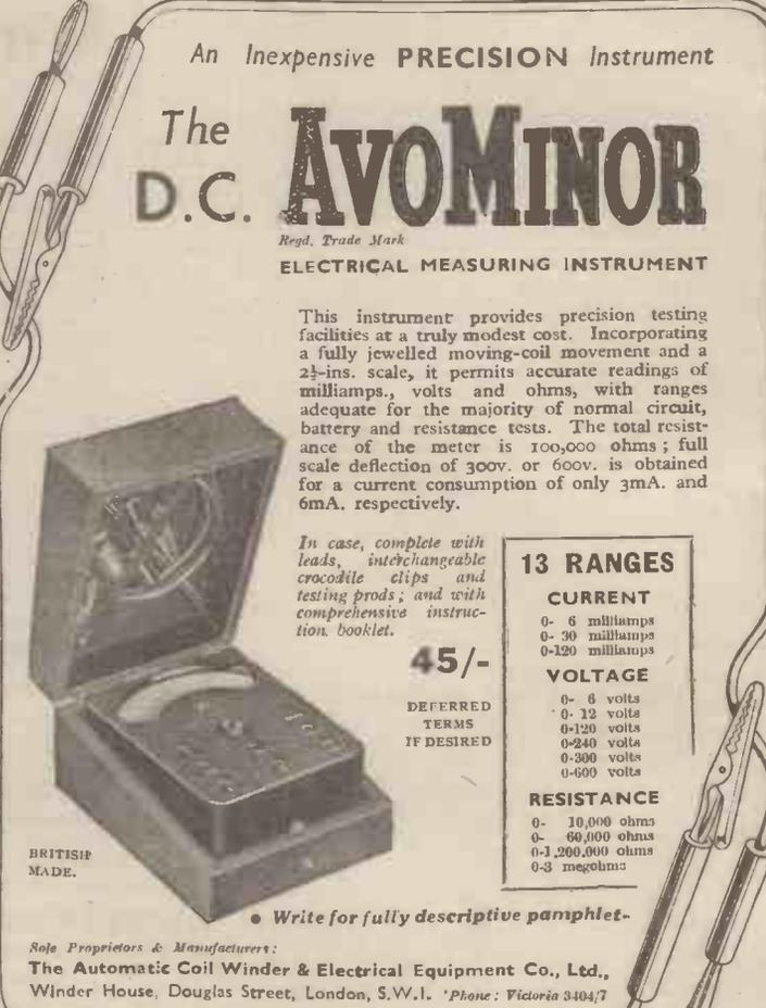
This instrument provides precision testing facilities at a truly modest cost. Incorporating a fully jewelled moving-coil movement and a 2 1/2-ins. scale, it permits accurate readings of milliamps., volts and ohms, with ranges adequate for the majority of normal circuit, battery and resistance tests. The total resistance of the meter is 100,000 ohms; full scale deflection of 300v. or 600v. is obtained for a current consumption of only 3mA. and 6mA. respectively.
