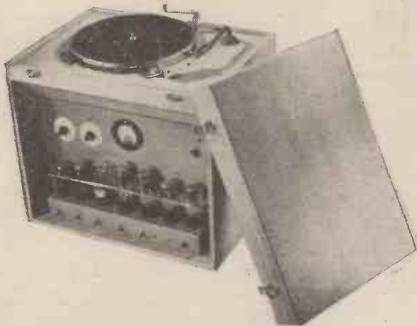
Oak case with lid and carrying handles. Output approximately 20 watts undistorted. Four output impedances provided as standard—24, 12, 6 and 3 ohms. Bass and treble tone controls for pick-up. Press button metering for all stages.
