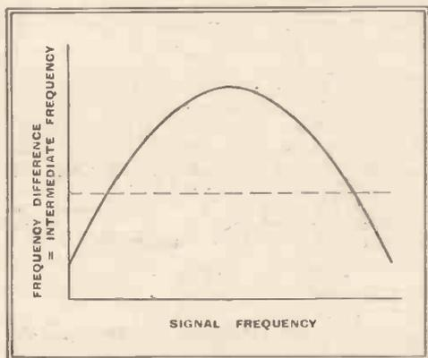
Fig. 11.—This curve illustrates the ganging errors likely when the oscillator is "ganged" only by changing the inductance and either the maximum or minimum capacity of its tuning condensers.
