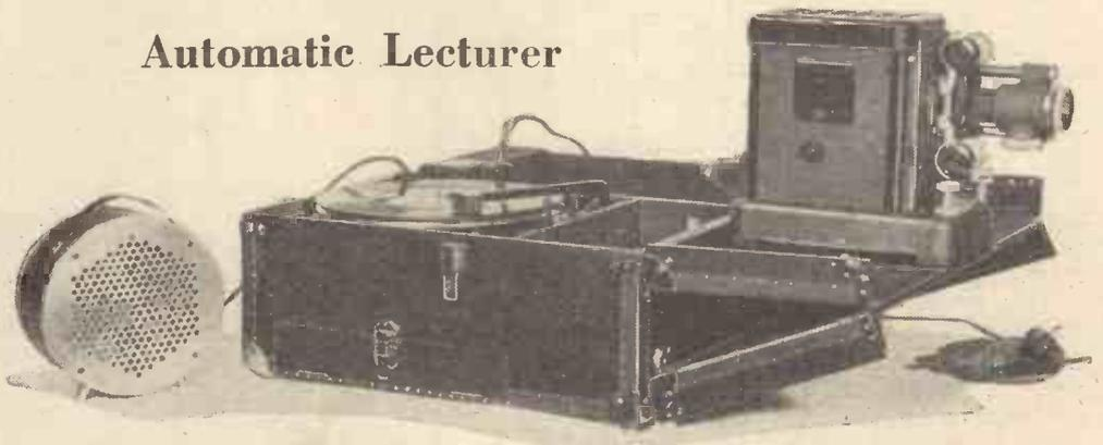
Portable equipment is being demonstrated by the Telefunken Company which enables talks previously recorded on slow-motion 15-minute discs to be amplified and, where necessary, illustrated by means of short films or lantern slides from a projector incorporated in the unit. The necessary breaks in the recording to permit the showing of particular slides can be timed during the recording. It is claimed that a satisfactory "lecture tour" can be carried out by anyone able to operate the gear.
