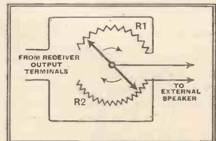
Constant impedance volume control near the "minimum" position. As volume is increased R1 is reduced and R2 increased. The value of R1 should be approximately equal to the loud speaker impedance and R2 about five times the resistance of R1.
