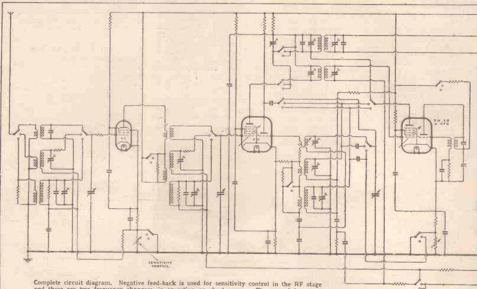
Complete circuit diagram. Negative feed-back is used for sensitivity control in the RF stage and there are two frequency changers in operation on short waves. The second frequency changer becomes the AFC control valve for press-button tuning.
