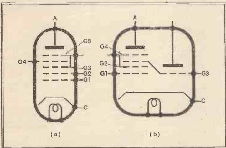
In the heptode G1 is the oscillator grid, G2 the oscillator anode, G3 and G5 are screen grids, which are maintained at a fixed potential, while G4 is the signal grid. In the triode-hexode G1 is the signal grid, G2 and G4 are screen grids, while G3 is the oscillator grid. Both valves, of course, may have an extra electrode outside the outer screen to reduce the effects of secondary emission; they then become octodes and triode-heptodes respectively.
