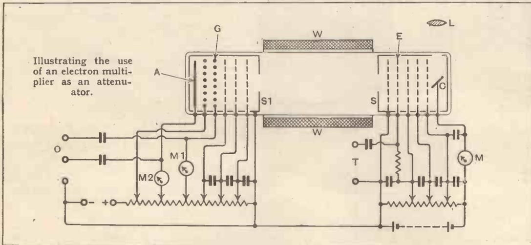
Illustrating the use of an electron multiplier as an attenuator.
