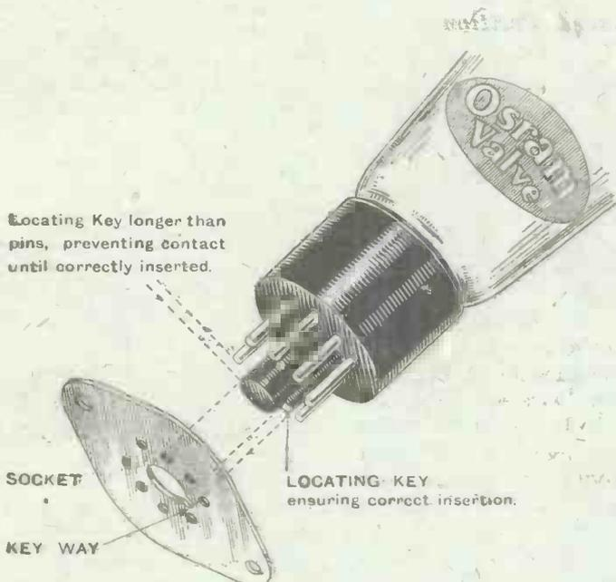
The utility of the valves with the self locating octal base is becoming firmly established, and designers and others will appreciate the introduction of new types having characteristic advantages hitherto not obtainable in this range.
