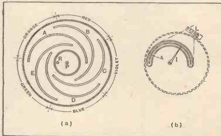
Tuning dial in which the various wavebands are indicated by different colours.
