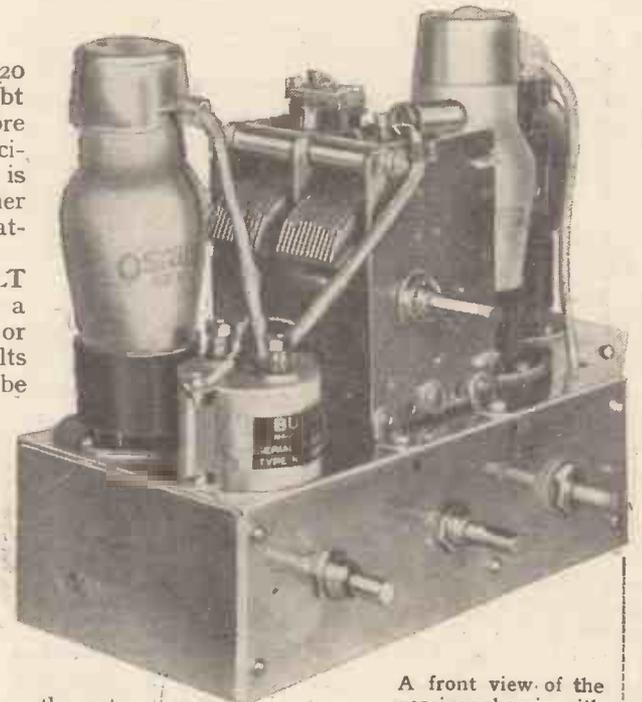
A front view of the receiver chassis with the RF valve in the foreground.
