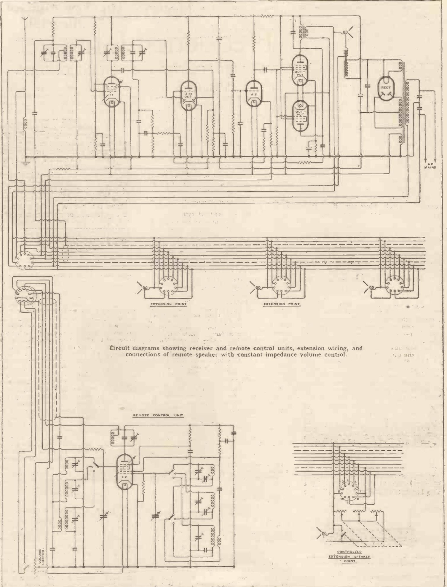
Circuit diagrams showing receiver and remote control units, extension wiring, and connections of remote speaker with constant impedance volume control.
