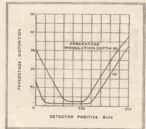
Fig. 4.—The effect of positive bias on distortion is shown here for two modulation depths. The signal input is again 40 volts and R<sub>2</sub> is 50,000 ohms.
