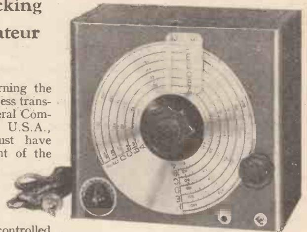
The meter is direct-reading, with separate scales for each of the bands covered.
