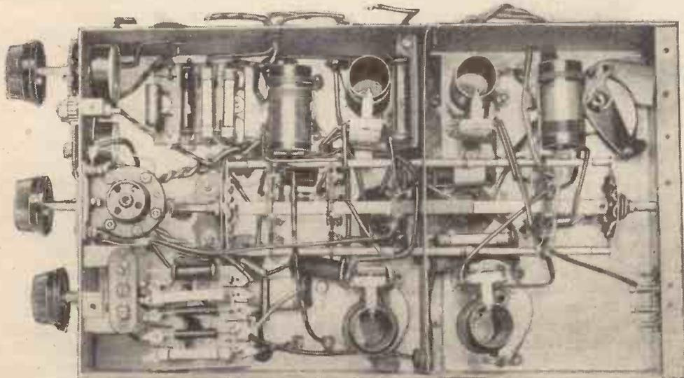
Underside of the pre-tuned unit; note the two panels carrying, respectively, the diode and the phase-changer components; also the small panel mounting for the 200-ohm resistor in the cathode of the RF pentode, and that for the voltage dropping resistance fitted near the dividing screen. The 8-mfd. condenser for detector decoupling is under the AF output terminal strip at the front of the chassis.
