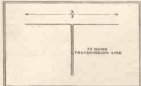
Fig. 25.—The centre of a half-wave aerial is the correct point of connection for a 72-ohm transmission line.
