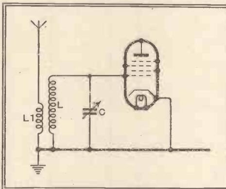
Fig. 4. The usual aerial coupling and tuning system are shown here.
