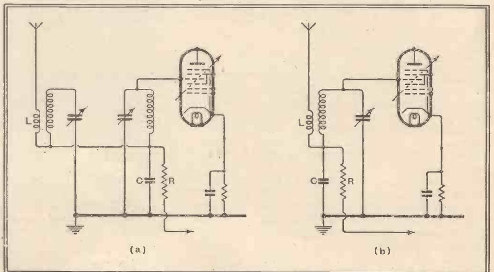
Fig. 3.—Receiver input circuits with which the multivibrator does not work satisfactorily unless AF and IF filters are included.
