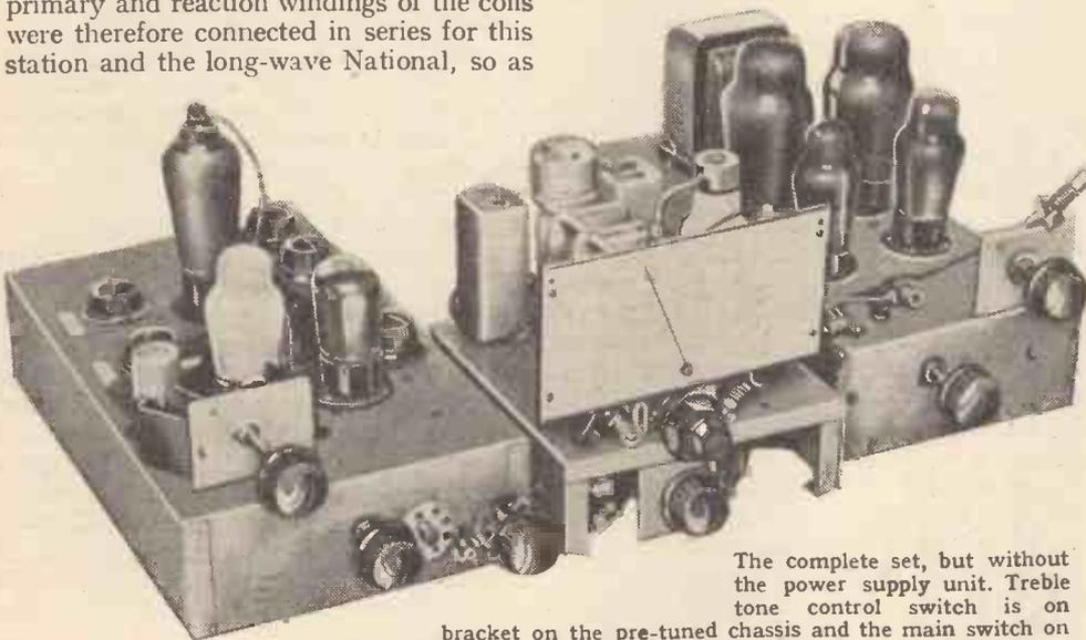
The complete set, but without the power supply unit. Treble tone control switch is on bracket on the pre-tuned chassis and the main switch on the corresponding bracket at the right. The gears which gang the two volume controls are clearly shown.
