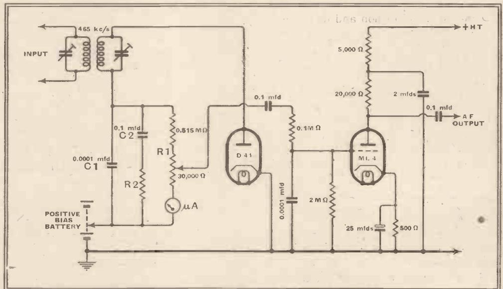
Fig. 2.—The circuit is shown here of the apparatus upon which the measurements were taken. The shunting effect of the AC load is provided by R<sub>2</sub>.
