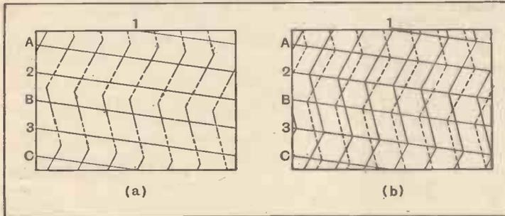
The normal interlacing system (a) compared with a method (b) in which the width of both sets of lines is doubled.
