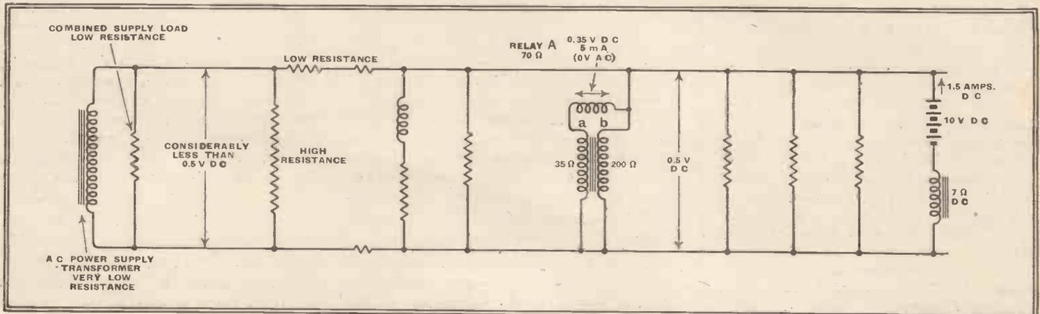
Fig. 2.—The equivalent electrical circuit in simplified form.
