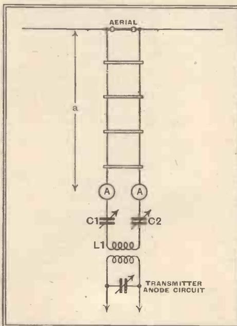
Fig. 27.—If the tuned feeders are an even number of quarter-waves long, a half-wave aerial should be arranged in this way.
