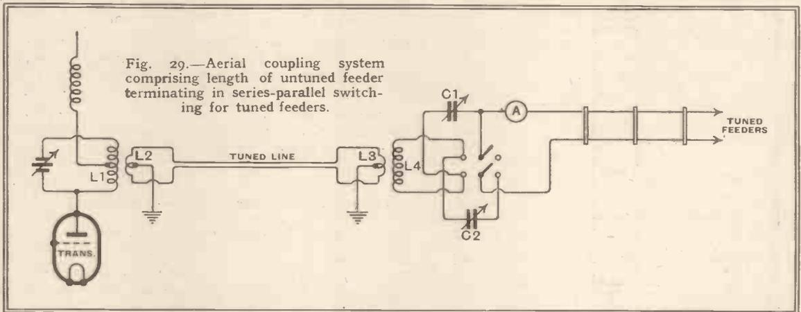
Fig. 29.—Aerial coupling system comprising length of untuned feeder terminating in series-parallel switching for tuned feeders.
