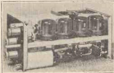
GERMAN CAR-RADIO. The new all-metal valves have been used extensively in the new car-radio receivers which were to be seen at the Berlin Motor Show. There is no waste space in the 6-valve Körting receiver, shown here.
