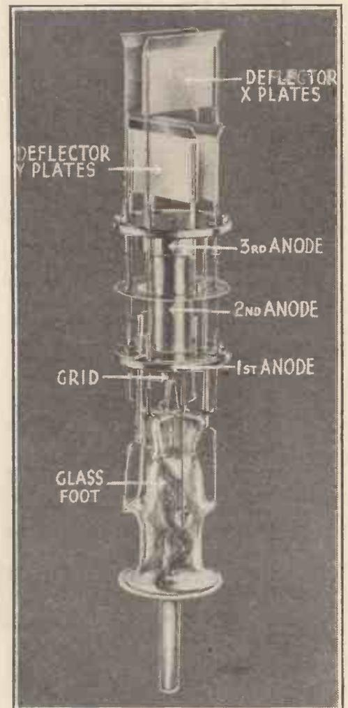
Fig. 14. Internal view of the Cossor three-anode tube.
