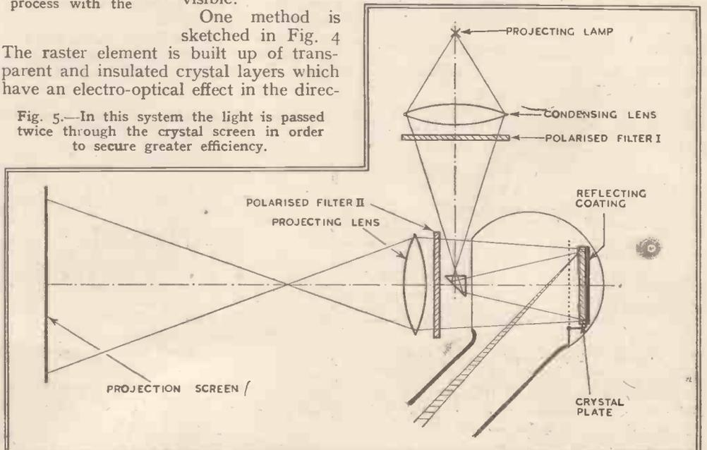
Fig. 5.—In this system the light is passed twice through the crystal screen in order to secure greater efficiency.
