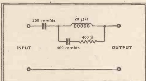
Fig. 4.—Standard all-wave dummy aerial.
