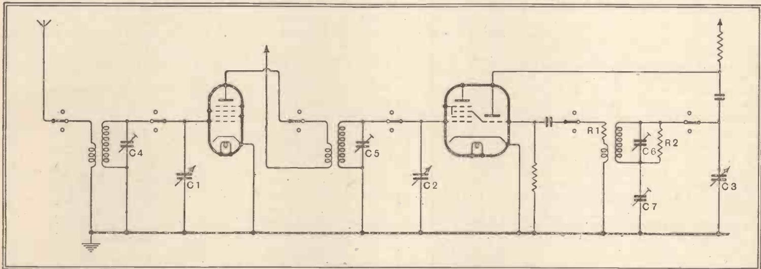
Fig. 14.—The circuit of the receiver including the frequency changer and showing the switching and the ganging arrangements.
