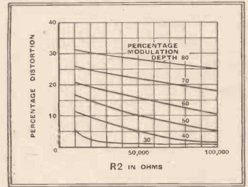
Fig. 3.—These curves show the effect on distortion of varying R<sub>2</sub> for various modulation depths. The signal input is 40 volts peak.
