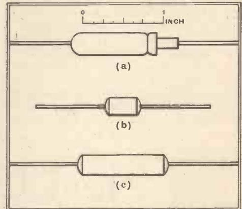
Fig. 2.—Sketch showing external appearance and sizes of Sprague (a) and Erie (b and c) compensating condensers.
