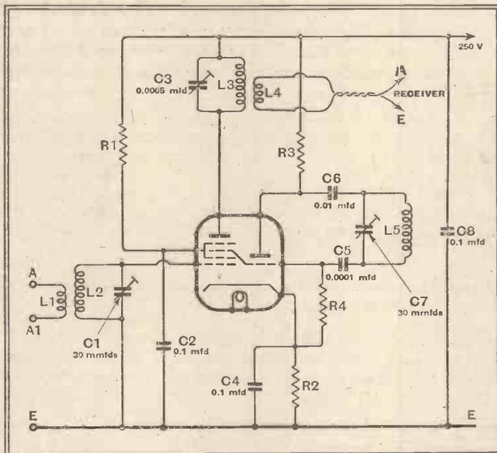
ling coil for taking the IF output to the input of the broadcast set.
