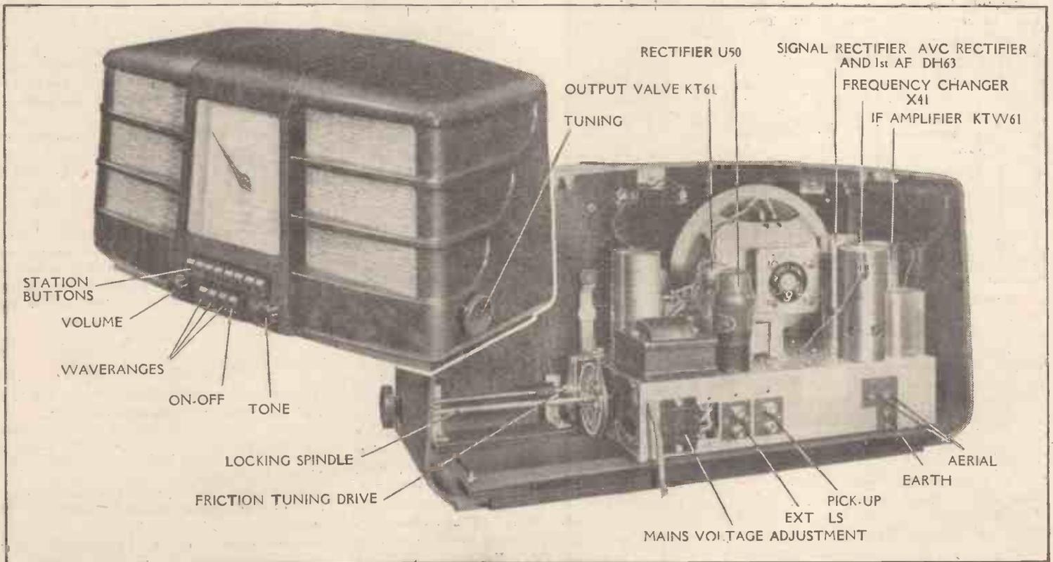
Arrangement of controls and layout of valves and terminal panels in the G.E.C. Model 4050.
