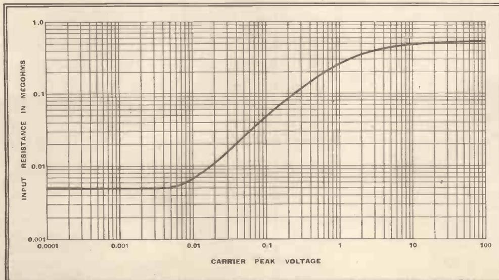
Fig. 8.—This curve illustrates the variation of input resistance with signal input voltage for 1 volt positive bias on the diode and R1 equal to 1MΩ. The diode AC resistance is 5,000 ohms.
