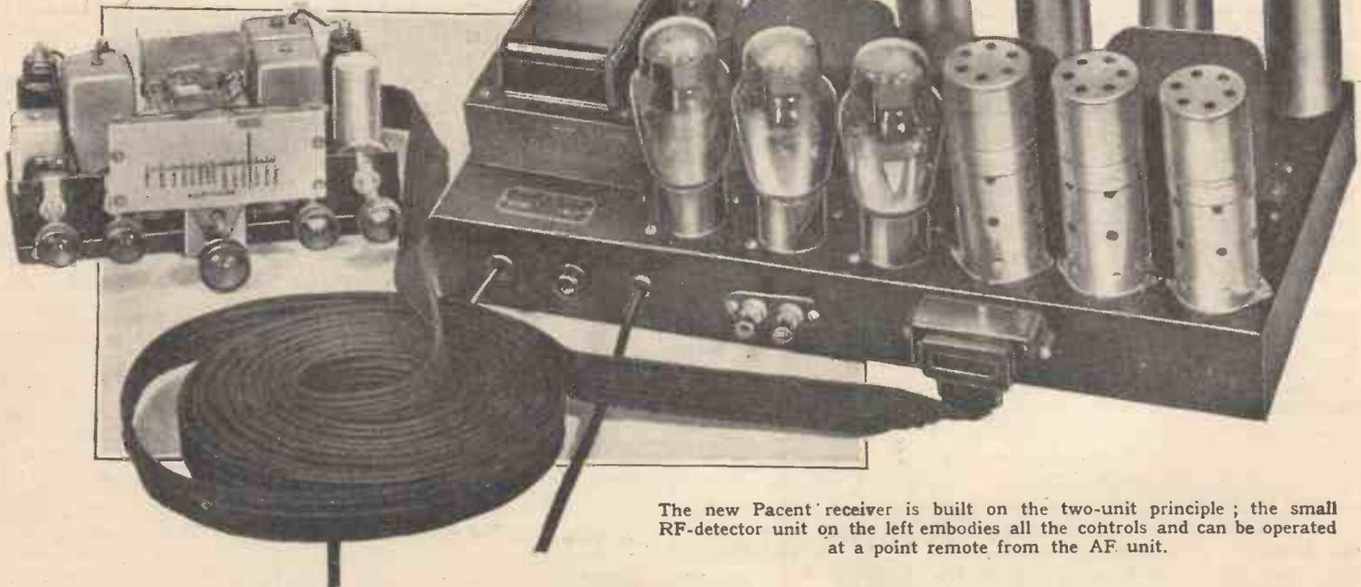
The new Pacent receiver is built on the two-unit principle; the small RF-detector unit on the left embodies all the controls and can be operated at a point remote from the AF unit.
