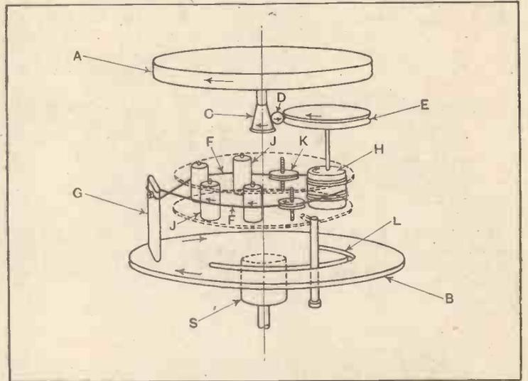
Schematic diagram of two-speed variable condenser drive mechanism.
