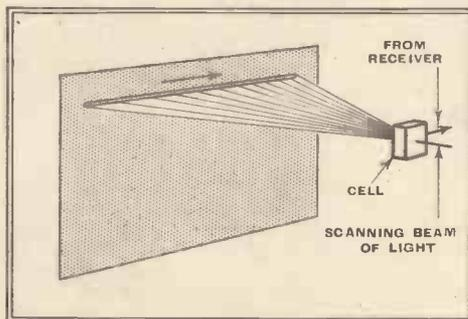
Fig. 3.—In the Scophony system not only is the spot corresponding to the transmitter scan position illuminated, but also a whole strip of the screen in its train. The cell has to store or "remember" the signals just past so as to keep the right distribution of light over the whole strip.
