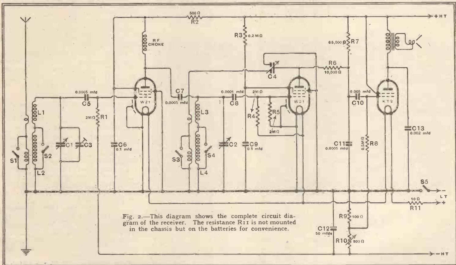
Fig. 2.—This diagram shows the complete circuit diagram of the receiver. The resistance R11 is not mounted in the chassis but on the batteries for convenience.
