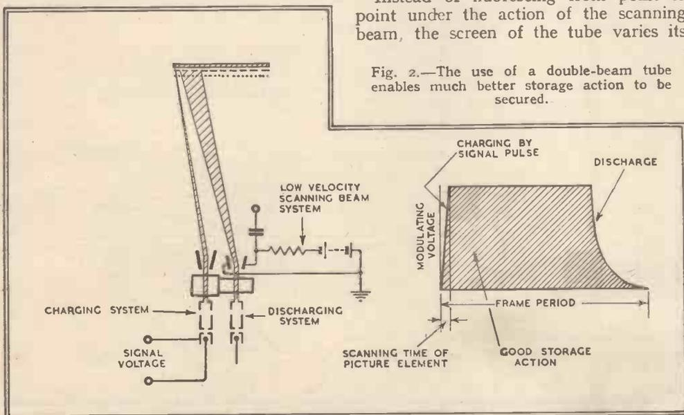
Fig. 2.—The use of a double-beam tube enables much better storage action to be secured.
