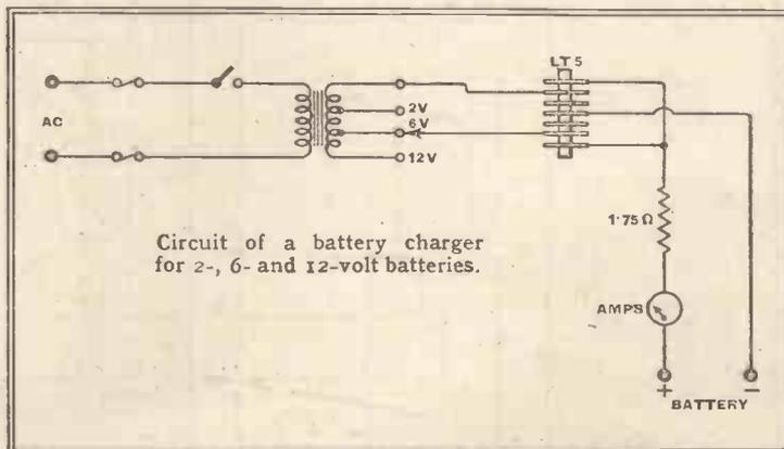
Circuit of a battery charger for 2-, 6- and 12-volt batteries.
