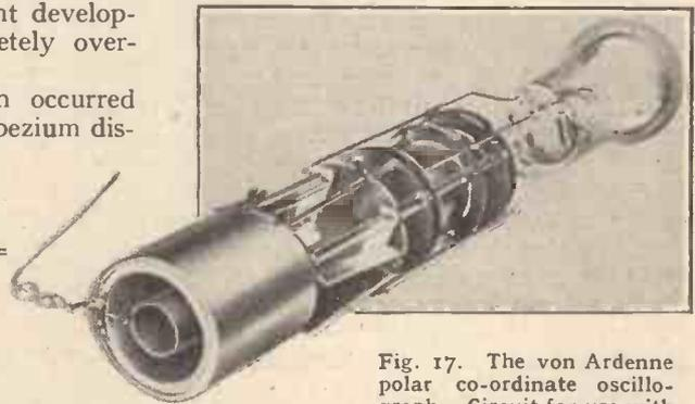
Fig. 17. The von Ardenne polar co-ordinate oscillograph. Circuit for use with the polar co-ordinate oscillograph (a). Variation of circle diameter due to application of potential to be examined is seen to the right of the circuit (b).
