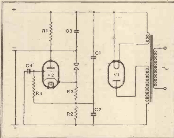
Ripple neutralisation by means of a smoothing valve. Values of components used were: C<sub>1</sub>, 0.01 mfd. ± 5%; C<sub>2</sub>, 0.8 mfd. ± 5%; C<sub>3</sub>, omitted (see text); C<sub>4</sub>, 0.25 mfd. ± 20%; R<sub>1</sub>, 5 megohms ± 20%; R<sub>2</sub>, 0.2 megohm ± 5%; R<sub>3</sub>, 3,000 ohms ± 20%; R<sub>4</sub>, 5 megohms ± 20%.
