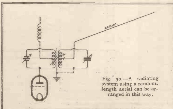
Fig. 30.—A radiating system using a random-length aerial can be arranged in this way.
