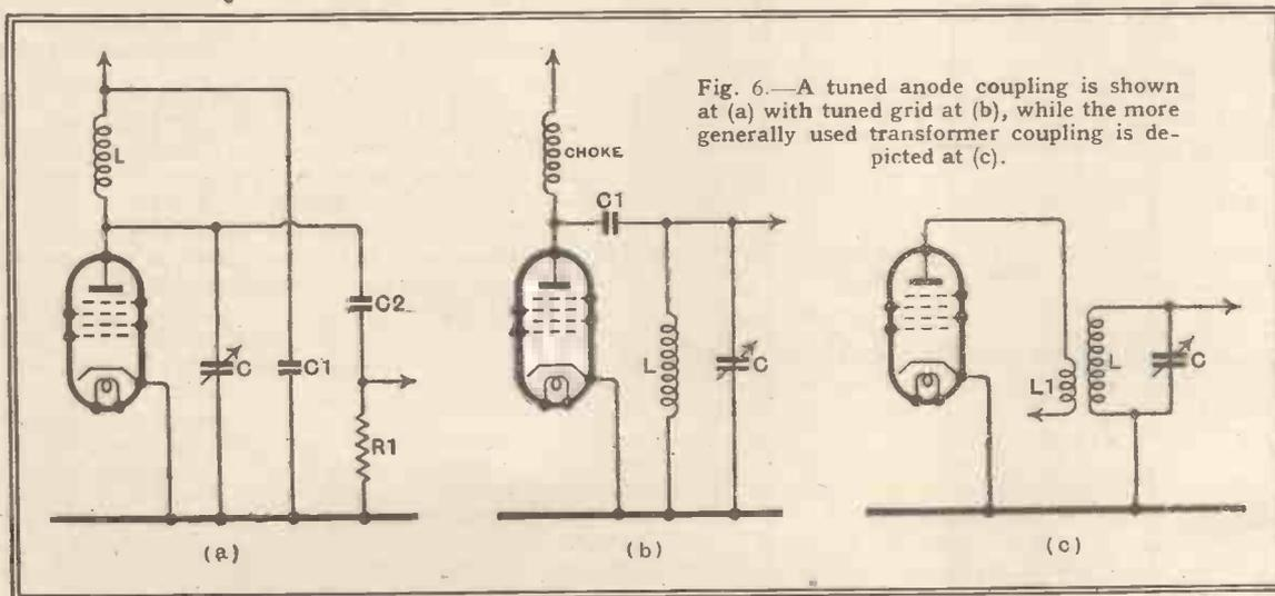
Fig. 6.—A tuned anode coupling is shown at (a) with tuned grid at (b), while the more generally used transformer coupling is depicted at (c).
