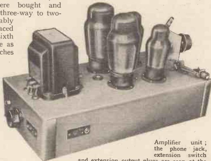
Amplifier unit; the phone jack, extension switch and extension output plugs are seen at the rear and the connections for the set speaker at the side.
