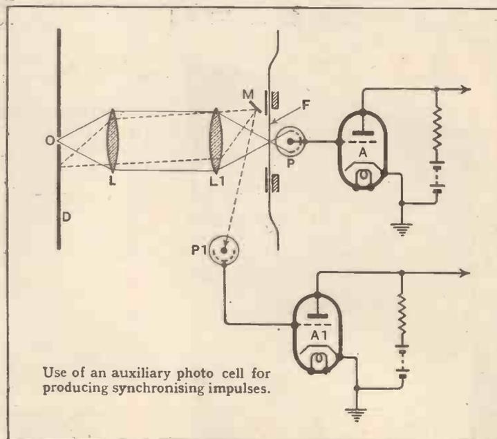
Use of an auxiliary photo cell for producing synchronising impulses.
