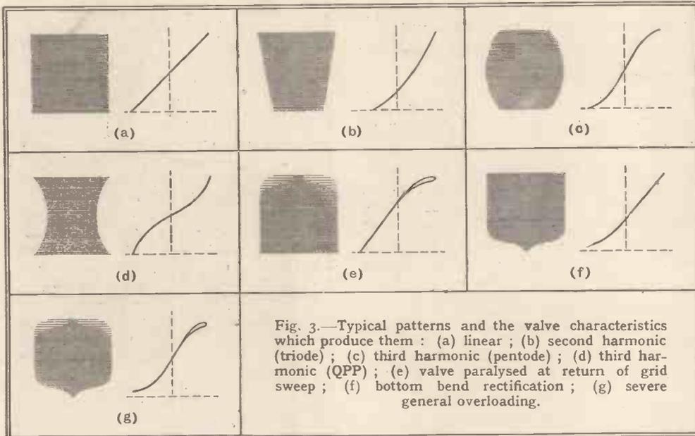
Fig. 3 will give a working idea of the effects produced by different curves. Weird and wonderful are some of the patterns produced by gross overloading, and a lot may be learnt about effects which may never have been expected. One point worth noting is that if one both listens to the sound and looks at the picture, then in every case it will be found that the picture indicates distortion long before it can be detected by ear.
