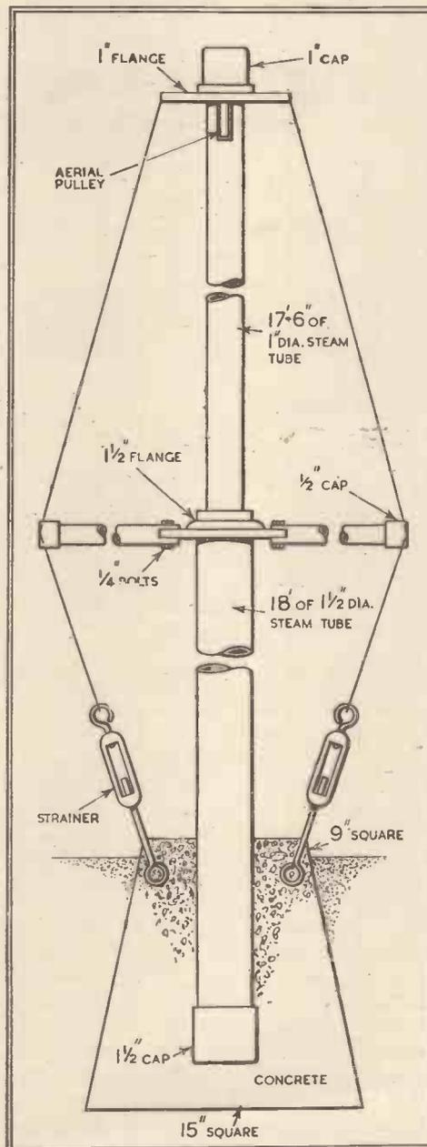
A compromise between the unsupported and the fully-stayed mast can be made by stretching stays of 7/20 SWG galvanized steel wire from the top of the mast to the base, passing en route through a slot cut in the outer end of spreaders attached radially to the centre of the mast. Three spreaders and stays, spaced at an angle of 120 degrees to each other, are used.
