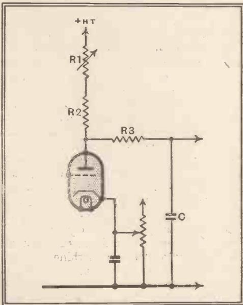
Fig. 1.—The conventional gas-triode saw-tooth oscillator.
