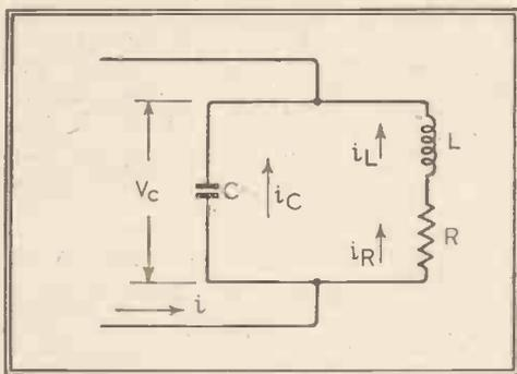
Fig. 1.—This diagram shows the basic circuit of the deflecting coil; R represents the coil resistance and C the circuit capacity.
