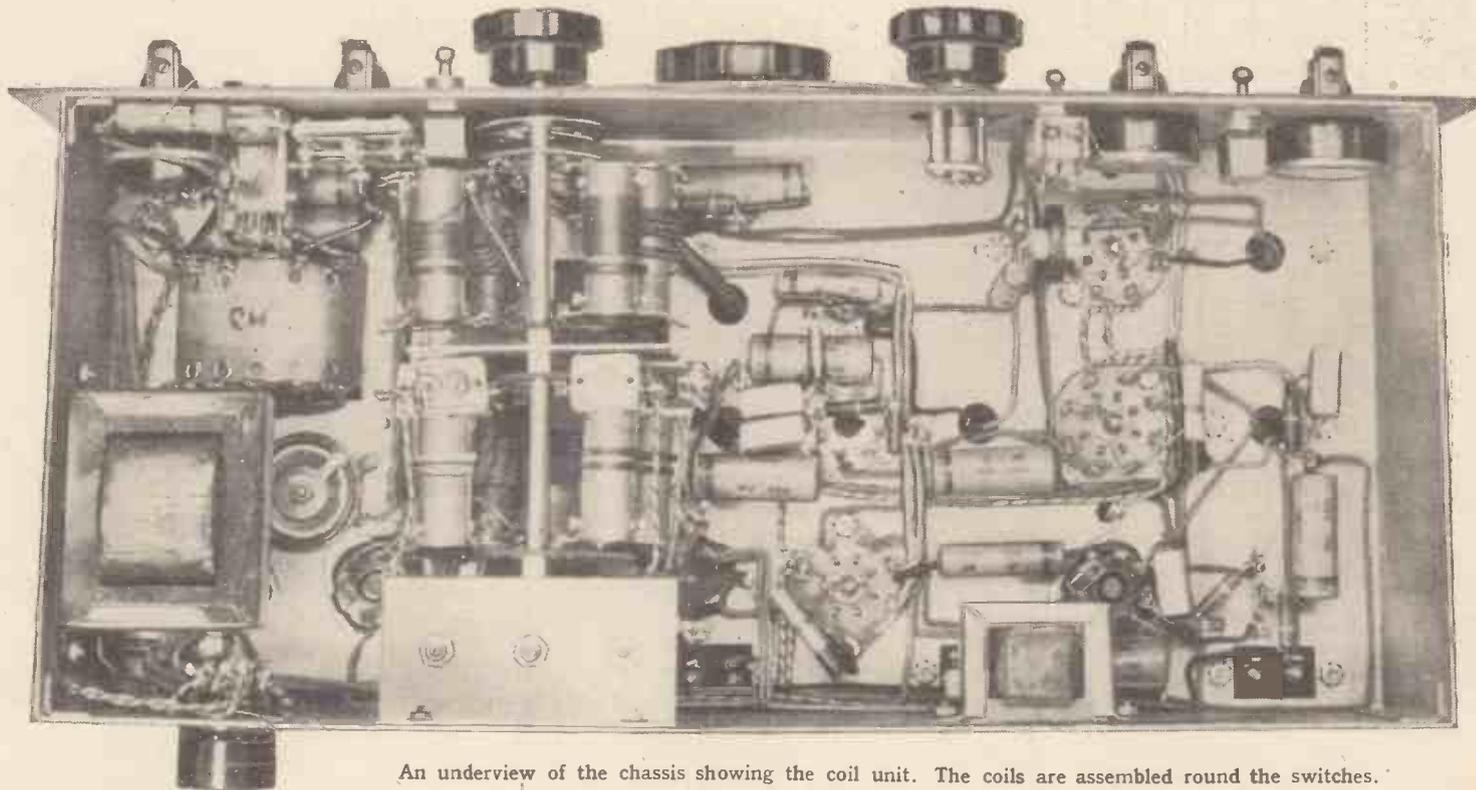
An underview of the chassis showing the coil unit. The coils are assembled round the switches.
