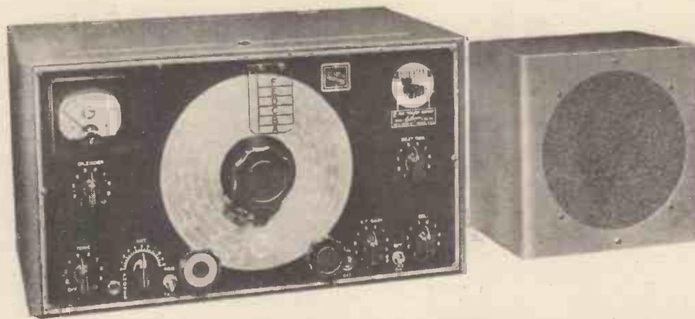
*IN this article there appears a description of an American communication receiver which is especially interesting in view of the use which is made of regeneration. It is obtained at signal-frequency and also at intermediate frequency, and as a result very high sensitivity and selectivity are obtained with a simple circuit*
