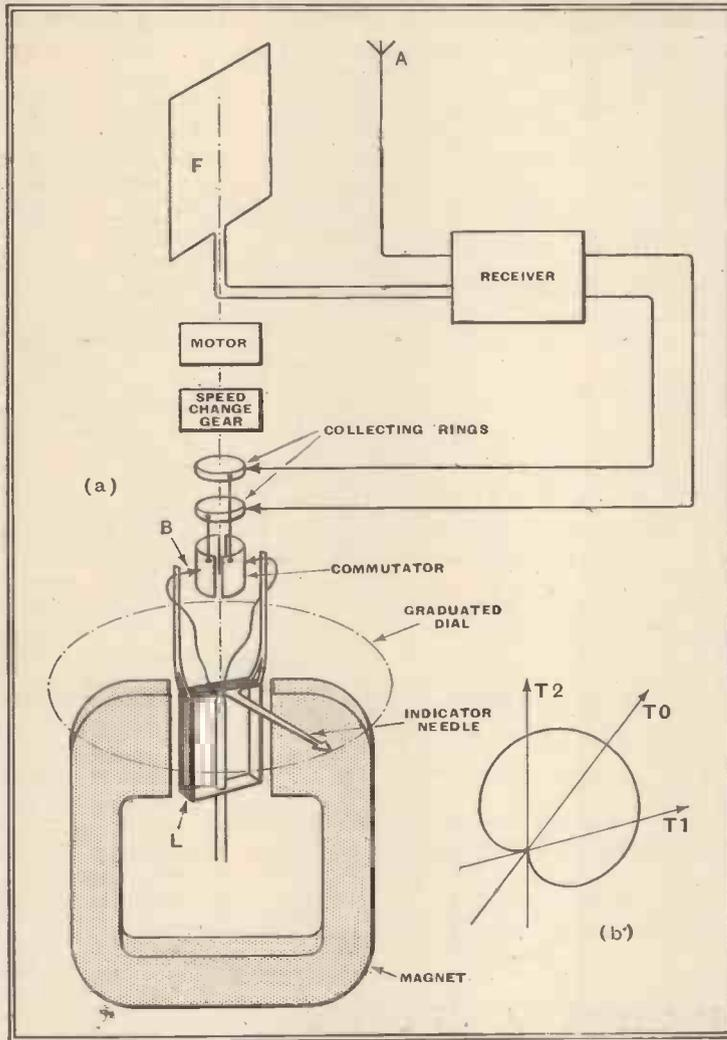
usual 180 deg. ambiguity of the single frame. The indicator is operated by reversing the pick-up current each time the aerial passes through the fore-and-aft line of the machine and balancing the currents collected on one side of the reversing switch against those collected on the other side.
