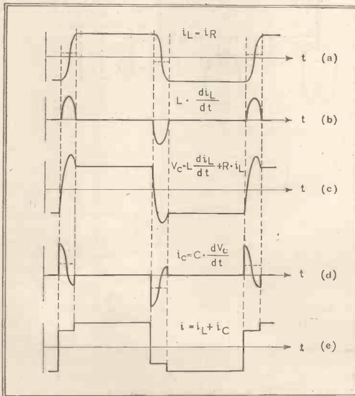
tial curve can be obtained by another differentiation (Fig. 2(d)). It is to be observed that in (c) the negative maximum value of the condenser potential is not reached at  $t_3$ , but only a little later. Accordingly, in (d) the current value zero is passed after  $t_3$ . The curve of the condenser current  $i_c$  is exactly equal, but in a reflected sense, to the first postulated coil current, which is
