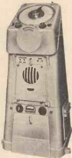
The direction finder which is mounted on the bridge enables the true bearing to be read. A second scale on the instrument is coupled to the gyroscopic compass so that true great circle bearings may be directly observed.
