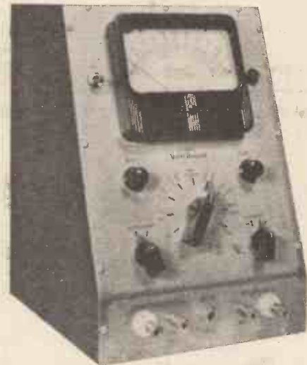
The Rider "VoltOhmyst" may be used for the measurement of all receiver voltages including AVC without introducing any appreciable load on the circuit.
