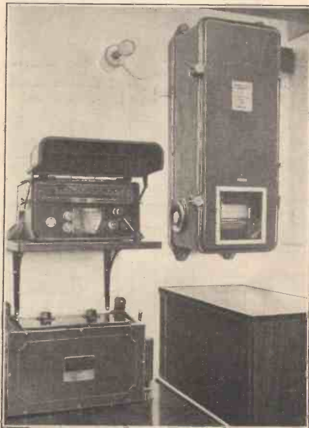
The echometer sounding device makes use of supersonic pressure waves through the water to plot a contour of the sea bed.
