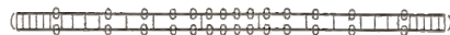
Fig. 2.—The same applies to a close-spaced parallel line, although this is a tuned circuit with inductance and capacity distributed over a long distance. The rings indicate lines of magnetic force around the wires, and the short lines represent the electric force between them.
