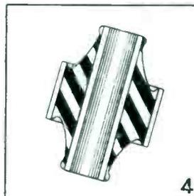
4. The double hyperbolic rubber contour gives even distribution and allows for central application of radial load. Stress-reducing pips prevent stress concentration.
