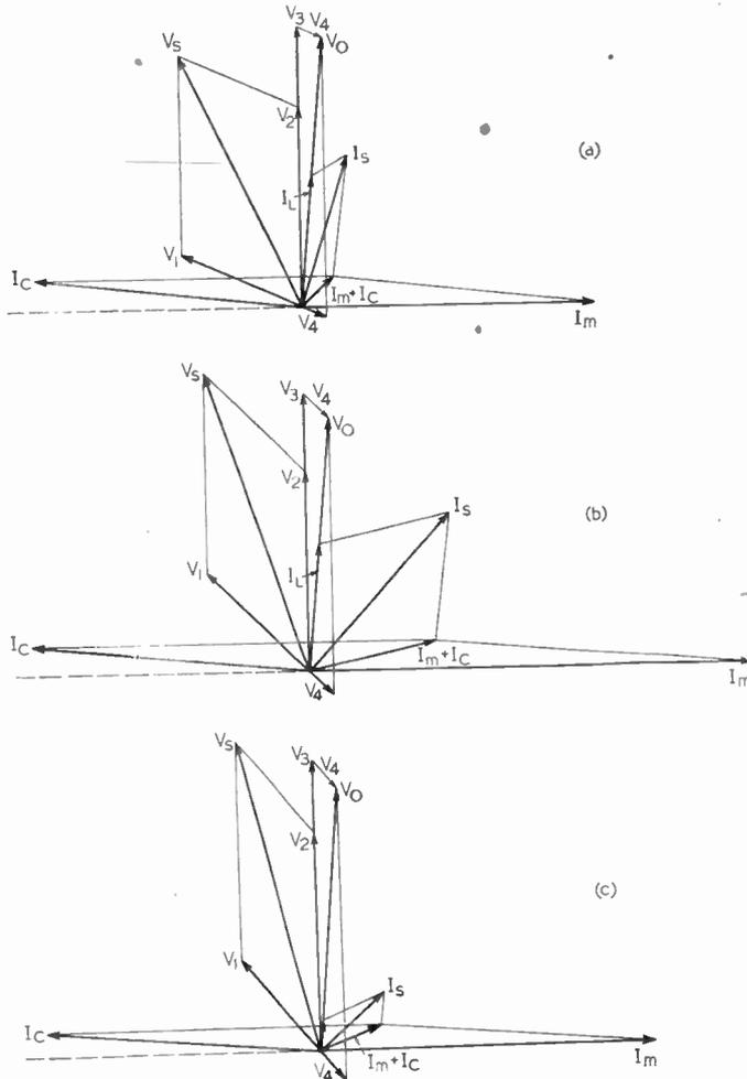
Fig. 3. Vector diagrams of action of "Stabilistor": (a) supply voltage low, load maximum; (b) supply voltage high, load maximum; (c) supply voltage high, no load. The effect of choke L at 50 c/s is assumed to be negligible.
