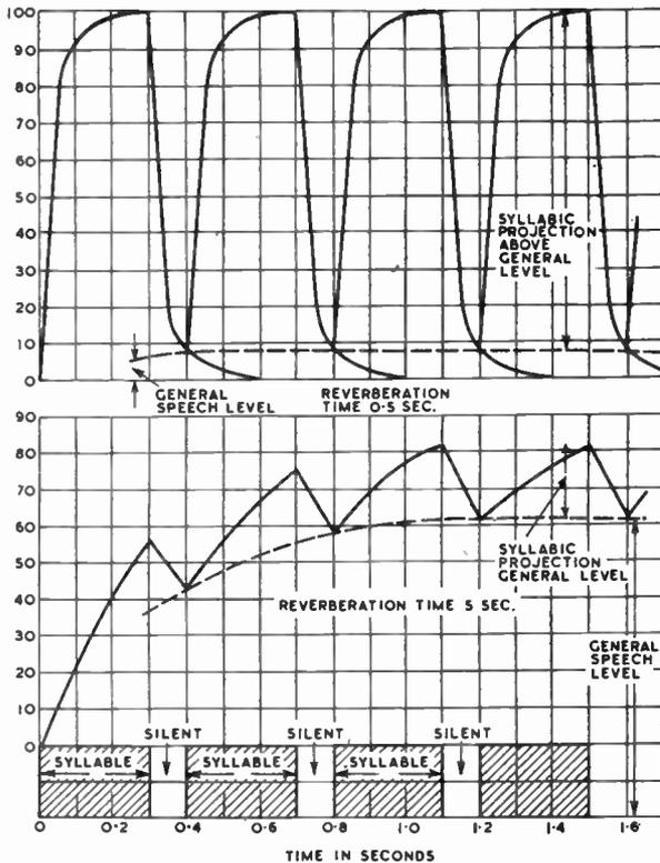
Fig. 2. Growth and decay of sound pulses of average syllabic length in rooms with different reverberation times.
