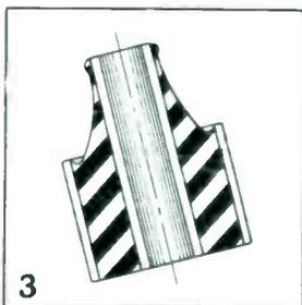
3. This hyperbolic rubber contour gives partially even stress distribution with stress reducing pips at metal edges, the stress concentration is at the flat edges and there is unbalanced application of radial load.
