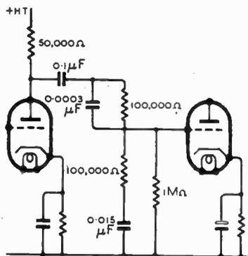
Fig. 5. Bass and treble boost circuit which generally improves the response of a receiver or amplifier.
