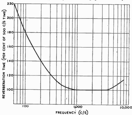
of reverberation time, Figs. 3 and 5 give the reverberation-time/frequency curve of Fig. 6 as being the optimum for reproduced music.
