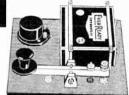
No. 1261. Complete Morse Practice Unit. Heavy commercial Key with nickel silver contacts and sensitive triple adjustment. High-tone Buzzer with silver contacts, mounted on bakelite base with cover. Battery Holder, complete with 4.5 Ever Ready battery. All metal parts heavily nickel plated, and the whole mtd. on polished Mahogany Base, 6 1/2 in. x 6 1/2 in. Price **29/6**
