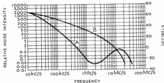
Variation of radio noise with frequency at noon (A) and at midnight (B) in the Northern temperate zone. From curves given by R. K. Potter, *Proc. I.R.E.*, Sept. 1932.
