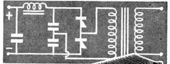
A metal rectifier in the voltage doubler circuit provides full wave rectification with a transformer secondary voltage less than the voltage of the output from the rectifier. Further, no filament winding is required and the transformer is simpler and less costly.
