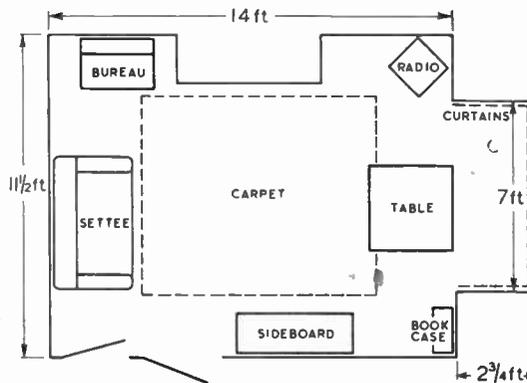
Fig. 1. Plan of small living room used for acoustic investigations.
