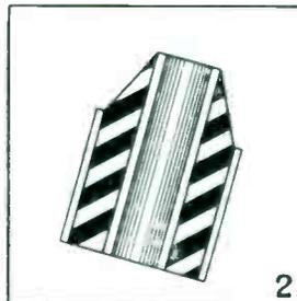
2. This gives flat rubber contour with high stress concentration at edges of rubber-metal bond. It gives equal stress at bonded surfaces but unequal stress in rubber volume and also unbalanced application of radial load.
