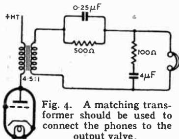
Fig. 4. A matching transformer should be used to connect the phones to the output valve.
