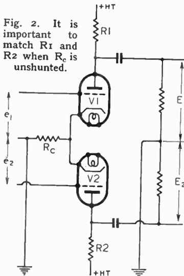
This is because the currents are dependent not only on  $R_1$  and  $R_2$ , but also on the valve resistances, so that the ratio of the currents is smaller than  $R_2/R_1$ .
