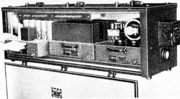
A single-channel train communication equipment comprising transmitter, receiver and power supply units. Interconnection is by means of plugs and sockets giving easy replacement of a faulty unit. The container has shock-absorbing mountings.
