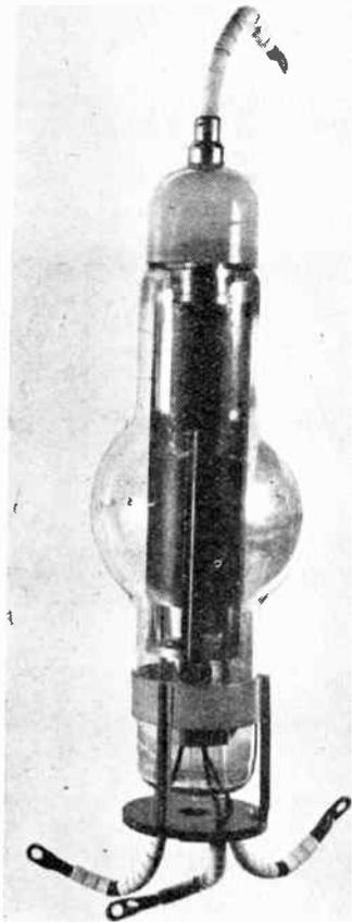
High-voltage thyatron developed by B.T.H. for use in pulse modulation.
