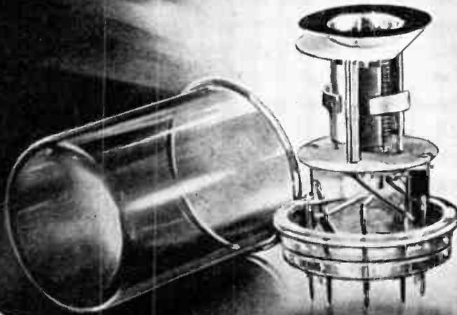
By a complete departure from the conventional form of valve construction, Mullard have effectively reduced the losses due to H.F. resistance, inductance and capacity effects within the valve itself and in the leads coming from the electrodes.
