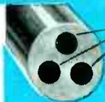
**3 CORES OF FLUX** provide just the correct proportion of flux to solder. NO extra flux is required. The flux does not tend to run out of the cores: so there is always a supply available for the next joint. The utmost economy of flux and solder is achieved.
