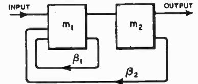
Fig. 8. Block diagram of amplifier of Fig. 7.
