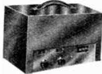
Output—two 6V6's in P.P. with cathode coupled phase changing using 6J5's. First stage 6J5, rectifier 5Z4.
