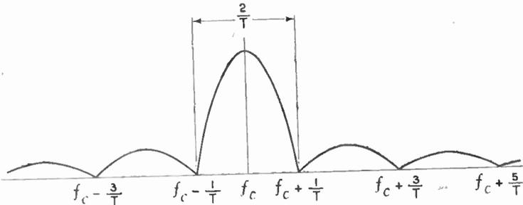
Fig 4. Sideband structure of rectangular pulse of length T.
