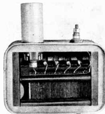
Delay-network unit for airborne H2S and ASV radar, designed to withstand high pulse loadings (case cut away). Developed and made by Dubilier.
