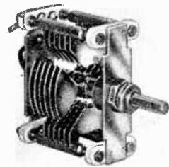
Split-stator condenser for radar developed by Eddystone. Maximum capacity (parallel-connected) 200  $\mu\mu\text{F}$ : flash - over 700 V.
