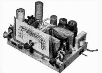
Parts, new, ex-televison, aluminium screened coils, excellent short-wave reception (the special coils used in this circuit give a performance equal to a superhet.), 4 1/2 watts output, complete with loudspeaker, all parts, wiring and theoretical diagram—nothing extra to purchase. Chassis dim.: 12in. x 8in. x 6in. to top of dial 200/250 v. A.C. Including tax .. 11½ Gns. Case and packing, 5/- extra.
