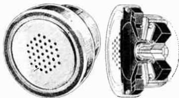
Originally manufactured as Moving Coil Headphones, these can be successfully used as Midget Loudspeakers (with a suitable transformer) as Speech Microphones or can be adapted for Pick-ups. A powerful Alni Permanent Magnet energises the 1/4 in. coil. In sealed metal case. 1 1/4 in. diameter as illustrated. 8/9 each, post free.
