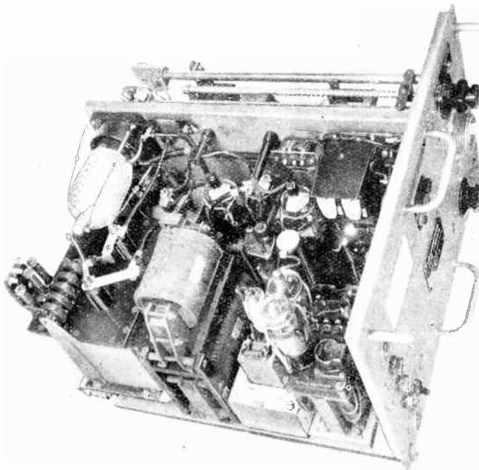
A Metro-Vick radar transmitter of the intermediate period, giving high pulse power with small valves.
