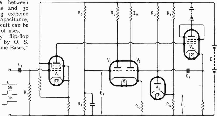
Fig. 3. Improved flip-flop circuit. Typical values:— $R_1 = 100k\Omega$ ,  $R_2 = 100k\Omega - 3M\Omega$ ,  $R_3 = 6.8k\Omega$ ,  $R_4 = 8.2k\Omega$ ,  $R_5 = 4k\Omega$ ,  $C_1 = 100pF$ ,  $C_2$  according to required  $t_0$ ,  $E_1 = 40V$ ,  $E_2 = 55V$ ,  $E = 250V$  volts,  $V_1 V_2 =$  ECC32 or 6N7,  $V_4 = V_3 =$  EF50,  $V_5 =$  EA50. N.B. For  $t_0 < 10\mu sec$  miniature valves would be desirable.
