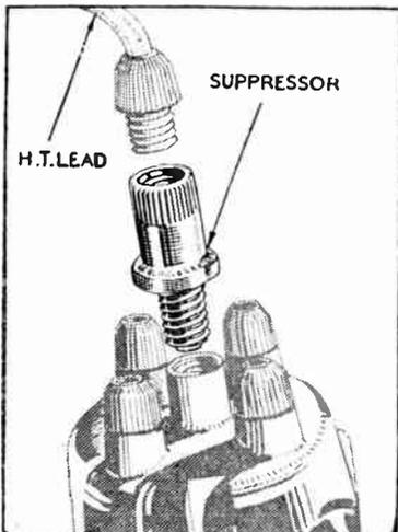
\*1 The sketch shows the simple method of fixing the "Belling-Lee" distribution lead suppressor L630 which sells at 1/6 each.
