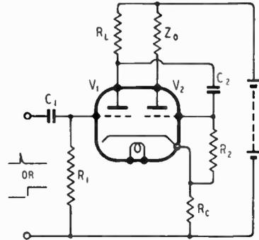
Fig. 2. Simple time delay flip-flop. Typical values:— $R_1 = 100k\Omega$ ,  $R_2 = 1M\Omega$ ,  $R_L = 100k\Omega$ ,  $R_c = 1000\Omega$ ,  $Z_0 =$  required load,  $C_1 = 100pF$ ,  $C_2$  according to required  $t_0$ ,  $E = 200$  volts,  $V_1 V_2 =$  ECC32 or 6N7.
