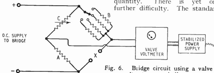
Fig. 6. Bridge circuit using a valve voltmeter as an indicator.
