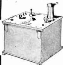
Oil Filled Transformer. 4 kVA. Input 230 volts, 50 cycles, output 18,000 volts. Contents approx. 56 lbs. copper, 112 lbs. laminations, 13 galls. transformer oil.
