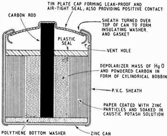
Fig. 1. Constructional details of the Vidor "Kalium" cell.
