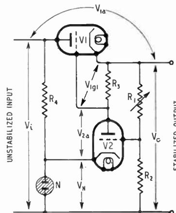
Fig. 1. Basic circuit of series-valve stabilizer, in which the output voltage  $V_0$  is adjusted by varying  $R_1$ . N is the voltage reference standard, and  $V_2$  the negative feedback amplifier.
