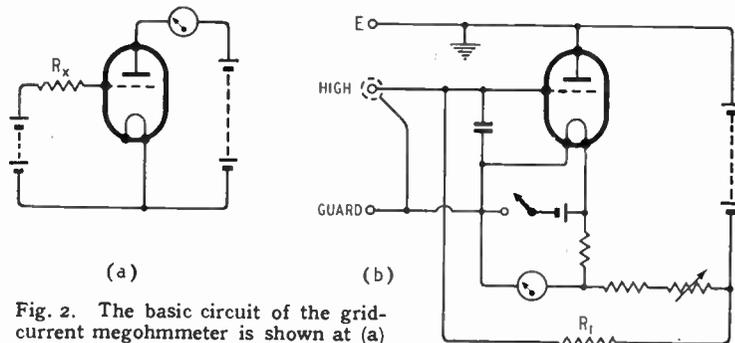
Fig. 2. The basic circuit of the grid-current megohmmeter is shown at (a) and its practical form at (b).
