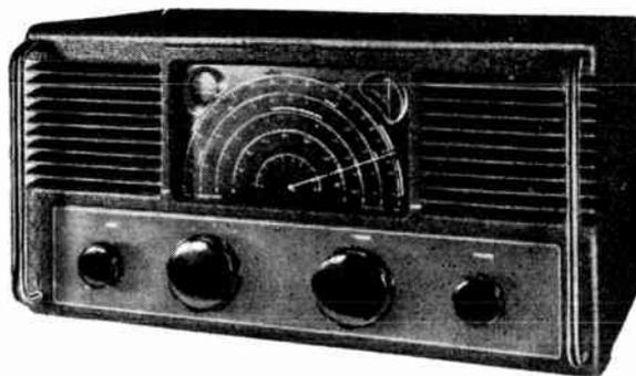
This view of the Eddystone 670 shows the large calibrated dial and the disposition of the controls. The bandspread dial is in the top right-hand corner of the main dial.
