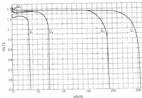
**Fig. 3. Discharge continuously through 25Ω (hearing aid conditions) of U1, U2, U4 and U6 sizes.**
