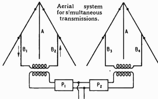
central mast A in each pair B<sub>1</sub>, B<sub>2</sub> and B<sub>3</sub>, B<sub>4</sub> of the outer aerials will be in phase, and will therefore cancel at the terminals of the second transmitter. The symmetry of the arrangement preserves the normal radiation pattern of both the aerials.
