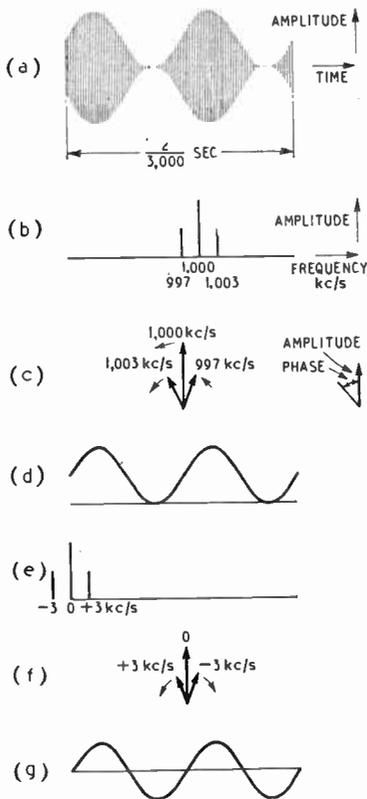
Fig. 3. A high frequency (1000-kc/s) carrier wave modulated at 3 kc/s, represented in three ways—*a*, *b*, and *c*. A zero-frequency "carrier wave" modulated at the same frequency is shown in the same ways at *d*, *e* and *f*. *g* is an alternative to *d*, representing a different "phase" of the "carrier wave."
