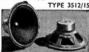
Overall diam. 12½". Depth 6". Weight 7lb. 15 ozs. Voice Coil Impedance 15 ohms. Fundamental resonance 60 cycles. Flux density 14,000 lines per. sq. cm. Frequency range 50-7,000 c.p.s. Fixing holes 4 holes ½" diam. spaced 90° on P.C.D. 12½".
