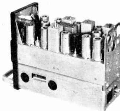
Chassis assembly of the G.E.C. BRT600 V.H.F. set. The power unit is in the base.
