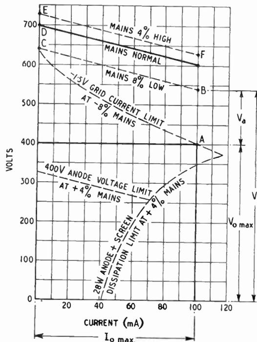
Fig. 2. Voltage/current design diagram for a series-valve stabilizer.
