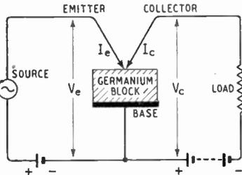
Fig. 1. Basic circuit of the Transistor.
