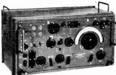
**R107. ONE OF THE ARMY'S FINEST COMMUNICATIONS RECEIVERS.** (See "W.W.," August, 1945.) 9 valves, R.F. amp. osc. Frequency Changer, 2 I.F.'s (465 kc.), 2nd Detector, AVC. Af. amp. B.F.O. A.C. mains, 100-250 v. or 12 v. accum. Frequency range 17.5 to 7 mc/s, 7.25 mc/s to 2.9 mc/s, 3.9 to 1.2 mc/s. Monitor I.S. built-in. Complete. Write for full details. **£18 18 0.** Carriage paid.
