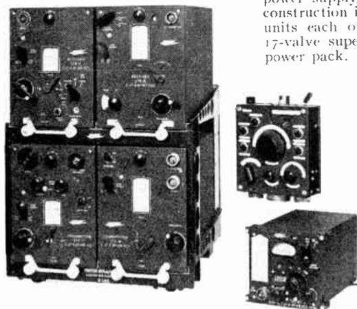
range of frequencies. The STR16 H.F. installation, for example, includes a 30-watt transmitter giving a range of about 500 miles on telegraphy at 5,000ft and 150 miles on telephony. The receiver covers 2.4 to 13 Mc/s in two bands. There is a companion 10-watt M.F. communications set covering 150 to 505 kc/s giving a range of about 150 miles and including D.F. facilities. It is described as the STR17.
