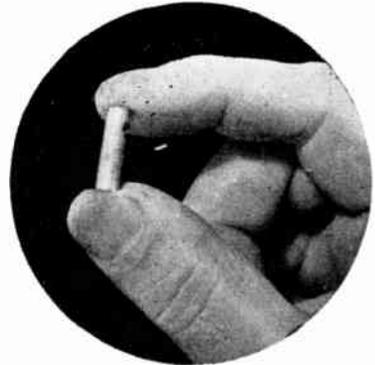
Indicating the size of a typical Transistor semi-conductor triode.
