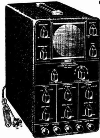
A general purpose instrument incorporating a high sensitivity electrostatically deflected 3½ in. tube. A linear time base covering 10-10,000 c.p.s. with coarse and fine frequency control is provided. Horizontal deflection can also be obtained at 50 c.p.s. or from an external source. Push-pull amplification for the vertical plates up to 100 k/c is provided.
