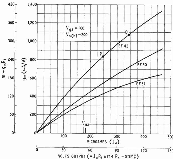
Fig. 5. Slope/anode-current or gain/output curves for three types of valve for  $V_2$  duty.  $V_{N2}$  is the zero  $V_{1g1}$  point using a G.120 1B for N<sub>2</sub>.
