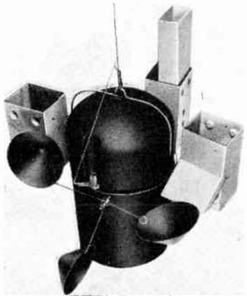
Radio sonde meteorological balloon transmitter shown by Salford.
