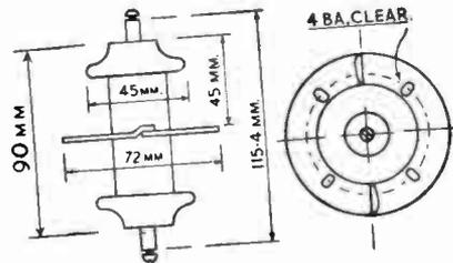
This new Ceramic "Hi-Load" Capacitor has been specially designed as H.T. or Heater By-Pass and Lead-Through Capacitor. Although very small in dimensions the capacitor has a capacitance of 1,000 pF and it is rated at 40 KVA R.F. with a maximum R.F. current of 20 amps. The sturdy rod forming the lead-through connection is capable of handling all normal currents. The high rating also makes the capacitor suitable as a tank capacitor.
