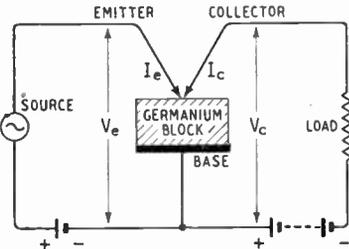
Fig. 1. Basic circuit of the Transistor.
