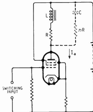
Fig. 4. Valve-controlled relay with surge suppressor shown dotted.
