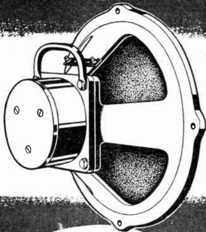
Rigid diecast chassis ; square casting for the magnet seating, secured with large hexagon head bolts ; centre pole and bottom plate all in one forging ; ring-clamped cone ; diecast centring ring ; practical construction matched by excellent response and high sensitivity — all made for Heavy Duty. The Truvox 12" P.M. Speaker will convince your most critical friends that your latest amplifier "has something." Truvox leaflet SH/152 gives all the technical detail — a postcard brings it to you.
