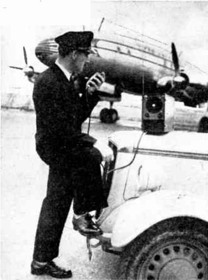
is divided into four bands, each 4-Mc/s wide, and by motor-operated switching any one of the bands can be selected from the remote control unit. The five chosen crystals can be arranged either to be all in one 4-Mc/s band or distributed over the whole range. The same crystal serves for both the transmitter and receiver.
