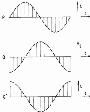
Fig. 1. At P is shown a succession of "snapshots" of the vector as seen from A, during one revolution. Seen from B, its appearance varies as shown at Q. Neither viewpoint reveals the direction of rotation. For that one has to have both views at once. Views P and Q' together would indicate reverse rotation, or negative frequency.
