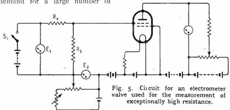
Fig. 5. Circuit for an electrometer valve used for the measurement of exceptionally high resistance.
