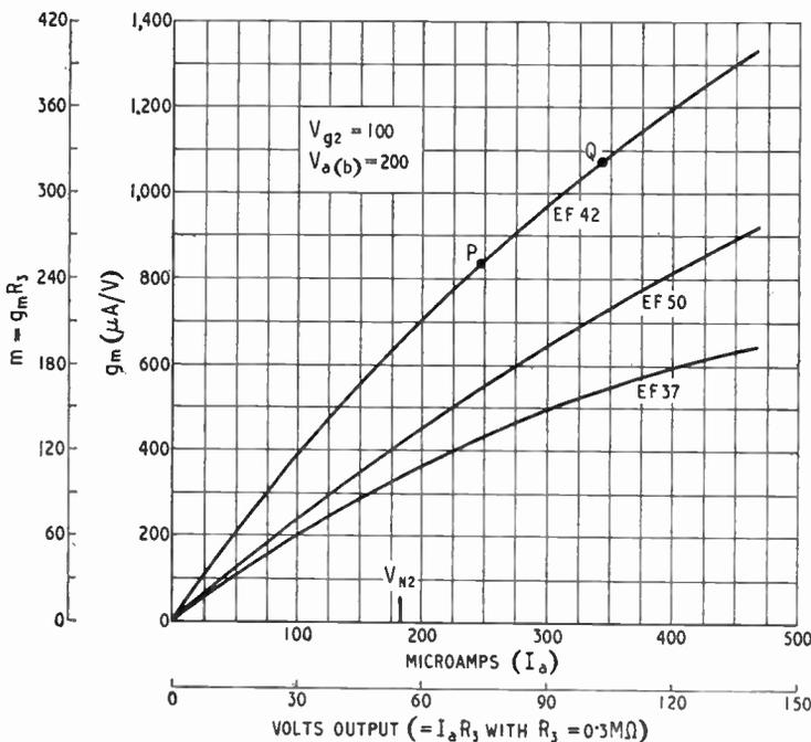
Fig. 5. Slope/anode-current or gain/output curves for three types of valve for V<sub>2</sub> duty.  $V_{N2}$  is the zero  $V_{1g1}$  point using a G.120 1B for N<sub>2</sub>.
