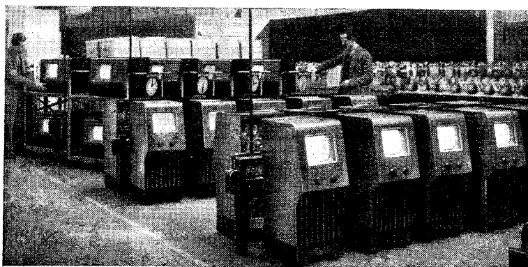
FERRANTI TELEVISION receivers undergoing an operating test during which a synchronized raster is focused on to the cathode-ray tube continuously for about four hours. This is done after all production tests have been carried out.
