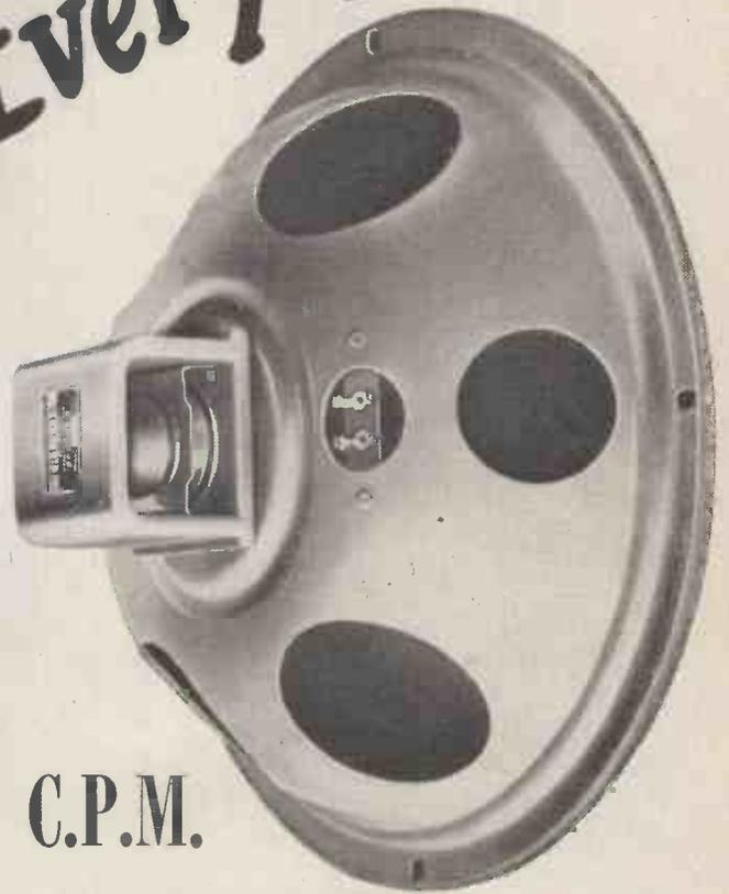
Frequency range 60-8,000 c.p.s. bass resonance 65 c.p.s.; flux density 10,000 gauss; power handling capacity 10 watt (peak). Voice coil D.C. Resistance 2.6 ohms. The specification speaks for itself. The TRUVOX 12 inch C.P.M. speaker Model BX11, marks something of an economic revolution in the high quality reproduction of sound.
