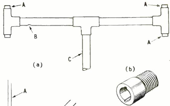
Fig. 2. The detail of the horizontal member is shown at (a) with a "close-up" sketch at (b) of one of the modified reducing adaptors.
