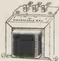
The new W.15 output transformer is illustrated on the right. The inductance is 70 H. with a leakage inductance of only 0.1 H., thus ensuring satisfactory results in wide response circuits with negative feedback. Maximum input 20 watts.
