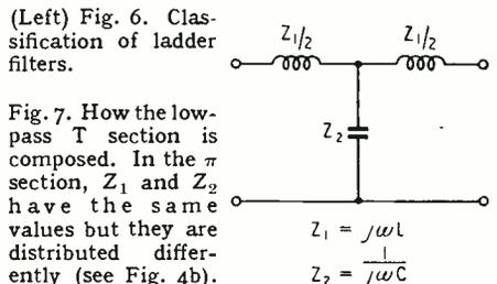
Fig. 7. How the low-pass T section is composed. In the  $\pi$  section,  $Z_1$  and  $Z_2$  have the same values but they are distributed differently (see Fig. 4b).
