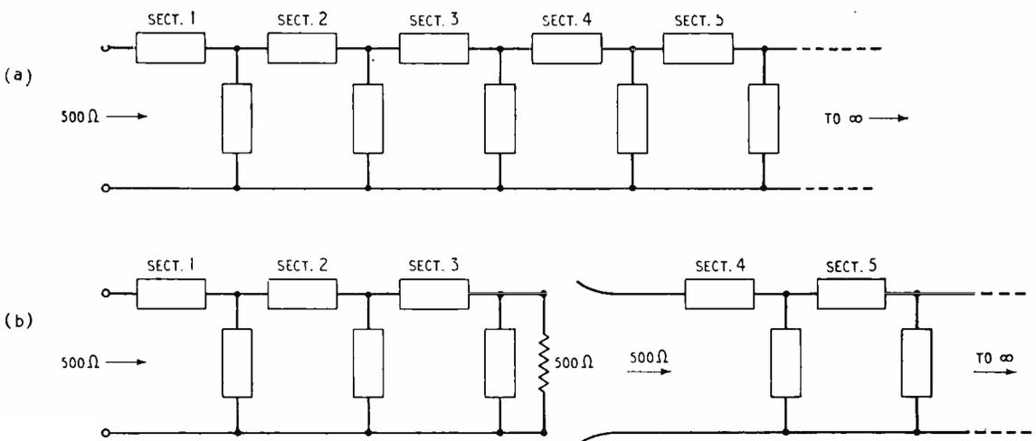
Fig. 3. If the filter chain is infinitely long, its impedance measured at the input terminals depends on itself only (a). An impedance of this value (called  $Z_0$ ) can therefore be used to simulate an infinite chain (b) and the impedance will be the same as this at the input to every section.
