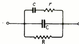
Fig. 8. Complete equivalent circuit diagram of a typical filter capacitor.
