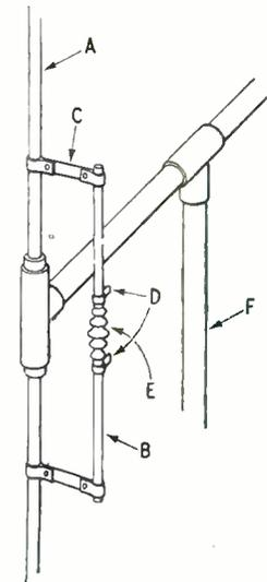
Fig. 3. Perspective sketch of the T-matching section; A = aerial rod, B = matching rods, C = brass supporting strips, D = cable-connecting clips, E = insulator, F = upper part of mast section.
