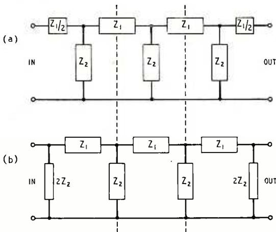
Fig. 4. By transferring half a section in Fig. 2 from one end to the other, the filter can be made to look the same from both ends. Splitting a series arm across gives T sections (a), and splitting a shunt arm lengthwise gives  $\pi$  sections (b).
