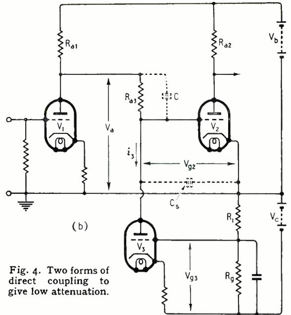
Fig. 4. Two forms of direct coupling to give low attenuation.
