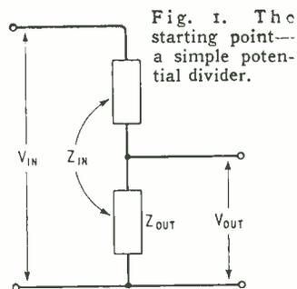
Fig. 1. The starting point—a simple potential divider.
