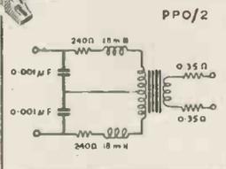
**THE** new "PPO" output transformers permit the reproduction of a full A.F. range with minimum distortion. Rating is 12w. for 0.5% harmonic distortion at 50 cycles. Six standard models are available, for accurate matching anode to anode loads of 4,000 ohms to 12,000 ohms. The secondary in each case is brought out in two sections for series or parallel connection to match a 15 ohm or 3.7 ohm load. These standard models are available from stock, other specifications can be wound to special order.
