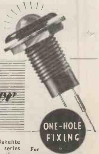
In handsome Black Bakelite holder complete with series resistance and leads, to show Pink, Red, Amber or Green, on 230v or 400v AC or DC. Specially designed for easy assembly in 1/2-inch mounting hole.
