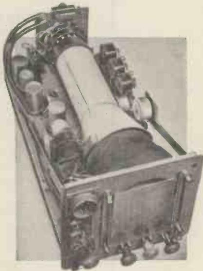
**TYPE 6 INDICATOR.** As specified for the "Wireless World" oscilloscope (reprint of data 9d.). Also for the "Inexpensive Television" (booklet 1/6), and the Mark I Televisor (constructors envelope, 2/6). These indicators are brand new, packed and sealed in manufacturer's original crates, they contain VCR97 Cathode Ray Tube, 4 EF50 valves, 3 other valves, and hundreds of useful components, including wire wound pots. Price is only £4/10/-, plus carriage and packing, 7/6.
