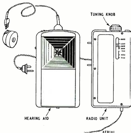
Showing inter-connections between hearing aid "transmitter" and auxiliary radio receiver unit.
