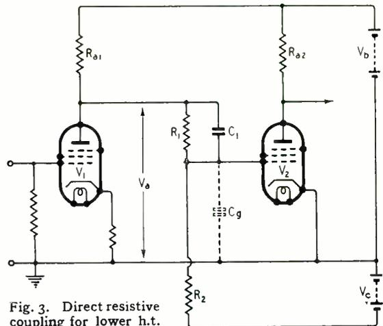
Fig. 3. Direct resistive coupling for lower h.t.
