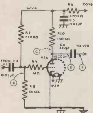
FIG. 1.—CIRCUIT OF SECOND LIMITER IN SYNCHRONIZING PULSE SEPARATOR.
