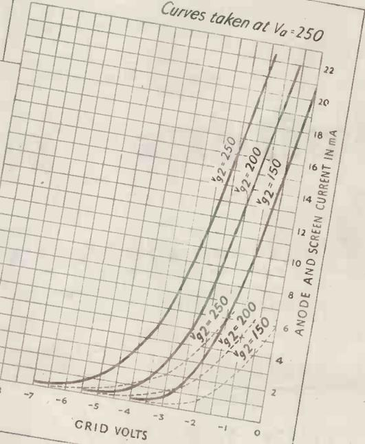
The Mazda 6F13 is a High Slope Screened R.F. Pentode suitable for use in R.F., I.F., and Video stages of a Television Receiver. It may also be used as a Mixer in a two-valve Frequency Changer Circuit.
