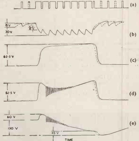
FIG. 2.—WAVEFORMS OF POTENTIAL ASSOCIATED WITH SECOND LIMITER OR FRAME SYNCHRONIZING PULSE SEPARATOR.
