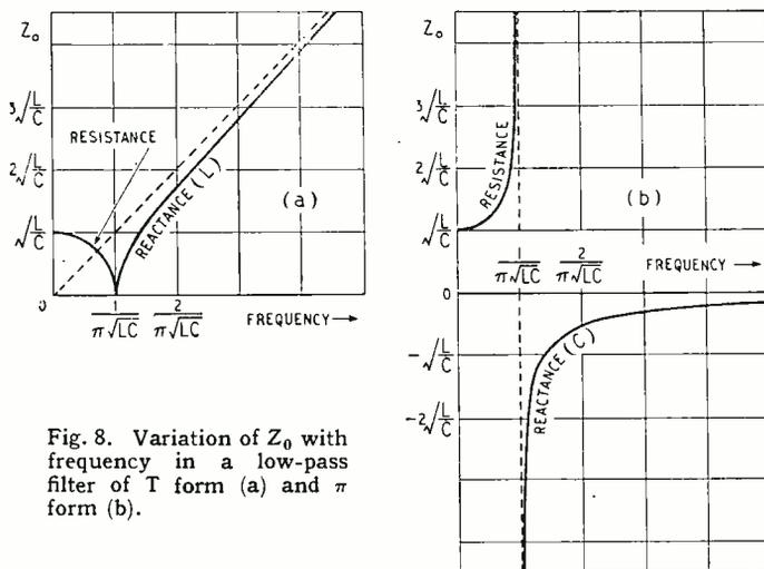
Fig. 8. Variation of  $Z_0$  with frequency in a low-pass filter of T form (a) and  $\pi$  form (b).
