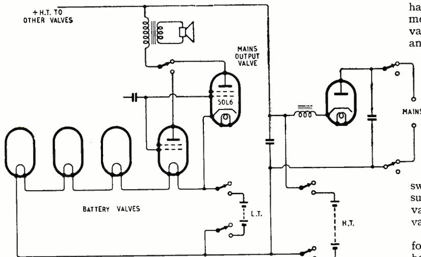
Fig. 3. Filament heating of early valves by anode current of "mains" output valve. All switch elements are, of course, ganged together.
