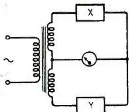
This is not as complicated as it sounds, because the frequencies are applied together in the form of a square wave. The bridge output is viewed on a cathode-ray oscilloscope, and the bridge components adjusted until the balance is obtained.
