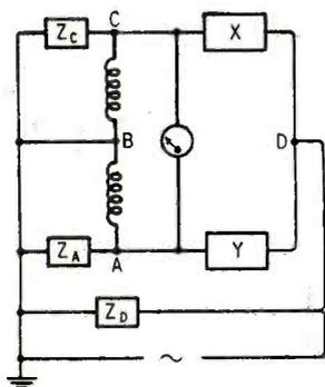
Fig. 2. Circuit with generator and detector connections interchanged.
