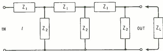
Fig. 2. Three potential-dividers (or  $\bar{\gamma}$  sections) in cascade. The influence of the load impedance,  $Z_L$ , complicates matters considerably.
