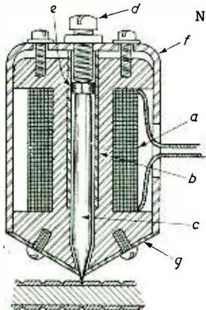
Needle-type magnetic recording head.
