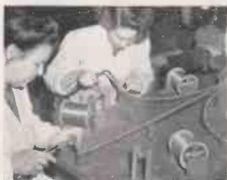
Soldering caps and wires of radio type tubular paper capacitors with *Ersin Multicore Solder* at the Dubilier Works, London.
