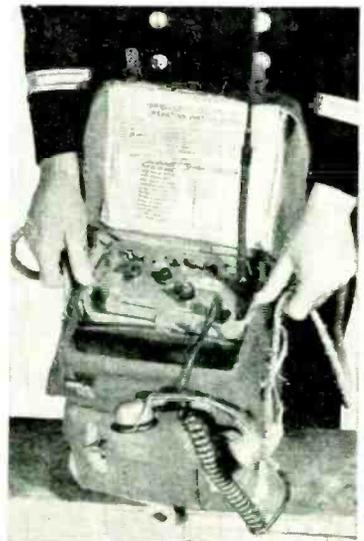
Six-channel crystal-controlled portable transmitter-receiver, Type HPS1, for use by harbour pilots.
