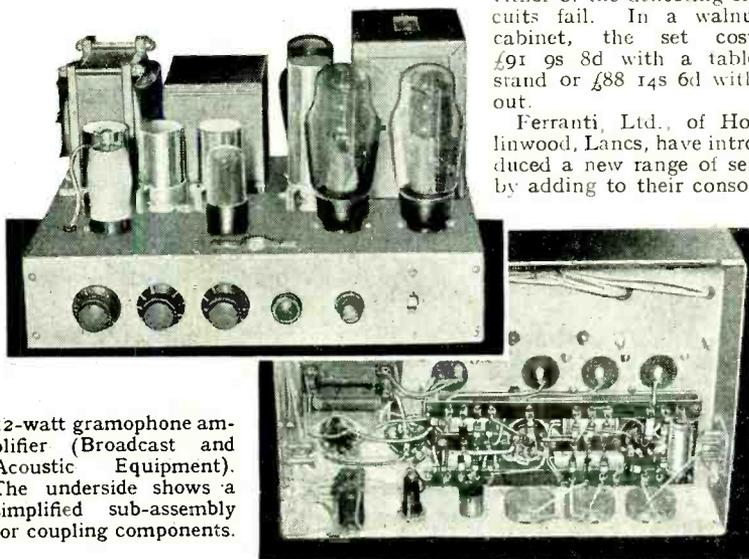
12-watt gramophone amplifier (Broadcast and Acoustic Equipment). The underside shows a simplified sub-assembly for coupling components.
