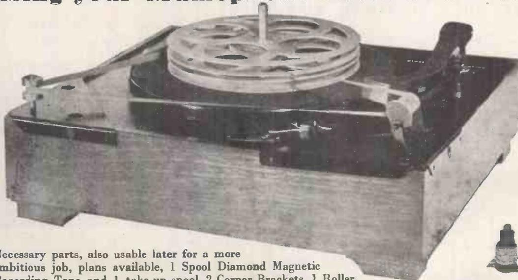
Necessary parts, also usable later for a more ambitious job, plans available, 1 Spool Diamond Magnetic Recording Tape and 1 take-up spool, 2 Corner Brackets, 1 Roller, 1 Record-playback Head Kit, 1 Friction Clutch, 1 Dual-purpose Supersonic Oscillator and Two-stage Preamplifier and your Radio Chassis. Set of parts £7 . 15 . 0, or items supplied separately.
