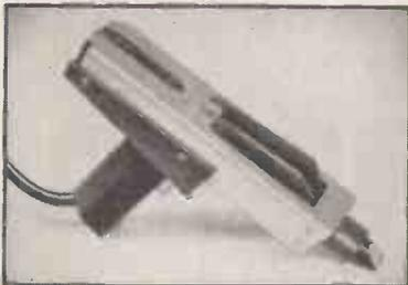
The soldering iron has a nickel silver bit driven by a magnetostriction transducer. The transducer is arranged to run at its natural resonant frequency by a feed-back system. A conventional low voltage winding heats the soldering bit.
