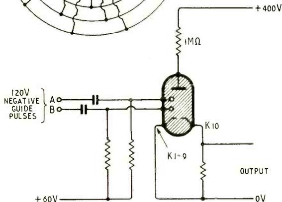
Fig. 4. Voltage diagram showing how the glow is passed from cathode to cathode by negative pulses on the guide electrodes.
