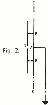
Fig. 2. Method of arranging a T-matching section.
