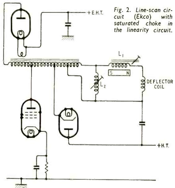
Fig. 2. Line-scan circuit (Ekco) with saturated choke in the linearity circuit.
