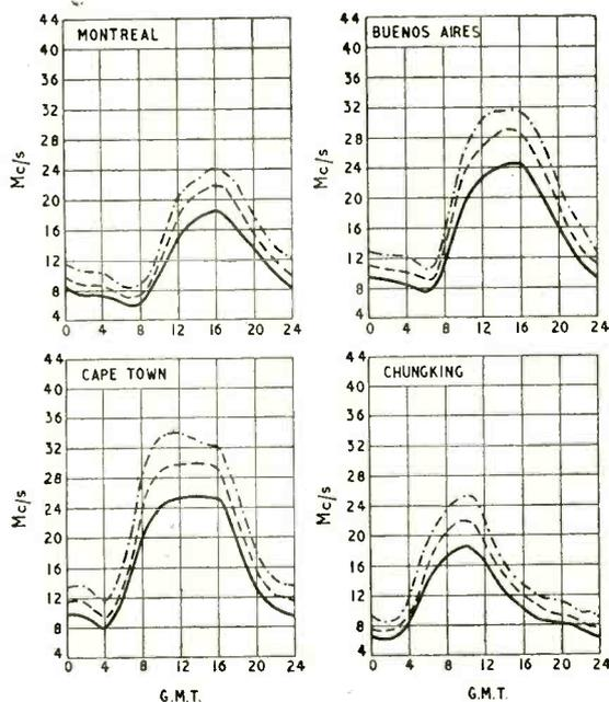
— FREQUENCY BELOW WHICH COMMUNICATION SHOULD BE POSSIBLE ON ALL UNDISTURBED DAYS
