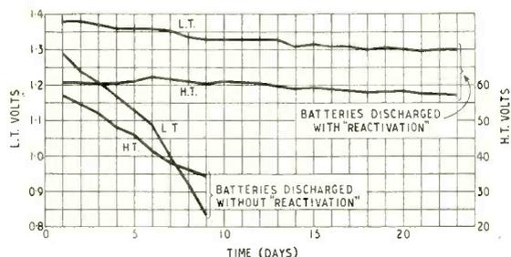
Discharge curves, taken from an N.P.L. interim report, giving the results of the first 23 days' test of the "Activette." The terminal voltages shown are the average of those measured on load at the end of each day's two-period discharge.
