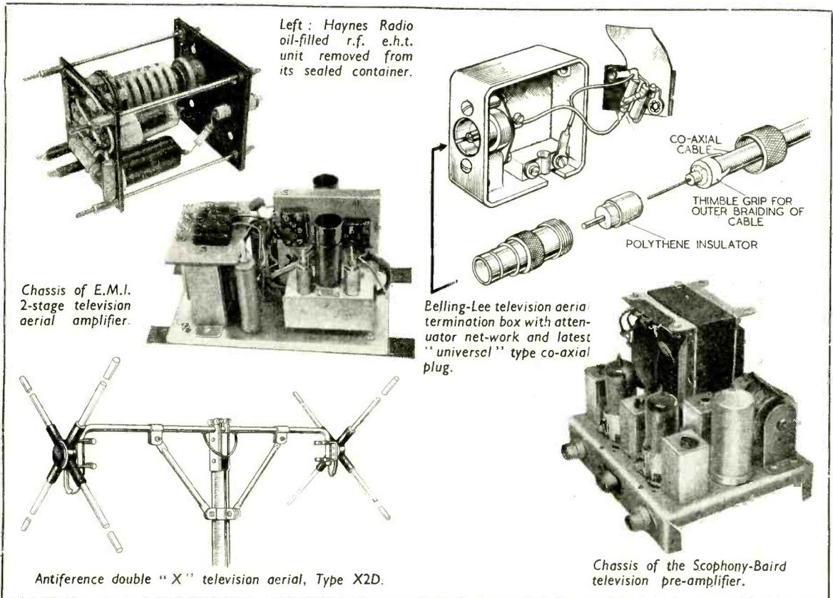
Left: Haynes Radio oil-filled r.f. e.h.t. unit removed from its sealed container.
