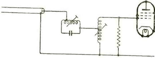
Fig. 5. I.F. input rejector used in Invicta T112.
