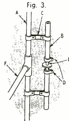
Fig. 3. Detail sketch of a T-matching section. A is the aerial rod, F the cross arm or boom, C the adjusting clips, D the cable connections, and E a disc to increase the effective leakage path of the insulator.
