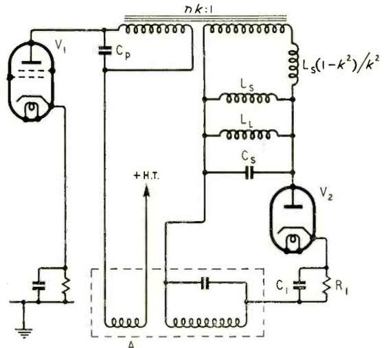
Fig. 11. Transformer-coupled deflector coil with a secondary diode.
