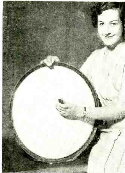
The 21-in Emiscope cathode-ray tube compared with a 1-in model, and below: Rectangular tube with 17-in diagonal (S.T.C.).
