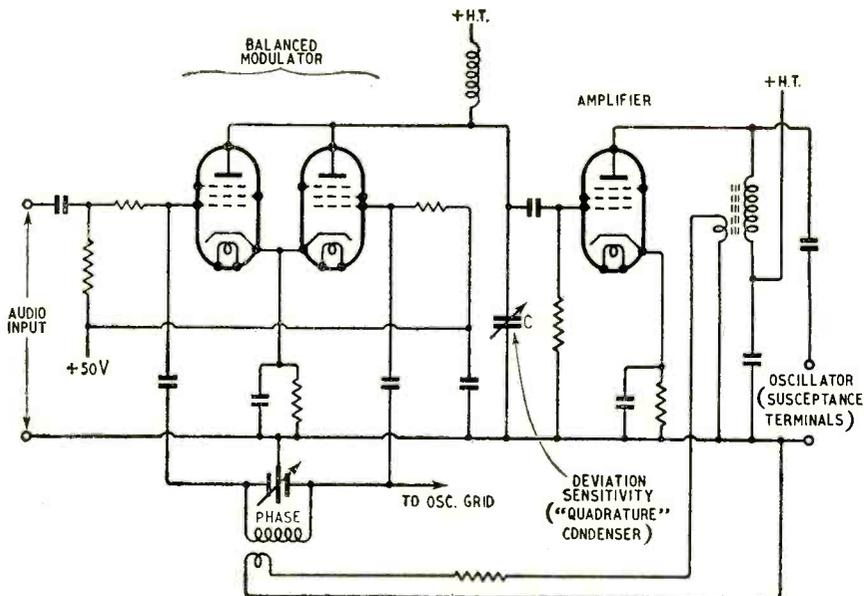
Fig. 5. Three-valve "susceptance modulator" circuit.
