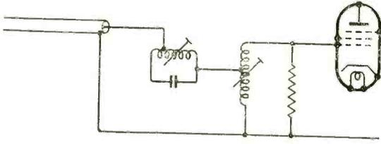
Fig. 5. I.F. input rejector used in Invicta T112.
