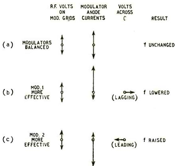
Fig. 6. R.f. phase relationships for a perfect set-up in balanced modulator.
