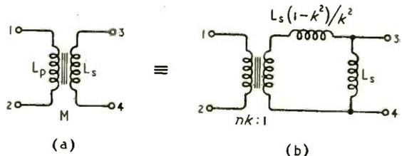
Fig. 9. Transformer (a) and its equivalent circuit (b).
