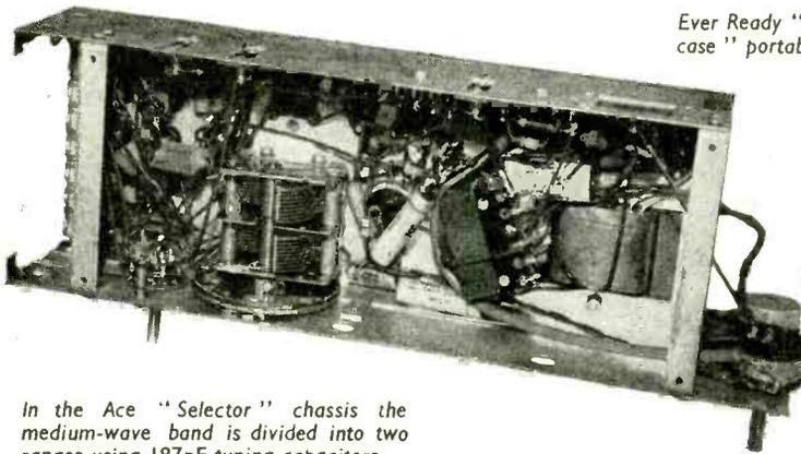
In the Ace "Selector" chassis the medium-wave band is divided into two ranges using 187pF tuning capacitors.
