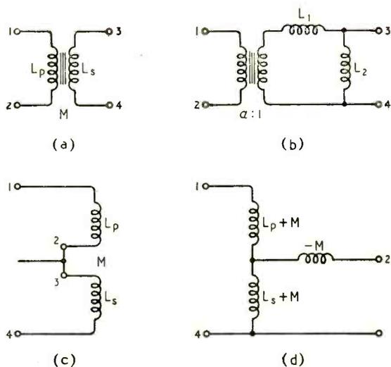
Fig. 15. Transformer (a), with its equivalent circuit (b). In auto-transformer connection (c) applies and has the equivalent (d) which can be reduced to the form of (e).
