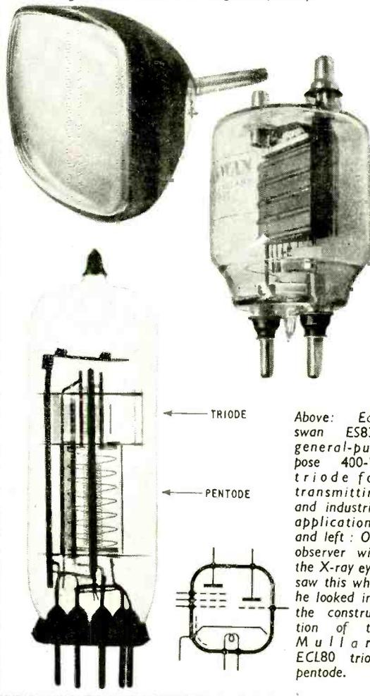
Above: Ediswan ES833 general-purpose 400-W triode for transmitting and industrial applications, and left: Our observer with the X-ray eyes saw this when he looked into the construction of the Mullard ECL80 triode pentode.
