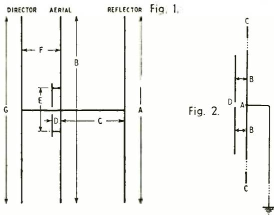
Fig. 1. General form of a three-element T-match aerial consisting of a director (G), aerial rod (B) and reflector (A).
