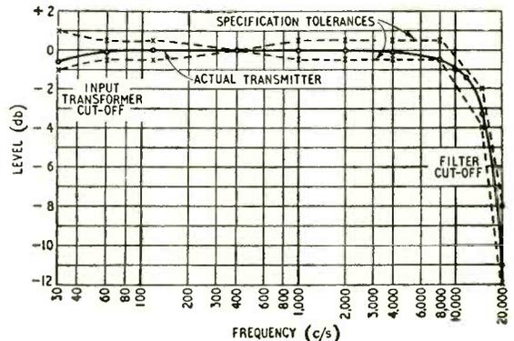
distortion measured at the site was 1.2 per cent at 30c/s. The only cause of increased distortion at low frequencies is the input transformer. At 100kc/s deviation the distortion was found to be less than 1.5 per cent.
