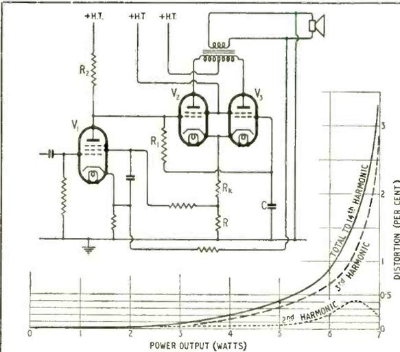
A cathode-coupled push-pull output stage in the Ferguson "300" gives low distortion with economy of components.
