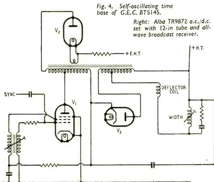
Fig. 4. Self-oscillating time base of G.E.C. BT5145.
