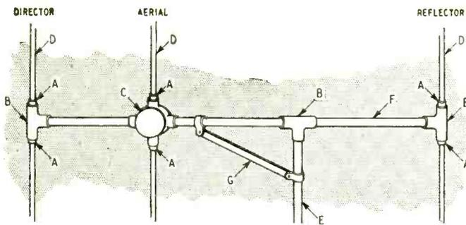
Fig. 4. Constructional details of a 3-element T-match aerial. Parts are as follows:— A, reducing socket 1 in to ½ in; B, 1-in screwed tee piece; C, 4-way circular junction box 1-in inlet or 4-way screwed junction socket if obtainable; D, ½-in dia conduit; E, 1-in dia conduit for mast section, F, 1-in dia conduit cross-arm or boom; G, support needed for 3- and 4-element arrays.
