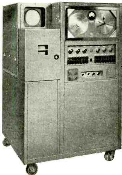
*Automatic Recorder used by the D.S.I.R. for investigating the ionosphere and demonstrated at Earls Court is made by the Union Radio Co. of Croydon.*
