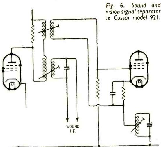
Fig. 6. Sound and vision signal separator in Cossor model 921.
