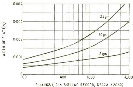
Wear on 0.0027-in radius sapphire stylus with different downward pressures. (S. Kelly)
