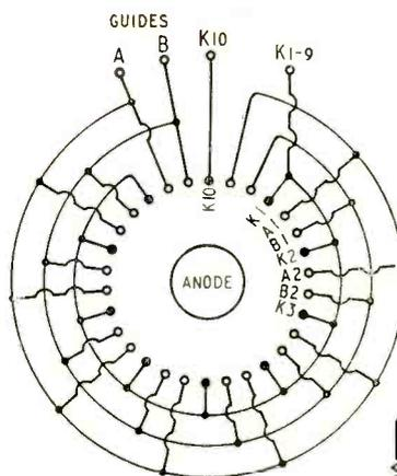
Left: Fig. 2. Arrangement of electrodes in the Dekatron tube. The ten cathodes are numbered K1 to K10. The two sets of guides, A and B, are for shifting the glow discharge from cathode to cathode.
