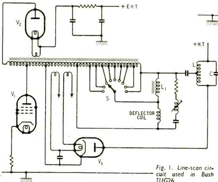
Fig. 1. Line-scan circuit used in Bush TUG26.
