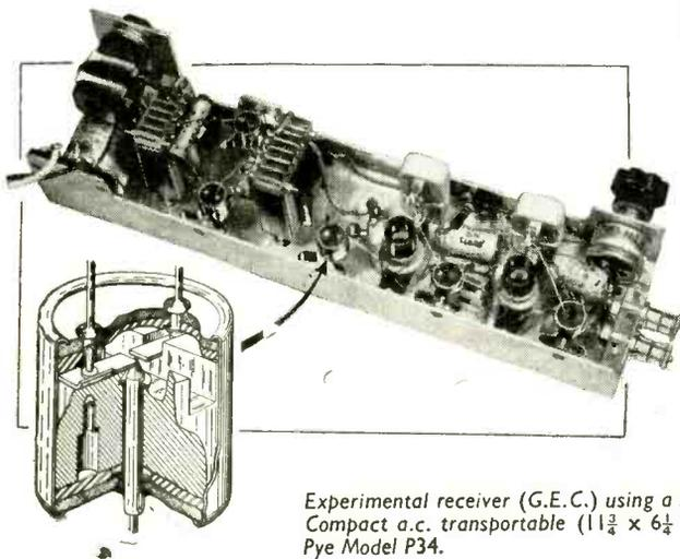
Experimental receiver (G.E.C.) using a new type of germanium crystal triode throughout, and right: Compact a.c. transportable ( $11\frac{1}{2} \times 6\frac{1}{2} \times 9$  in) with frame aerials built into a plastic cabinet—the Pye Model P34.
