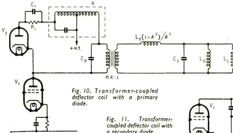
Fig. 10. Transformer-coupled deflector coil with a primary diode.
