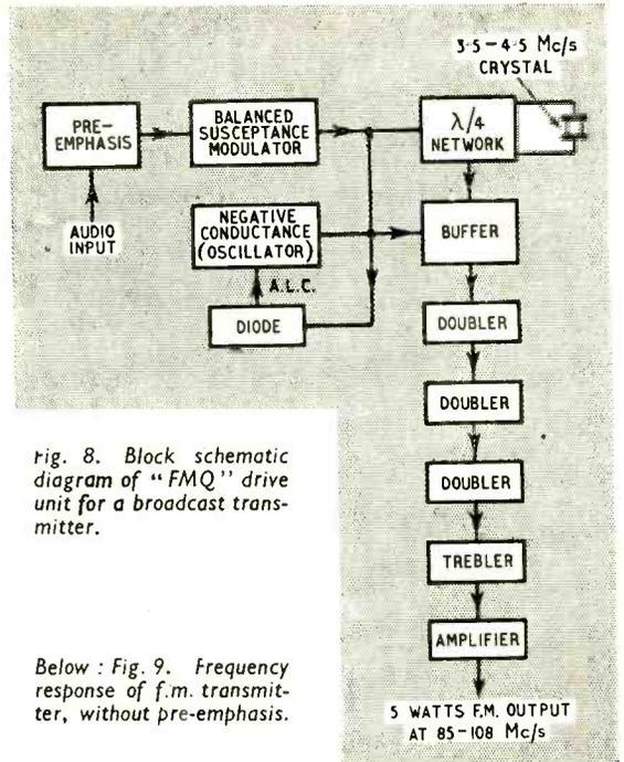
Fig. 8. Block schematic diagram of "FMQ" drive unit for a broadcast transmitter.
