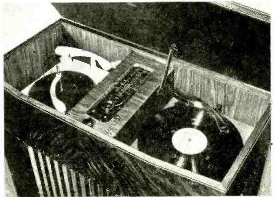
A record changer for 78 r.p.m. and a separate transcription-type turntable for  $33\frac{1}{3}$  r.p.m. records are provided in the Decca Model 96 radio-gramophone.
