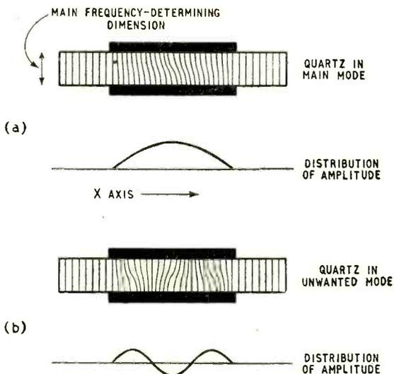
Fig. 7. Schematic diagram of section of quartz crystal showing wanted and unwanted modes of vibration.
