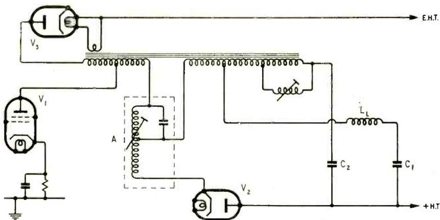
Fig. 16. Typical American scanning circuit using an auto-transformer and h.t. boost.
