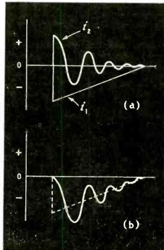
Fig. 14. The diode current is the sum of the scan current  $i_1$  and the oscillating current  $i_2$  shown at (a). The sum is indicated at (b).
