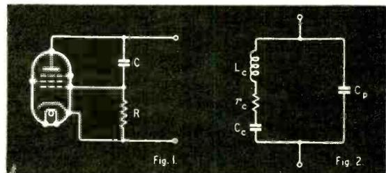
Fig. 1. Simple reactance valve circuit.
