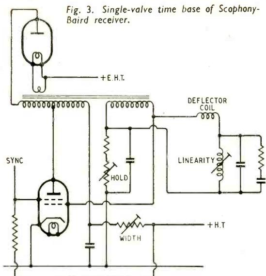
Fig. 3. Single-valve time base of Scophony-Baird receiver.
