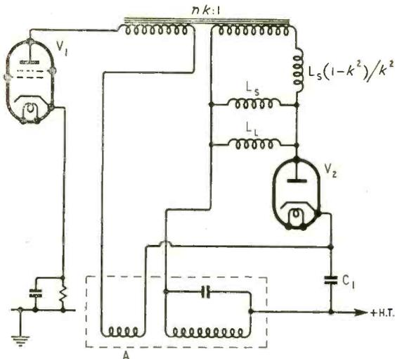
Fig. 12. Circuit of Fig. 11 re-arranged to give h.t. boost.
