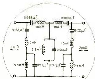
Intermodulation test set, described by E. W. Berth-Jones, showing input bandpass filter with its characteristic.
