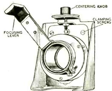
Ultra focus unit, with knurled, insulated knob for picture centering. The picture does not shift when the knob is released nor when the clamping screws are tightened.
