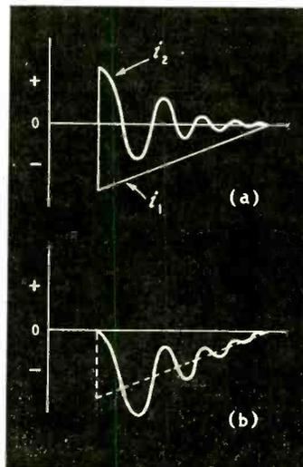
Fig. 14. The diode current is the sum of the scan current  $i_1$  and the oscillating current  $i_2$  shown at (a). The sum is indicated at (b).
