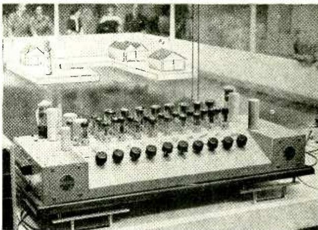
Control desk for one of the Philips radio-controlled boats at the Radio Show. In the background is the demonstration tank.
