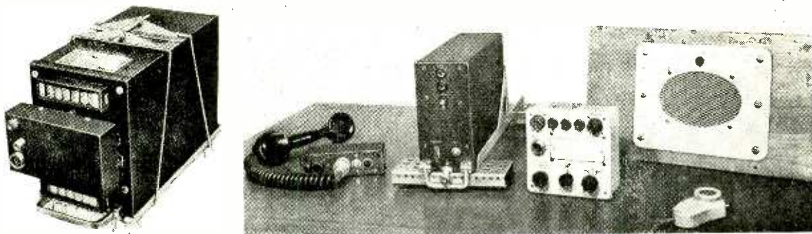
Left : Plessey Type PTR61, v.h.f. transmitter-receiver fitted with remote control attachment. The equipment provides 6 channels send and receive, for immediate operation. Right : Redifon Type A145 airborne passenger announcement system showing pilot's control (left), amplifier unit, steward's control and microphone and one of the 13 loudspeakers.
