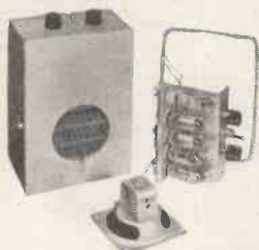
A complete Kit of Parts to build a Midget 4-valve Alldry Battery Portable Set, covering medium waveband.
