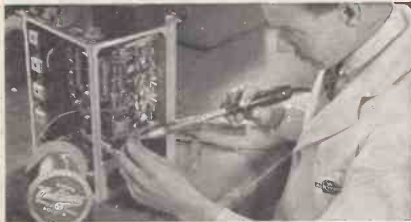
Ersin Multicore being used in servicing a modern aircraft transmitter-receiver at Airwork's Maintenance Workshops, Gatwick
