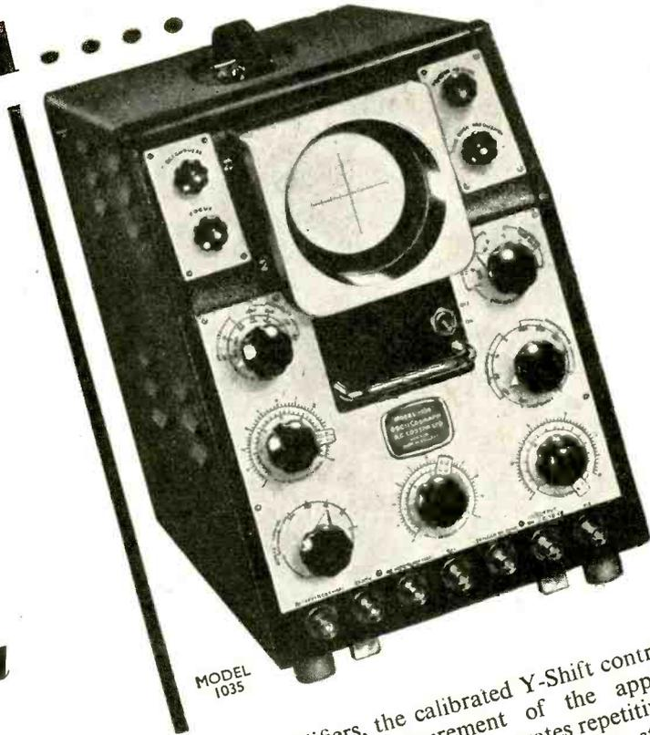
Designed by electronic engineers who are intimately concerned with the problems which technicians have to face, the Cossor Oscillograph with unique Double Beam Tube has the advantage of enabling the traces of two related phenomena to be examined simultaneously. The 4" dia. flat-faced Tube is operated at 2kV. and signals are normally fed through
