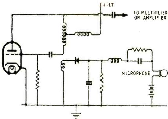
Fig. 1. Circuit diagram of a simple transmitter employing a germanium crystal to produce frequency modulation of the oscillator.
