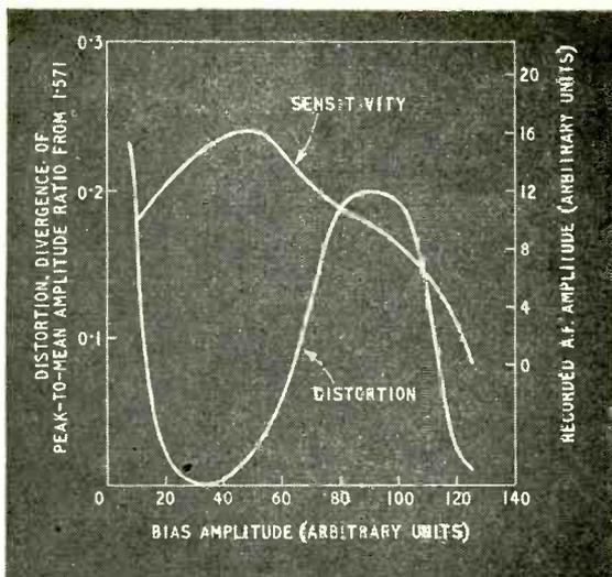
Fig. 8. Calculated variation of sensitivity and distortion with bias amplitude.
