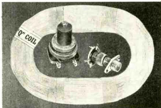
Specimens of Osrom miniature coils and spiral-wound frame aerial.
