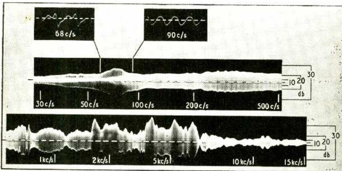
Fig. 1. Oscillographic record of a 10-in loudspeaker, with corresponding waveforms at 68 and 90 c/s.
