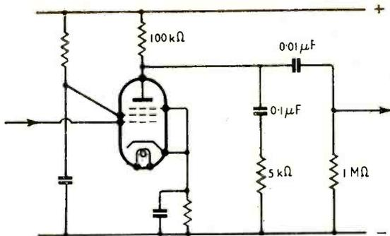
Fig. 8. Circuit designed as described, to compensate for loss of bass in gramophone recording.
