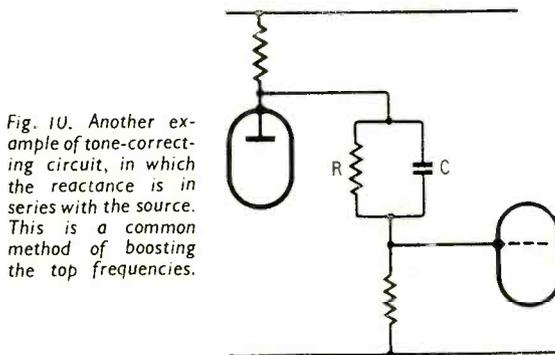
Fig. 10. Another example of tone-correcting circuit, in which the reactance is in series with the source. This is a common method of boosting the top frequencies.
