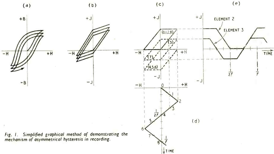
Fig. 1. Simplified graphical method of demonstrating the mechanism of asymmetrical hysteresis in recording.
