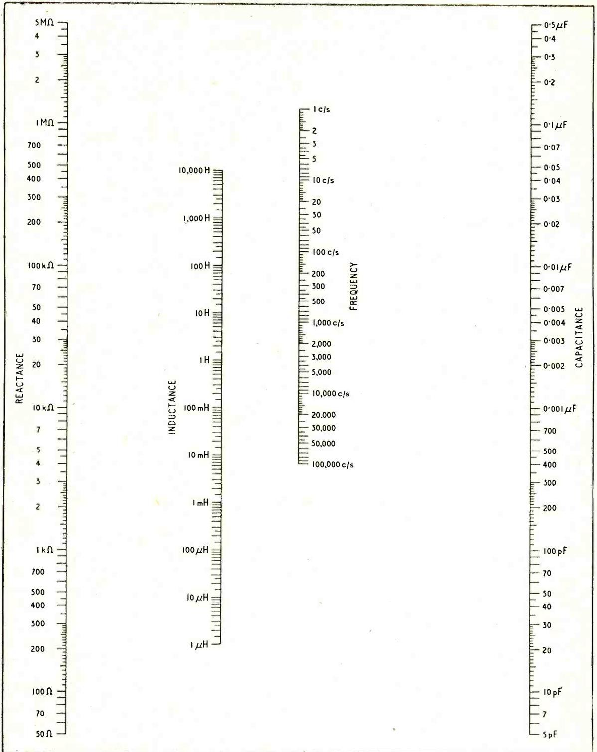
Fig. 4. By using a stretched thread or ruler edge to pass a straight line through any values on two of the scales (such as a capacitance and a frequency) the same line points out the corresponding values on the other scales (such as the reactance of that capacitance at that frequency, and the inductance which would tune that capacitance to that frequency).
