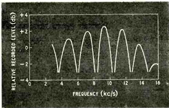
Fig. 5. Overall frequency response with 550- $\mu$  recording and 20- $\mu$  reproducing head. Tape speed 47.25 in/sec. Zero bias.
