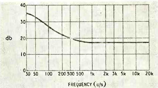
Fig. 9. Frequency characteristic of Fig. 8., including effects of 100-kΩ feed resistor, 1-MΩ grid leak, and 0.01-μF blocking capacitor.
