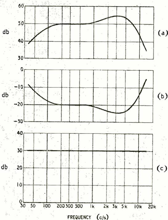
Fig. 1. (a) Example of a hilly frequency characteristic to be equalized; (b) required frequency characteristic of equalizer; and (c) extremely satisfactory result of adding (b) to (a).
