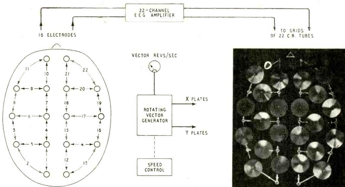
Fig. 5. Essentials of Grey Walter's "toposcope" for giving a pictorial presentation of the electrical activity of the brain. 22 small cathode ray tubes are mounted in a transparent plastic screen (right) which represents the arrangement of electrodes on the patient's head (left).
