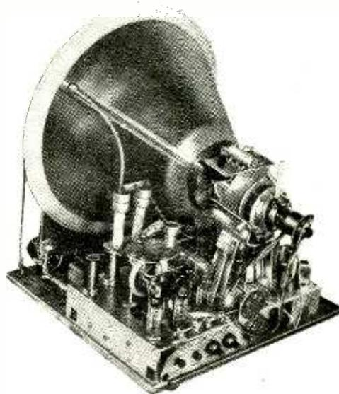
Ferguson Model 989T television receiver with 16-in metal tube.
