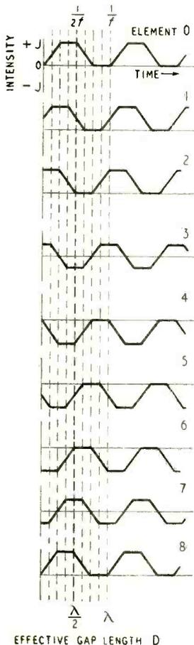
Fig. 3. Waveforms developed by recording gaps of different length, and plotted from amplitudes indicated by vertical intercepts in Fig. 2.
