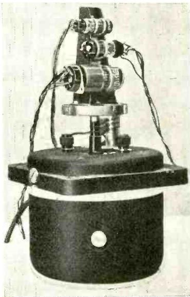
Goodmans industrial vibration generator set up for testing miniature valves.
