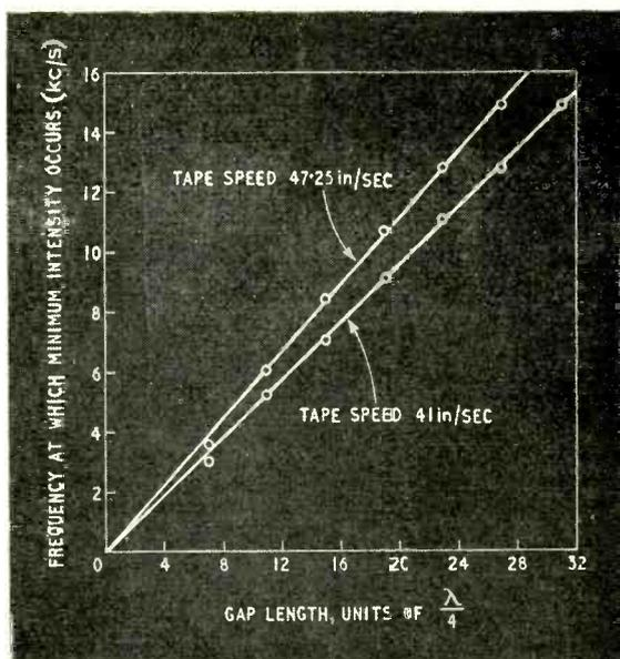
Fig. 6. Relationship between gap length and frequency at which minima occur.
