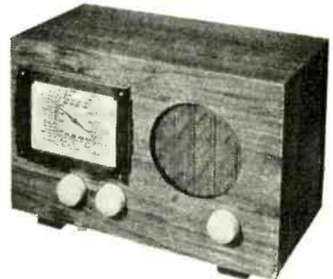
A Midget 3-valve T.R.F. Receiver for operation on A.C. mains, covering long and medium wavebands.
