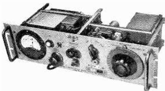
*Quartz crystal activity test set shown by Salford Electrical Instruments.*
