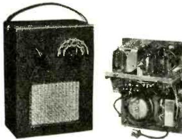
The simple design of this Receiver is so arranged that either a 3-valve Set or a 2-valve (afterwards easily converted to the 3-valve) can be made.
