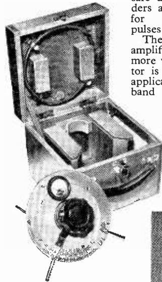
Field potential divider and remote indicator unit comprising 20-100 kV voltmeter (Hivolt).
