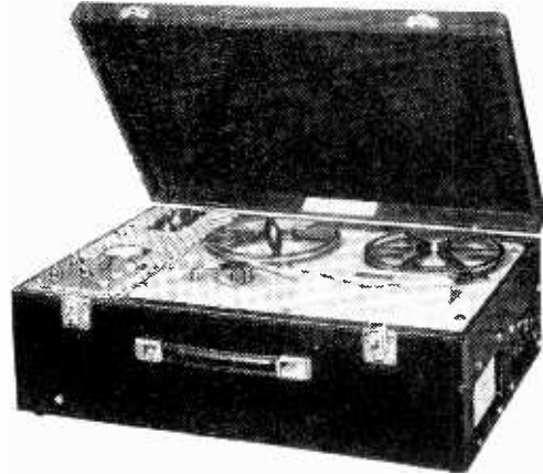
The amplifier, speaker and case, with detachable lid, measures 8½ in. x 22½ in. x 15½ in. and weighs 31 lb.
