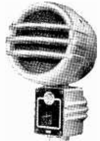
The UNICORN, model H21. A miniature exponential horn type speaker of novel design and construction (prov. patent). Ideal for noisy locations, vehicles, etc. Handling capacity approx. 5 watts, impedance 15 ohms.
