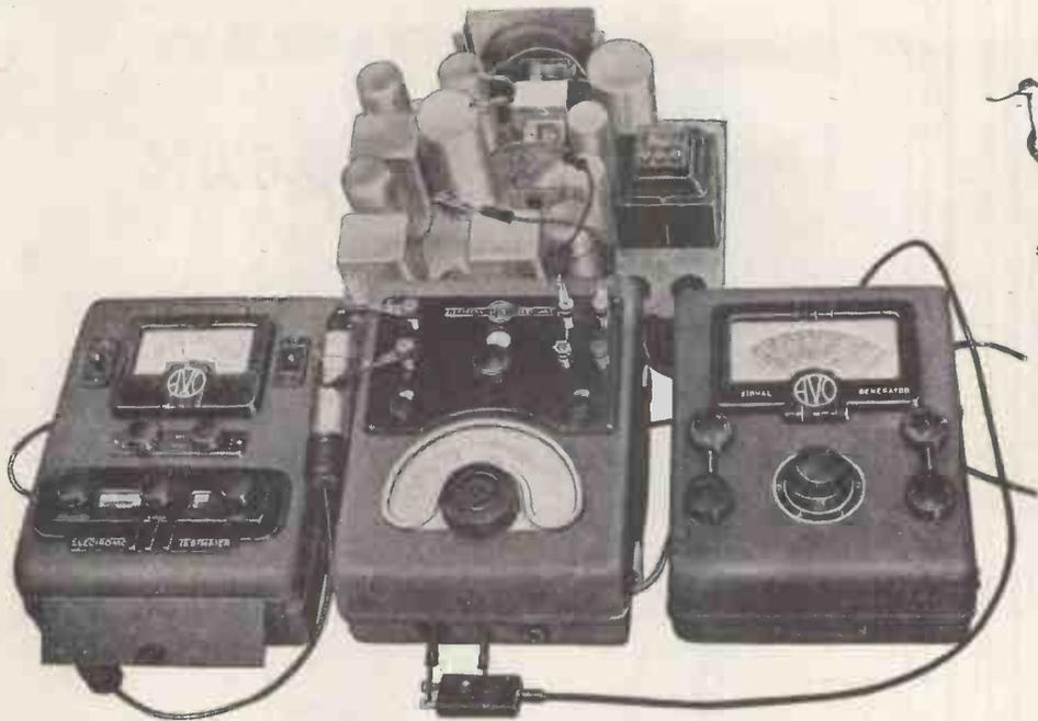
The illustration depicts a set of modern "AVO" testgear being used to measure the "Q" of the secondary winding of the second I.F. transformer on a chassis of unknown characteristics—just one of many tests which can be performed by this combination of instruments.
