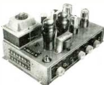
prevent audio frequencies from getting into the erase head via the bias feed network. A biased neon lamp level recorder is fitted, and calibrated on each individual amplifier.
