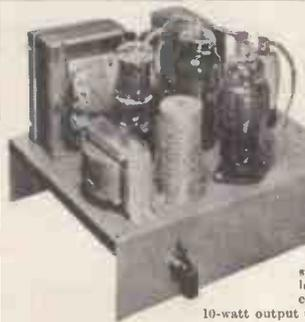
A 4-VALVE QUALITY "PUSH-PULL" 6-8 watt AMPLIFIER for A.C. mains. Incorporating Negative Feedback. Filter Input Circuit and employing 6V6's in Push-Pull. A simple arrangement is provided to enable either a magnetic-crystal or lightweight pick-up to be used, and is suitable for use with Standard or long-playing records. A tone control is incorporated, and the 10-watt output transformer is designed to match
