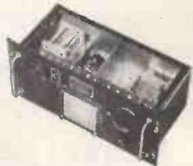
TU.7B Range 4,500-6,200 Mc/s. Ask for X/H29. TU.8B Range 6,200-7,700 Mc/s. Ask for X/H30. TU.9B Range 7,000-10,000 Mc/s. Ask for X/H467. EITHER UNIT 10/- each CARRIAGE 2/- EXTRA
