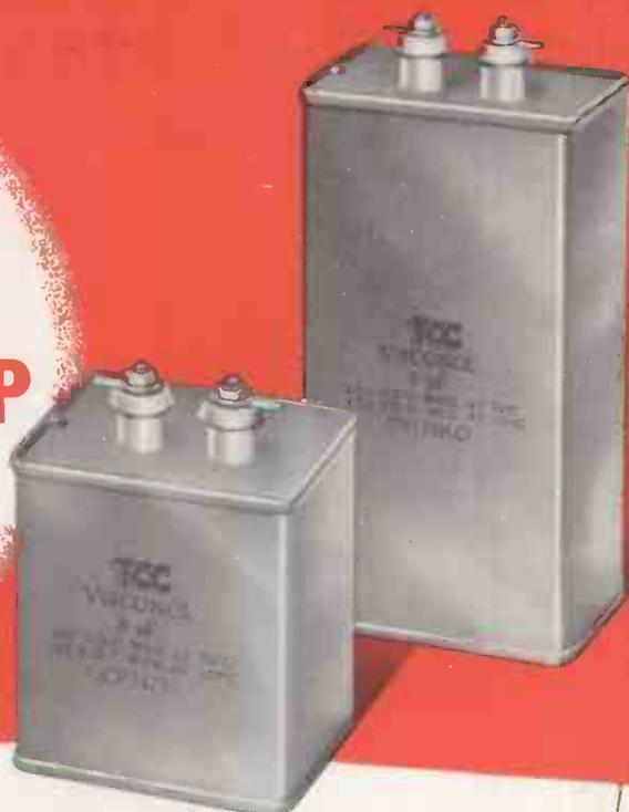
This range has several advantages over the ordinary Paper Condenser and complies with the requirements of Inter-Service Specification and R.C.L.131. Our exclusive mineral oil "Visconol", with which the paper dielectric plates are impregnated, has two outstanding characteristics: it is non-void forming, and therefore gives higher insulation voltages, and its chemical stability raises the upper working temperature limit to 100°C.
