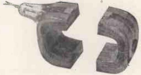
*The potting of transformer coils makes good use of 'Araldite's' excellent dielectric properties combined with outstanding adhesion to metals.*
