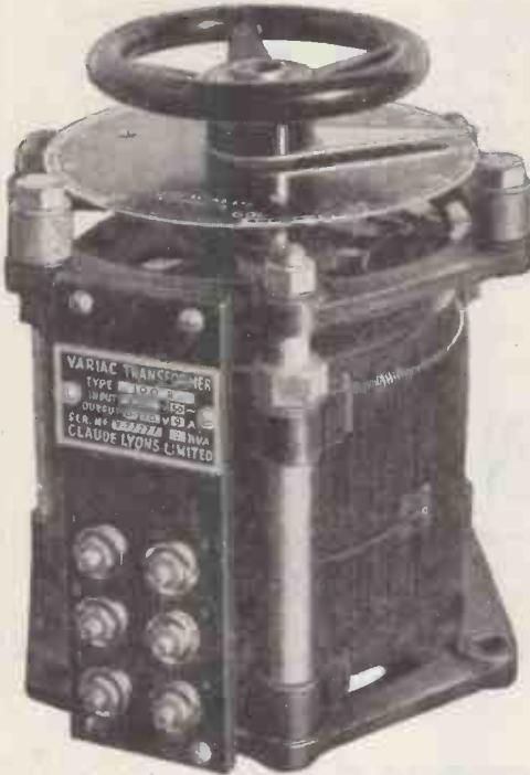
'VARIAC' infinitely variable voltage-regulating transformers are designed and constructed for many years of trouble-free operation. Not only do they supply perfectly smooth control of voltage from zero, but many types (including 100-R), also furnish output voltages considerably above line voltage while the 100-RM/2B is a dual output type. Illustration left shows Type 100-R, Rating 2,000 va., Input Voltage 230/115. Output Voltage 0-270.
