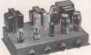
Nusound 8½ watt Quality Amplifier — PP 6V6—Independent Bass and Treble boost and cut—neg. Feedback—provision for Radio Feeder Unit—Freq. response 25 to 20,000 c.p.s. + ½dB—hums 80 DB down at 6.5 watts—Feedback 14 DB. Available with Remote Control Unit. Price £17/10/-, or as illustrated.
