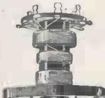
**DUAL WAVE TRF. COILS**
