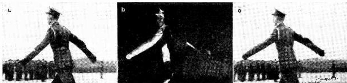
Fig. 1. Illustrating the technique of transmitting only the changes in the picture: (a) represents the first scan, and (c) the second, while (b) shows the amount by which (c) differs from (a) as a result of the figure moving to the left.
