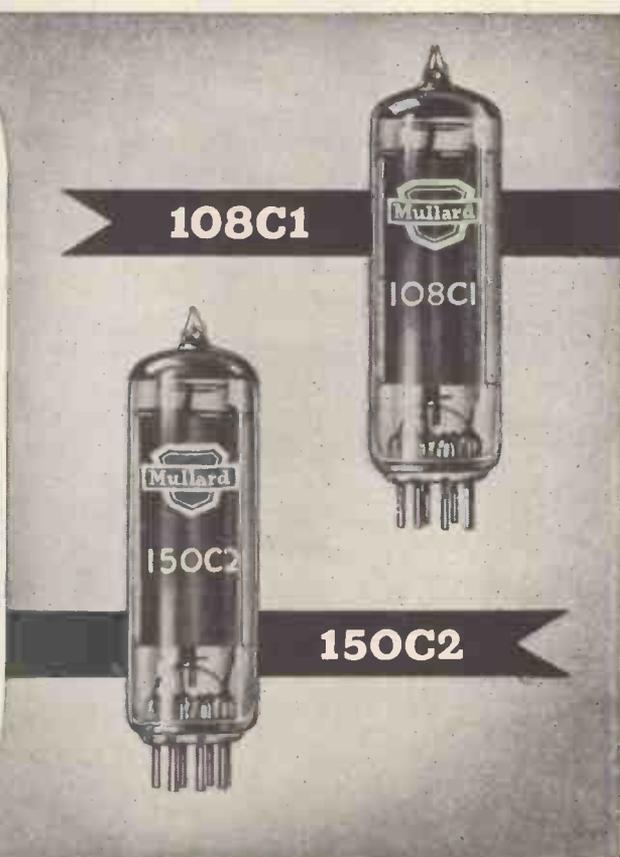
In order to meet the requirements of designers for stabilisers with very low regulation voltages, Mullard have added to their range two new tubes, the 108C1 and 150C2. They are particularly suitable for simple stabiliser circuits in which a constant output voltage is required over wide variations in input voltage and load current.
