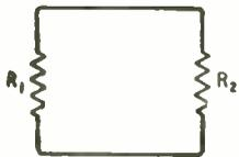
Fig. 1. Two resistances, in series or in parallel?
