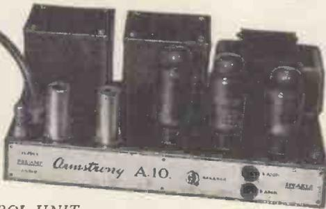
Output: 10-12 watts. Distortion: Less than .1% total harmonic at 8 watts. Frequency response: 10-100,000cps., within 1db 15-30,000cps. Hum level: Better
