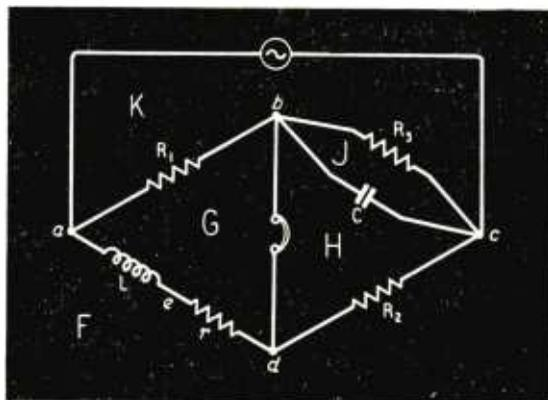
Fig. 1 (Left). Circuit diagram of the well-known Maxwell bridge for measuring inductance in terms of capacitance. There are seven potentially different currents, labelled here in the usual manner  $I_1$  to  $I_7$ . Fig. 2 (Right). The same circuit as Fig. 1, with its five meshes labelled *F* to *K* for systematic current identification.
