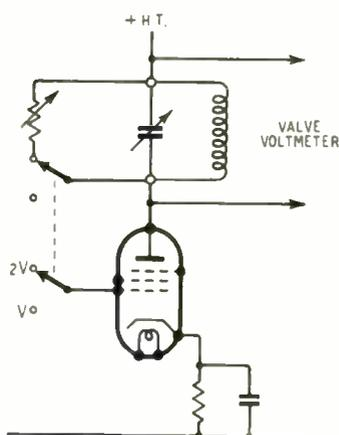
Fig. 1. (Left) Basic circuit for measurement of dynamic resistance.
