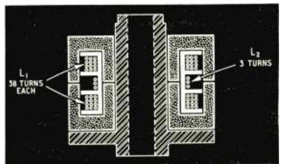
Fig. 5. Oscillator coil winding details. The coil and former are Neosid Type 10D.
