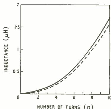
Fig. 4 (right). Inductance of smaller printed coils with  $d=0.42$  mm,  $D=0.96$  mm,  $r=4$  mm and  $R$  variable. Full line represents calculated values and the broken line measured values.
