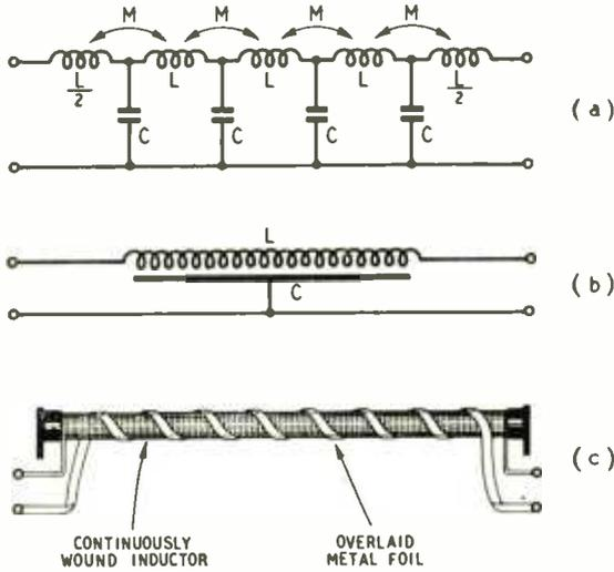
Fig. 7. Electrical delay lines: (a) lumped-constant circuit; (b) distributed-constant circuit with a practical arrangement at (c).
