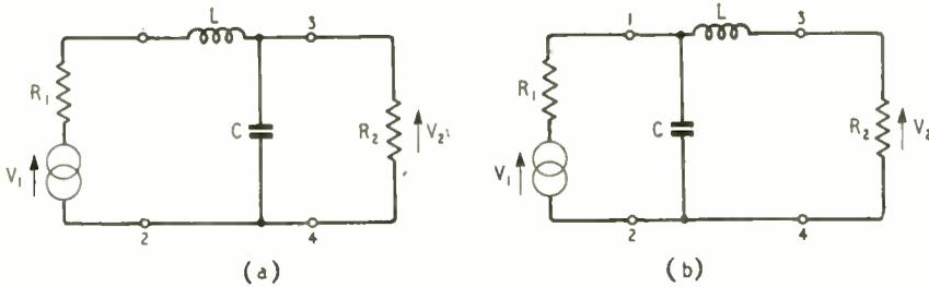
Fig. 3. The two ways of arranging the "second-order" filter.
