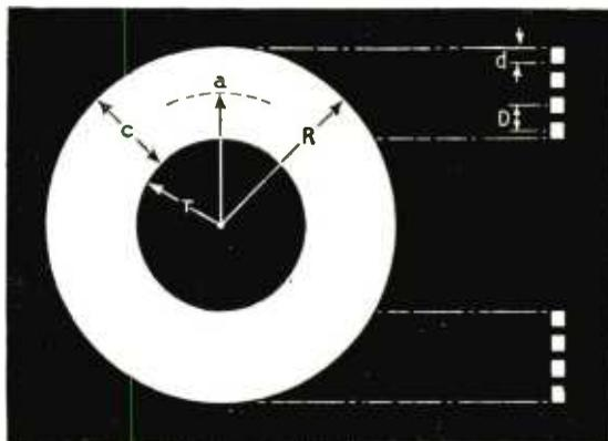
Simplified sketch of printed coil, showing meaning of abbreviations used in the Appendix and in the captions to Figs. 3, 4 and 5. ( $a$ =mean radius,  $r$ =inner radius,  $R$ =outer radius,  $c$ =depth of winding,  $d$ =width of conductor,  $D$ =pitch of winding.)
