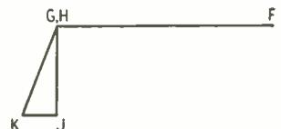
vector for  $I_{KH}$ , by putting K where a line drawn from it, parallel to  $ba$ , arrives at G. Lastly there are the two currents between  $b$  and  $c$ , one of them ( $I_{KJ}$ ) being in phase with  $V_{cb}$ , and the other ( $I_{JH}$ ) leading it by  $90^\circ$ . So there is no difficulty in drawing the corresponding vectors, to complete the triangle KJH.
