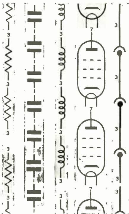
Fig. 2. Typical symbols printed on “Sellotape” strips.
