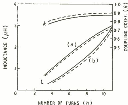
Fig. 3 (left). Inductance ( $L$ ) and coupling coefficient ( $k$ ) of printed coils with  $d=0.25$  mm and  $D=1.025$  mm. Full lines are calculated values and broken lines measured values. In curves  $k$  and (a),  $R$  is constant at 16 mm and  $r$  is variable; in curve (b)  $r$  is constant at 6 mm and  $R$  is variable.
