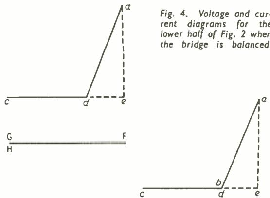
Fig. 4. Voltage and current diagrams for the lower half of Fig. 2 when the bridge is balanced.
