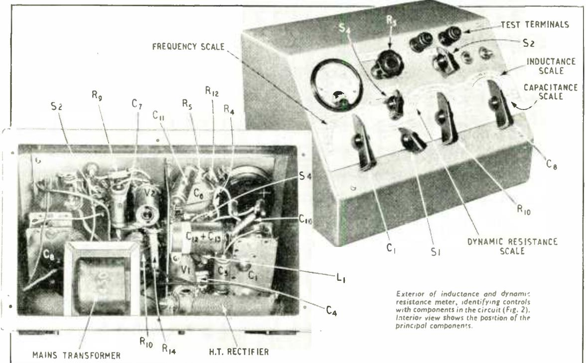
Exterior of inductance and dynamic resistance meter, identifying controls with components in the circuit (Fig. 2). Interior view shows the position of the principal components.
