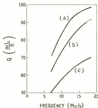
Fig. 5.  $Q$  values of various printed coils, all having  $r=4$  mm,  $d=0.42$  mm and  $D=0.96$  mm. Coil (a) has 9 turns with  $a=0.8$  cm and  $c=0.8$  cm. Coil (b) has 7 turns with  $a=0.72$  cm and  $c=0.64$  cm. Coil (c) has 6 turns with  $a=0.67$  cm and  $c=0.54$  cm.
