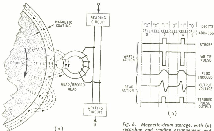
Fig. 6. Magnetic-drum storage, with (a) recording and reading arrangement and (b) waveforms representing the stored digits.
