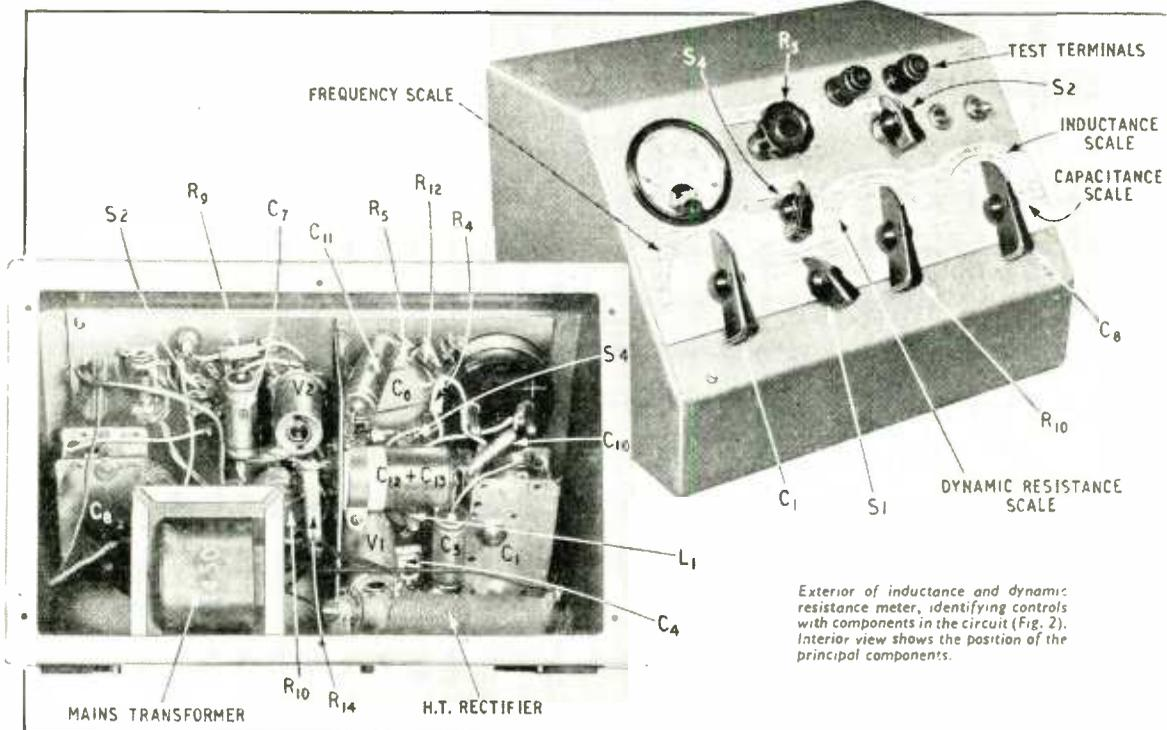
Exterior of inductance and dynamic resistance meter, identifying controls with components in the circuit (Fig. 2). Interior view shows the position of the principal components.
