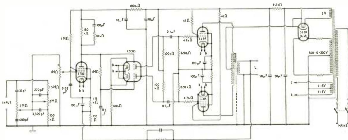
Circuit of Mullard "5-10" amplifier. The values of the cathode resistors in the output stage are 270  $\Omega$  for "normal" loading and 437  $\Omega$  for "low loading". Feedback resistor and capacitor values depend on the output impedance of the loudspeaker used.
