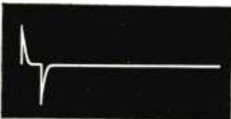
Fig. 3. Waveform of differentiated line sync pulse.
