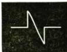
Fig. 5. Sync-pulse waveform required for ideal operation.
