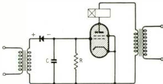
Fig. 2. Modified circuit using a thyatron valve.
