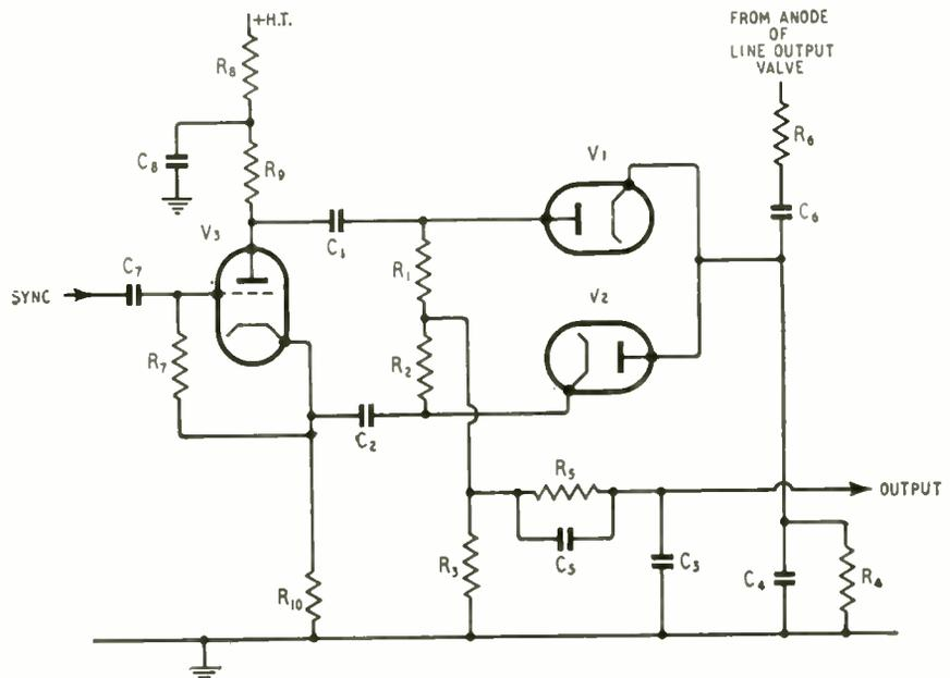
Fig. 6. Complete a.f.c. circuit using a phase-splitting input valve and showing the anti-hunt capacitor  $C_5$ .
