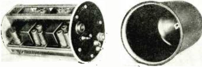
Fig. 2. Airborne electronic equipment totally enclosed in a sealed container.
