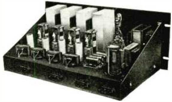
Four-channel unit transmitting d.c. warning signals over P.O. lines in event of programme failure at a substation.
