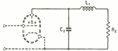
Fig. 6. In designing an output transformer we begin with this low-pass circuit.
