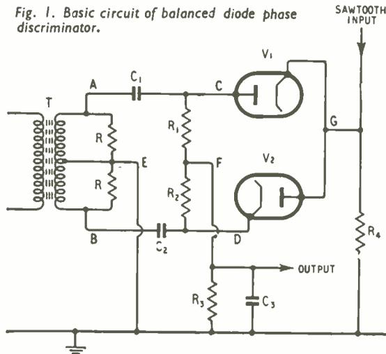
Fig. 1. Basic circuit of balanced diode phase discriminator.
