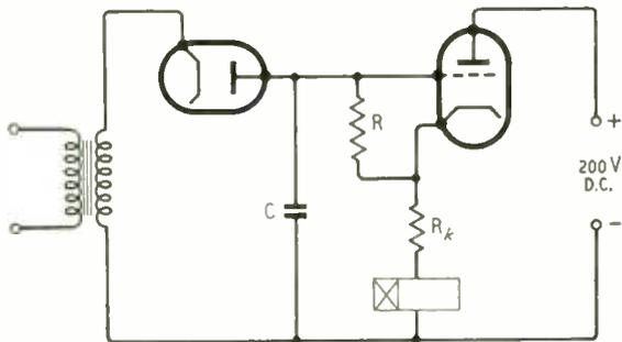
Fig. 1. Basic circuit of signal-operated switching system described in the text.
