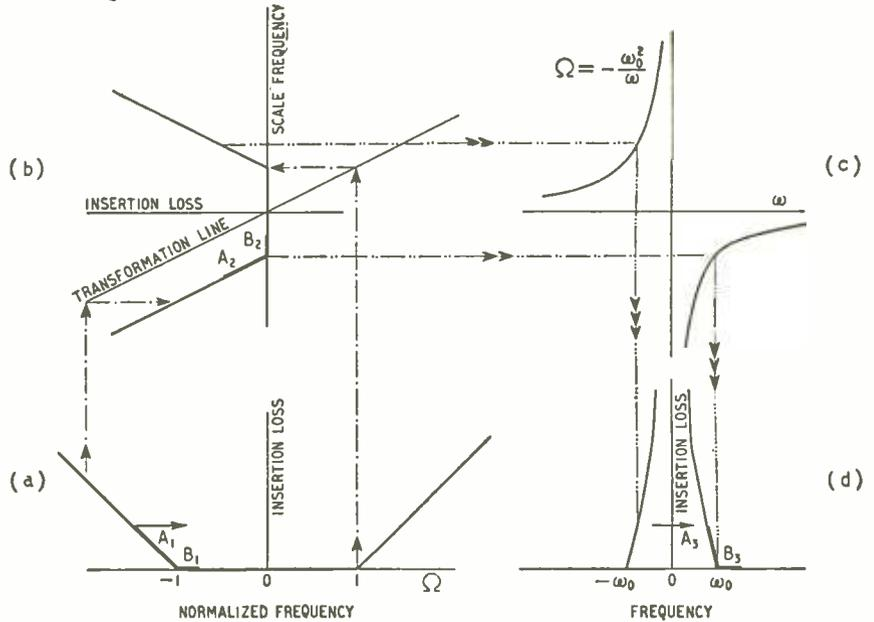
kind of thing: since it had, at its first appearance, the dimensions (frequency/frequency) there is no dimensional limitation. So long as  $Z$  and  $Y$  are proportional to  $\Omega$  we get the filter type insertion loss characteristic.
