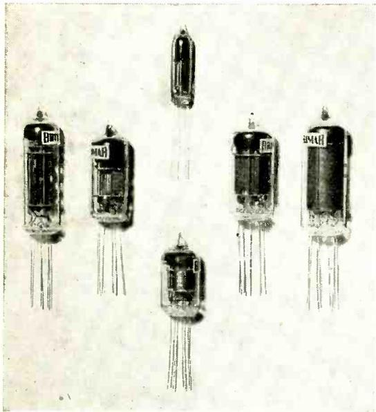
Fig. 6. Typical examples of flying-lead valves.
