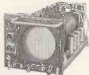
**INDICATOR TYPE 182A** Indicator contains 3 EF50, 1 5U4G, 4 SP61 and a 6 1/2 in. C.R.T. Type VCR 517, complete with Mu Metal-screen, 9 wire wound pots, with large assortment of resistors, and condensers. Can be converted to Oscilloscope (as described in "Radio Constructor.") Circuit supplied. Tubes have no "Cut Off" and can be demonstrated to callers. BRAND NEW (less relays). In original transit case, 67/6 plus 7/6 carriage.
