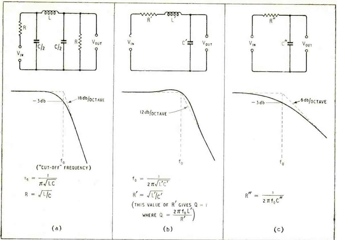
Fig. 4. The constant-k,  $\pi$ -section low-pass filter shown at (a) has the same response (to both sine-waves and transients) as that given by circuits (b) and (c) in cascade, assuming that (c) does not appreciably load (b).
