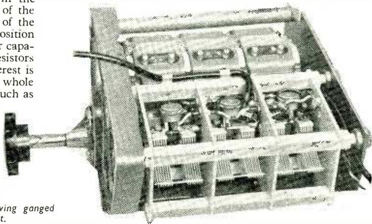
Right: Front-end unit of Eddystone 770R showing ganged capacitors, valveholders and (in rear) coil turret.
