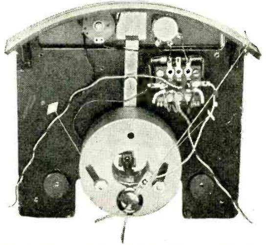
The amplifier mounted on the base plate of a 7-in scale edgewise-reading meter. Batteries are on the back of the meter case. The control potentiometers can be seen immediately below the scale and their shafts protrude through the case on either side of the mechanical set zero.
