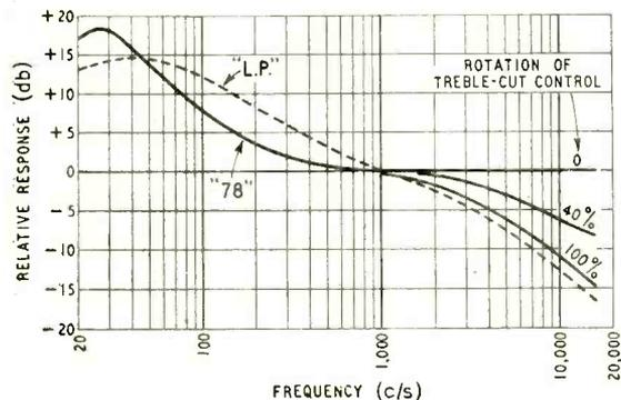
Fig. 2. Measured response curves for gramophone input stage (all components within 5% of values shown in Fig. 1).
