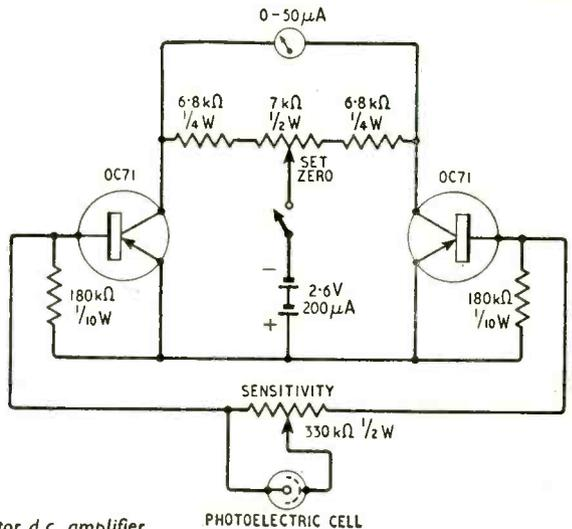
Right: Circuit of the transistor d.c. amplifier.
