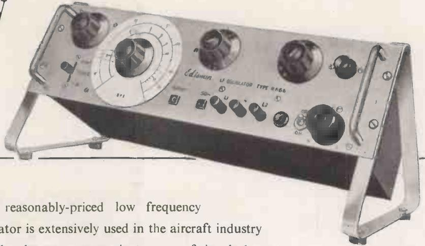
This reasonably-priced low frequency oscillator is extensively used in the aircraft industry and elsewhere as a convenient source of signals down to 1.15 c.p.s. for the testing and calibration of vibration recorders, servo systems etc. It is also widely used in medical research and clinical work for the calibration of biological amplifiers and recorders, and low frequency wave analysers.
