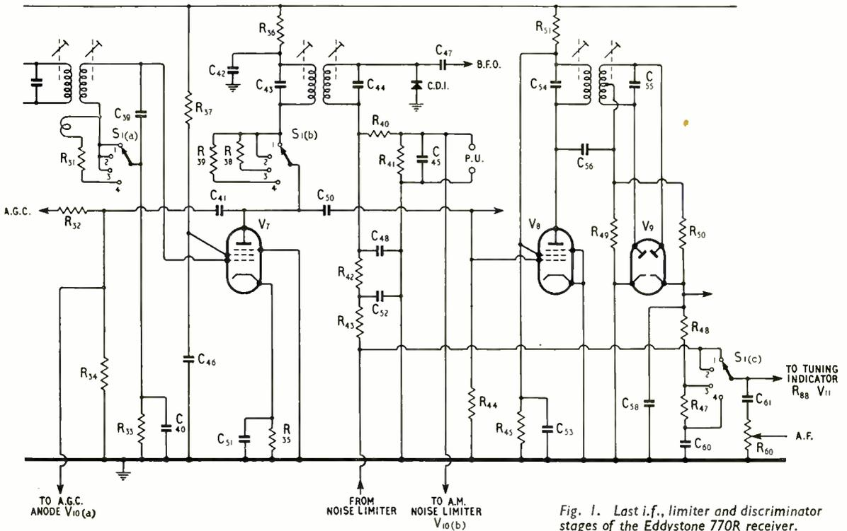
Fig. 1. Last i.f., limiter and discriminator stages of the Eddystone 770R receiver.
