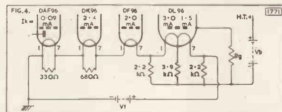
has to produce the required bias plus  $2 \times 1.4V$ , therefore it, must be a high-value close-tolerance component.
