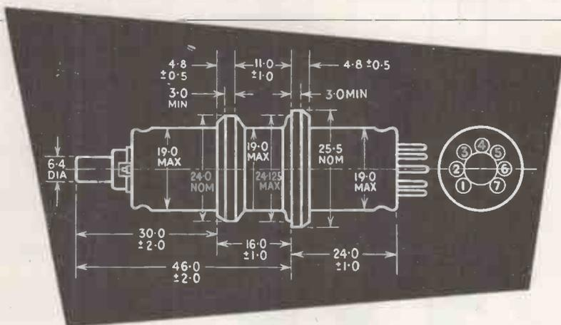
This is a low voltage, reflex velocity modulated valve for use as a local oscillator in the 10 centimetre ("S") Band. It is of the plug-in type, with disc seals for resonator connection, and is indirectly heated.
