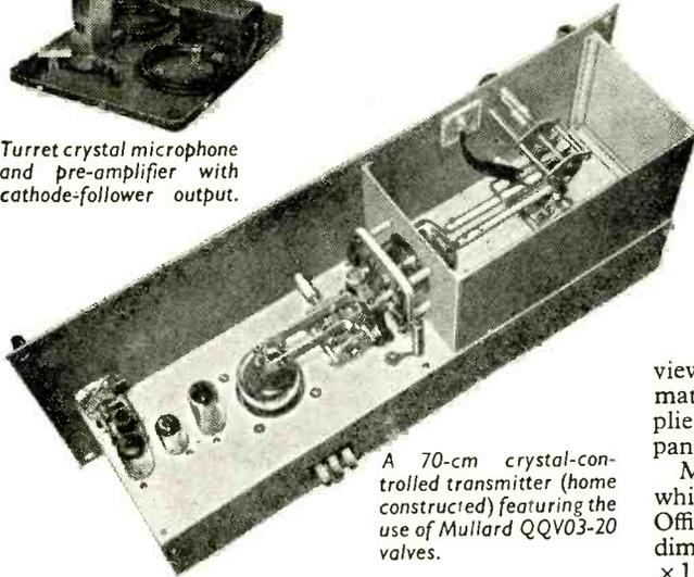
A 70-cm crystal-controlled transmitter (home constructed) featuring the use of Mullard QQV03-20 valves.
