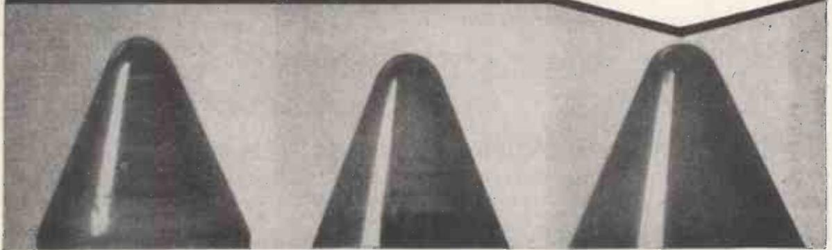
1 Polished with Diamond. 2 Tumbled by Sapphire Bearings process. 3 Flame Fashioned by Sapphire Bearings.
