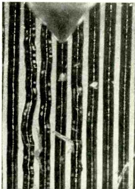
Fig. 1. Photomicrograph of record grooves before cleaning.
