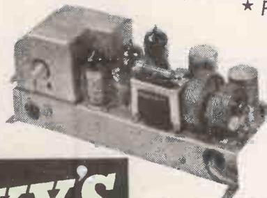
4 valves: 2 UL41 in push pull, 1 UCH42 and 1 UAF42. Input voltage 100/110 AC/DC. Very easily converted to 230 volts. Supplied with circuit diagram and full details. Size: — 9 x 4 x 4 in. Uses 2 metal rectifiers, 1 each RM2 and RM3. Ideal for ships' record players, tape recorders, home record players, baby alarms, etc., etc. Supplied complete, fully assembled and wired, with 4 valves.
