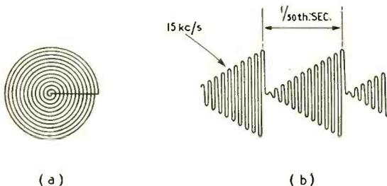
Form of the spiral scan is shown at (a) while (b) is the waveform used to produce it
