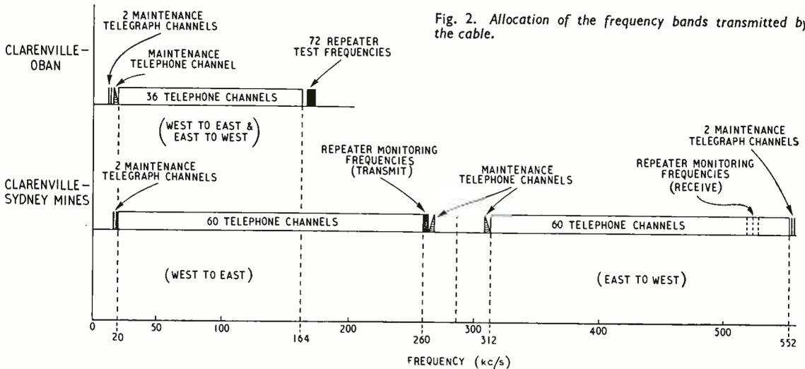
Fig. 2. Allocation of the frequency bands transmitted by the cable.
