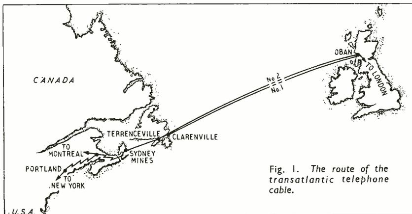
Fig. 1. The route of the transatlantic telephone cable.
