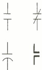
(It must be remembered that Americans draw all lines of the same thickness.) Their closed contact (right) is rather like a British variable or pre-set capacitor which has lost the end of its shaft. They avoid confusion by giving their capacitors one curved plate (left). Possibly we could persuade them to change their open contact to our symbol used in Electric Traction
