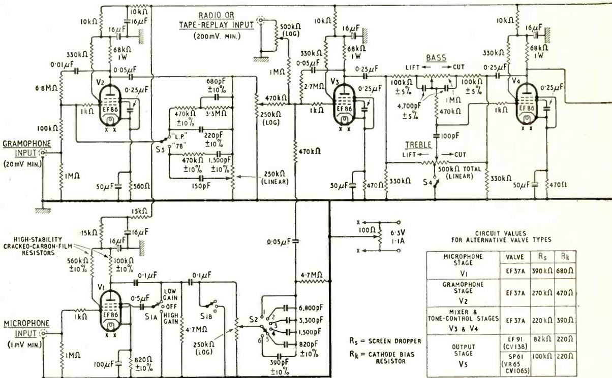
Fig. 1. Complete circuit of pre-amplifier. All resistors  $\frac{1}{2}$  watt  $\pm 20\%$ , except where otherwise specified. All capacitors (other than electrolytic)  $\pm 20\%$  except where otherwise specified. Mullard valve type EF86 may be directly replaced by Osram Z729; other alternatives require circuit changes as shown in the inset table.
