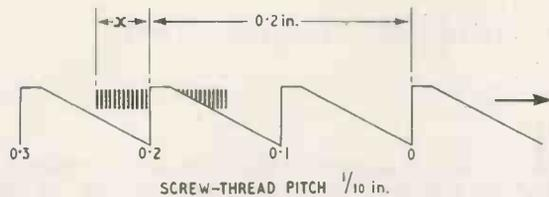
Fig. 4. Typical position of the interpolation-scale image of Fig. 3 in relation to the teeth of the coarse scale.
