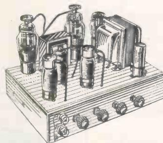
This amplifier, whilst having sufficient output to fill a small hall, is the ideal amplifier for the quality enthusiast who knows that though the average listening level is less than one watt it is necessary, for the very highest quality, to have an output of at least ten times this figure in order to obtain completely distortionless reproduction of sudden loud sounds.
