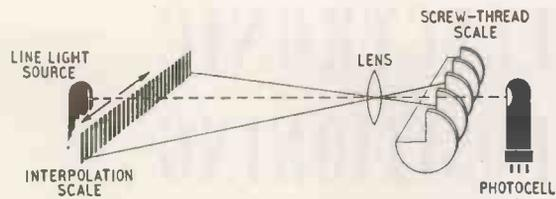
Fig. 3. Displacement measuring device using an accurately machined coarse scale and optical interpolation system.
