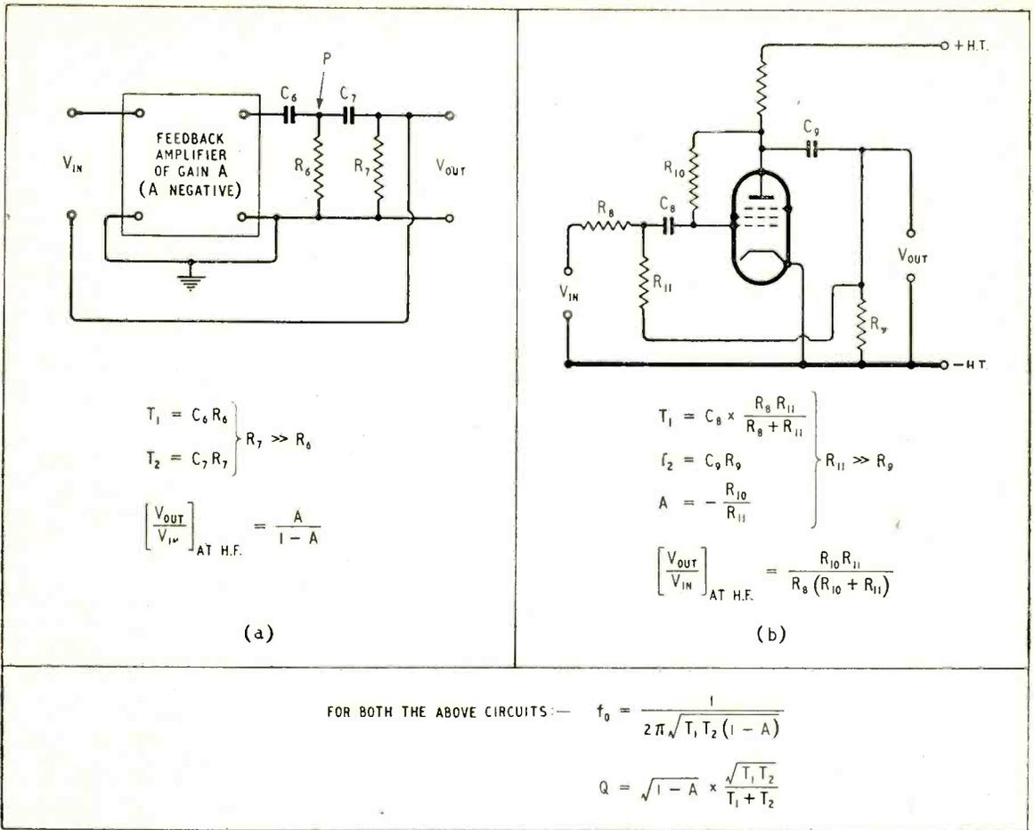
Fig. 6. Feedback circuits simulating Fig. 4 (b) with  $L'$  and  $C'$  interchanged. For simulating a constant- $k$ , high-pass filter with  $R = \sqrt{L/C}$  terminations,  $Q$  is made unity and a passive a.c. coupling,  $-3\text{db}$  at  $f_0$ , is added externally to the above circuits.
