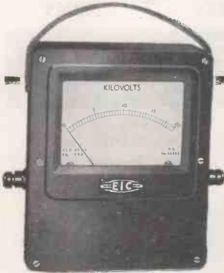
The high magnetic stability and strength of 'Sincomax' magnets makes a robust job even of a sensitive Microammeter. In this application as in many others Murex Sintered Magnets continue to give accurate and reliable service.
