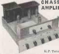
A modern high quality 12 watt Amplifier for the HOME CONSTRUCTOR, having a Valve line-up of U709, B309, Z729 and two N709's in Push Pull. The Assembly Instructions include five "easy stage-by-stage" diagrams and is available for 3/6. Price of COM-**£23/10/-** (Plus 7/6 Carr. and Ins.) WE WILL SUPPLY THE COMPLETELY ASSEMBLED (Plus 7/6) AMPLIFIER for **£25/-** Carr. & Ins.)
