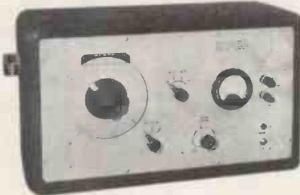
Audio-frequency Signal Generator operating from A.C. Mains. Frequency range: 50 cycles to 55,000 cycles.
