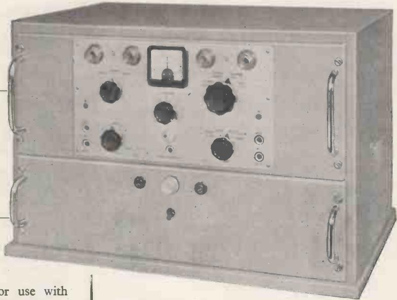
The HU.12 unit is designed for use with two suitable receivers of frequency shift or on-off telegraph transmissions in double diversity. The combined AF outputs of the receivers are converted into double current signals to operate an undulator, relay or other 'space-mark' type of equipment requiring a current up to 30 mA. No receiver modification is necessary except, perhaps, adjustment of the BFO frequency.
