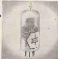
The type B7 unit is mounted in the standard B7G valve envelope and is hermetically sealed and fully evacuated.
