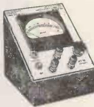
Ohmmeter for the rapid and direct measurement of very low values of resistance. Model R.M.155.
