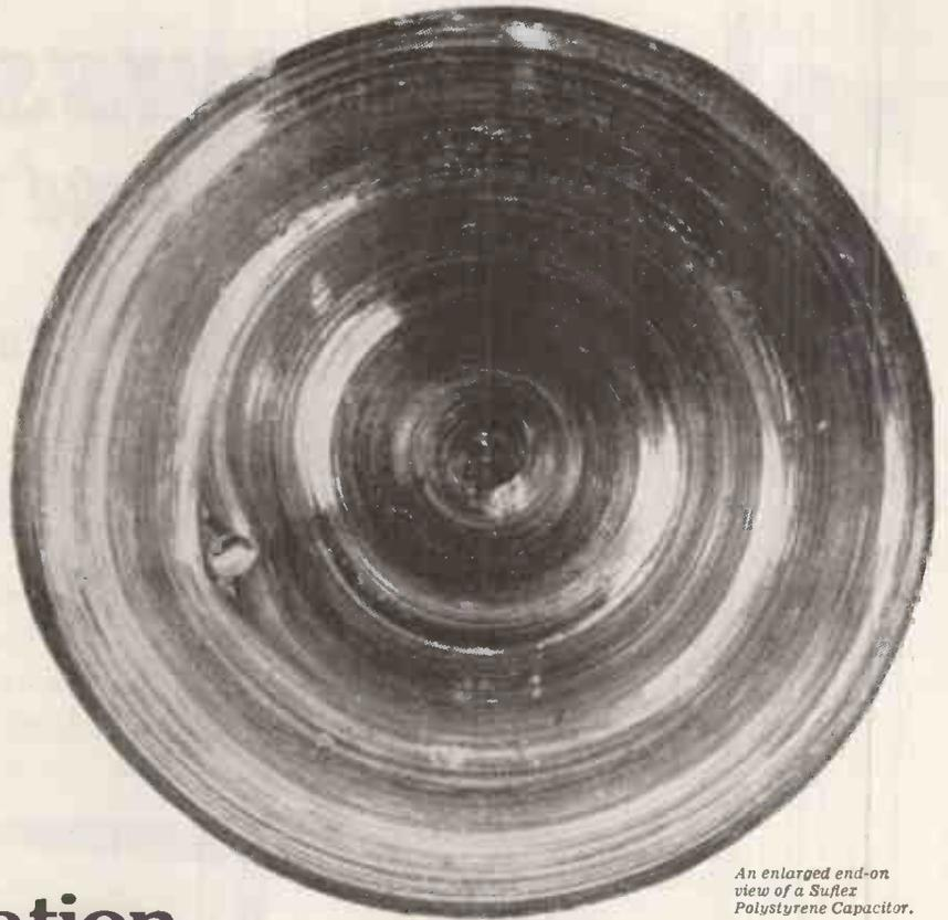
*An enlarged end-on view of a Suflex Polystyrene Capacitor.*
