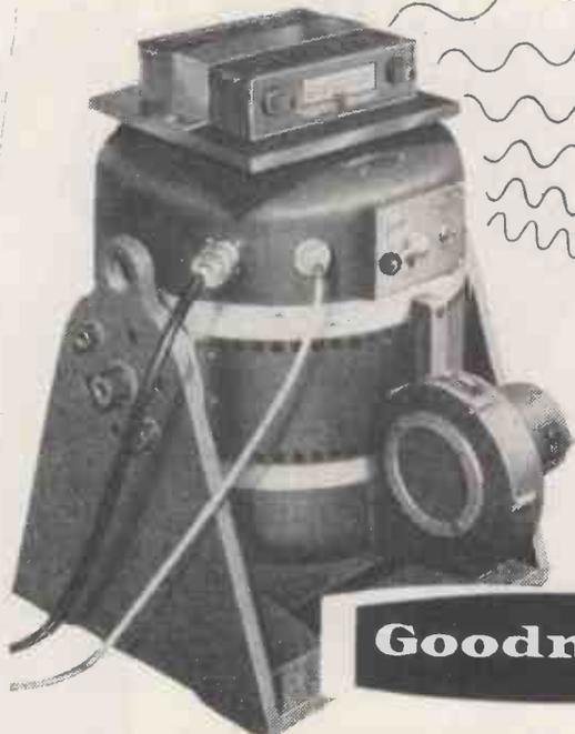
THAT is how a prototype car radio behaved when subjected to laboratory-simulated operating conditions on a Goodmans Vibration Generator. As a result of the test, modifications were made which now ensure long-life peak performance of every production model.
