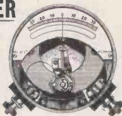
Apart from their normal use in Bridge circuits, etc., these instruments are ideal for conversion to Millivoltmeters for use in conjunction with Thermo-couples as Temperature Indicators.
