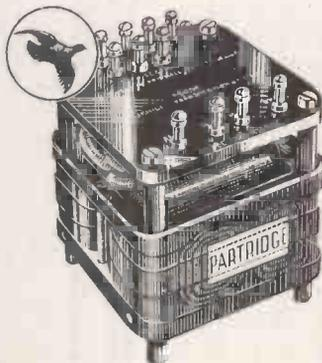
Optimum conditions are obtained in the form of output stage used in this amplifier when about 40% of the primary winding of the output transformer is common to anode and screen grid circuits. The Partridge Type P.3878 is of C-core design with windings of 43% of primary turns, and is specified by the designer for this amplifier.
