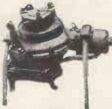
contain selsyn transmitter/receivers and it is these that provide the impulses which cause the aerial to rotate backwards or forwards. The equipment intended for 117 volt A.C. mains but will operate from our mains if connected through step down transformer of 1 K.W. rating.
