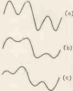
Fig. 6. In order to preserve the waveform of (a) + (b) when (a) is phase-shifted, the phase of (b) must be shifted twice as much.
