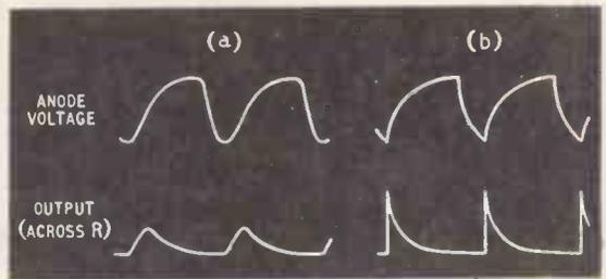
Fig. 5. Actual waveforms obtained in a circuit of the Fig. 3 type (with rectifier added to remove negative pulses), with (a) small and (b) large input signal amplitudes. Despite the very different peak values and shapes of the output pulses, they are equivalent, thanks to the principle illustrated in Fig. 2. The output pulses at (b) are very close to the theoretical shape—*c* in Fig. 4.
