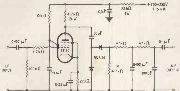
Above:—Fig. 9. Recommended circuit of limiter and discriminator.
