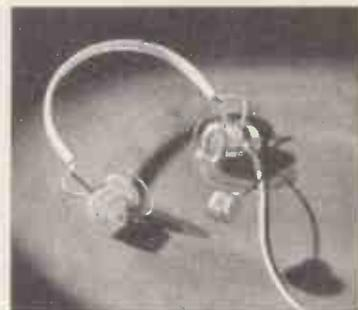
Flexibly mounted Perspex ear discs are a feature of the Amplivox lightweight headphone/microphone sets.
