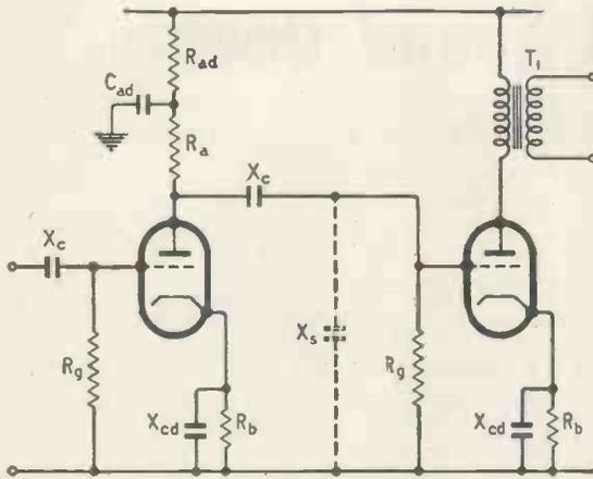
Fig. 3. Elementary amplifier showing sources of phase shift.
