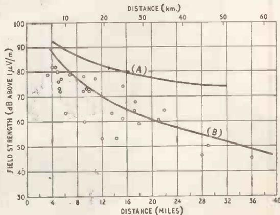
Measured field strength along four radials from transmitter KPTV at Portland, U.S.A.
