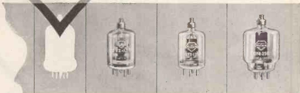
This new tetrode, the QY3-65, embodies a similar technique and construction to the Mullard range of all-glass transmitting valves which are already well established in communications and industry. It has an anode dissipation of 65 watts and a maximum frequency of 250 Mc/s and is directly interchangeable with the American 4-65A.
