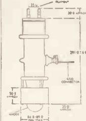
Triode Type CV 1098 this is a high-power air-cooled triode. Specification of which is as follows: Filament voltage 8.2 v., filament current 35 amps., anode dissipation 750 watts.
