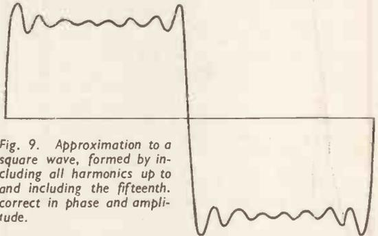
Fig. 9. Approximation to a square wave, formed by including all harmonics up to and including the fifteenth. correct in phase and amplitude.
