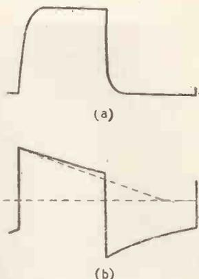
Fig. 11. Oscillograms of square waves distorted by the conditions shown in Fig. 10. Although Fig. 10(a) would suggest much worse distortion than (b), the relatively serious effect of phase-shift in (b) proves decisive.
