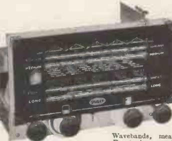
Incorporating the normal Long, Medium and Short wave bands, plus V.H.F. (Frequency Modulated) 87-101 mc/s. Latest miniature B.V.A. valves ECC85, ECH81, EF89, EABC80, EL84, EZ80, EM80. High Q inductances used throughout—Ferrite rods, for Medium and Long Waves Overall dimensions: Length 12in., Depth 1 1/2in. x 5 1/2in. including knobs and including knobs, 9 1/2in. Height 7 1/2in. Dial, which is multi-coloured on black background, has indicators for tone control and
