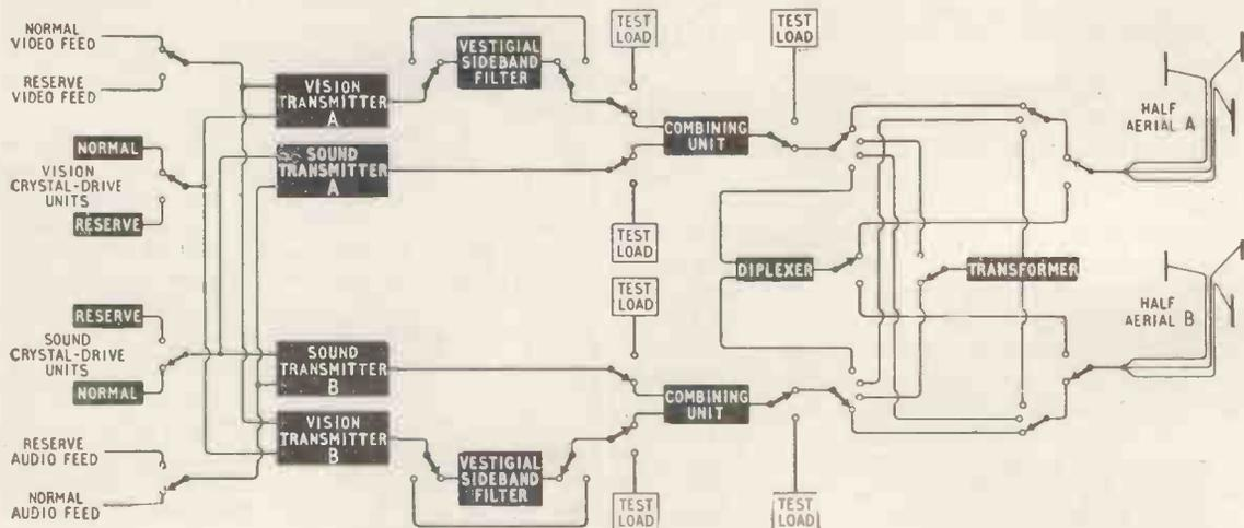
sections to be made. This is brought into action if the fault cannot be cured quickly, the idea being to permit a combination of transmitters and aerial sections that will give an output power reduced by only 3dB instead of 6dB. For example, both pairs of transmitters can be switched to either half of the aerial *via* the diplexer, or one pair of transmitters can feed both halves of the aerial *via* the transformer.
