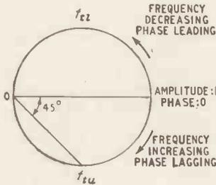
Fig. 4. The circle is the track of the tip of a vector hinged at O, representing signal voltage in a circuit where there is "single-order" cut-off at both high and low frequencies, as the frequency is varied. The vector  $O f_{tu}$  corresponds to the marked point at -3 dB in Fig. 2.
