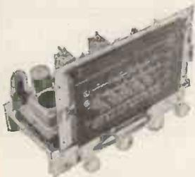
A 9-valve A.M./F.M. chassis with 4 wavebands (long, medium, short and F.M.), push-pull output stage and magic eye for precision tuning. Specially designed for permeability tuned F.M. stage and a very high degree of I.F. amplification for fringe area
