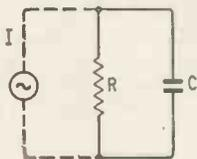
Fig. 1. The voltage set up across a resistance by a given signal current decreases with increasing frequency if there is a capacitance (intentional or otherwise) across it.
