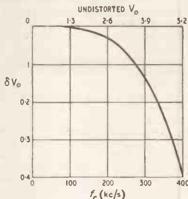
Right:—Fig. 11. Second-harmonic distortion due to non-linearity shown in Fig. 10, for 75 kc/s deviation, plotted against carrier frequency,  $f_c$ . All other harmonics are extremely small.
