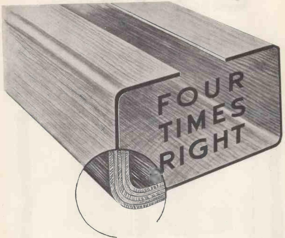
The SPEARS-LAMINA plywood shell has four complete right angles, pre-formed without cutting, steaming or stressing, and giving immense strength to the structure. The shell is made in thicknesses from 2 millimetres to 2 inches, radii from  $\frac{1}{2}$  in. upwards, dimensions from a few inches to 6 feet every way. Besides rectangles, any shape can be made which does not include a concavity. Minimum quantities are 10,000 of a pattern, and delivery at the rate of 500 to 5,000 per week.
