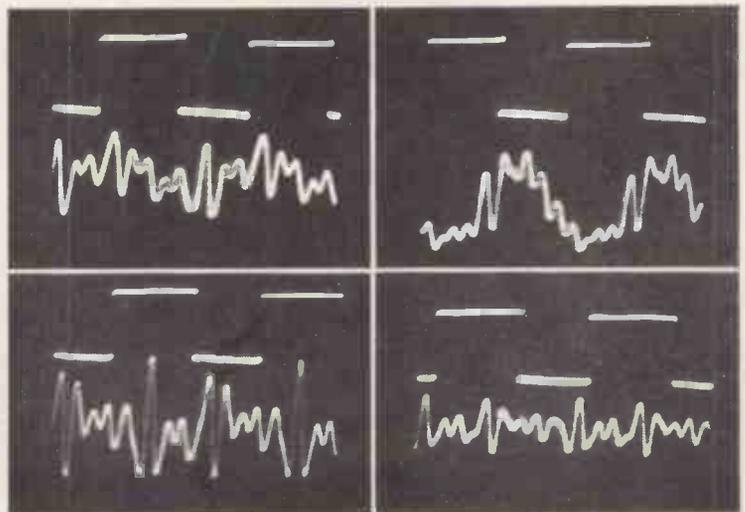
was to convert the waveform of Fig. 5(a) into that of Fig. 5(b) but even this drastic change could not be detected by any member of an experienced listening crew. The equipment has subsequently been used as a demonstration at several lectures, but to date, no listener has ever claimed to be able to detect the difference between the two waves.
