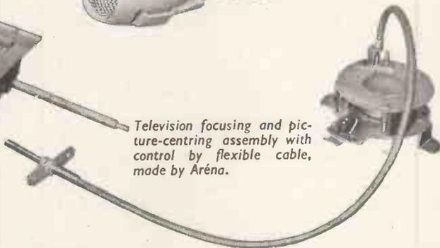
Television focusing and picture-centring assembly with control by flexible cable, made by Aréna.
