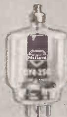
This new tetrode, the QY3-65, embodies a similar technique and construction to the Mullard range of all-glass transmitting valves which are already well established in communications and industry. It has an anode dissipation of 65 watts and a maximum frequency of 250 Mc/s and is directly interchangeable with the American 4-65A.
