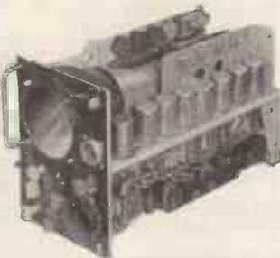
**MINIATURE I.F. STRIPS.** Size 10½in. x 10½in. x 3in., frequency 9.72 Mc/s, 2 EF.92's and 1 EF.91. I.F. amps. EB91, DET/AGC EF.91, AGC. Amp. and EF.91 limiter. Circuit supplied. Price less valves, 8/- each, post paid.
