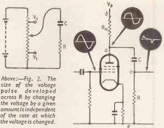
Above:—Fig. 2. The size of the voltage pulse developed across R by changing the voltage by a given amount is independent of the rate at which the voltage is changed.
