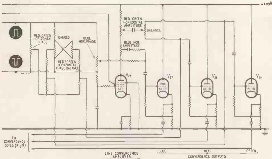
Fig. 11. Line convergence amplifier and output valves.
