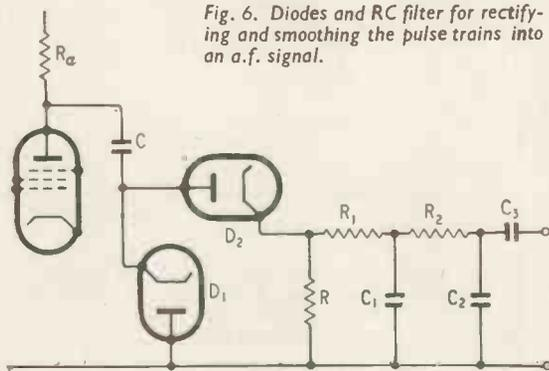
Fig. 6. Diodes and RC filter for rectifying and smoothing the pulse trains into an a.f. signal.
