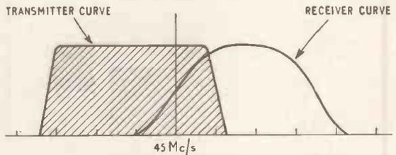
information sent by a vestigial sideband transmitter. The full line curve shows the reception capability of upper sideband receivers. The area under this receiver curve outside the shaded area represents what is described as the slight loss of detail. If such a "slight loss" occurred in apparatus for the B.B.C. instead of for the public, the B.B.C. would undoubtedly describe the loss of information as serious and unacceptable.
