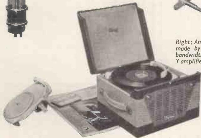
Left: A miniature gramophone turntable (45 r.p.m.) made by Edentzter. Right: The same equipment in a small portable record player by Clement, using a transistor amplifier (OC70, OC71 and two OC72s) and powered by four 1.5-V torch batteries. The size of the exhibits can be seen from the copy of our French contemporary, *Toute La Radio*, underneath.
