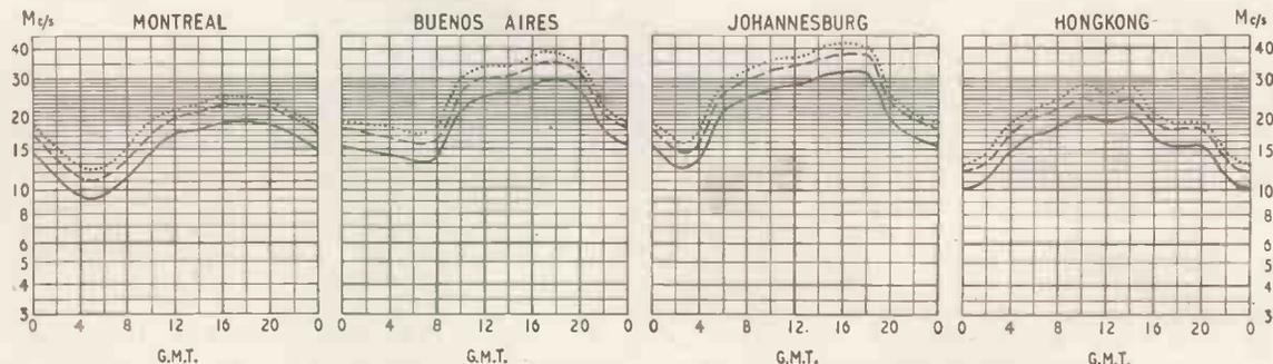
THE full-line curves given here indicate the highest frequencies likely to be usable at any time of the day or night for reliable communications over four long-distance paths from this country during April.
