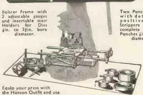
Equip your press with the Hunton Outfit and use inexpensive standardised Punches and Dies 1/2 in. to 3 1/2 in. diameter, obtainable from stock—in 1/2 in. sizes—when required.
