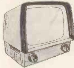
Complex curved sides, top and back in phenolic; chassis sits in virtually a plain wooden box with a fancy front. The moulding is used as a dust cover and holds the glass and mask, the glass being detachable via the wooden trim across the front. Plain colours, stoved enamel or the patented "Oxvar" finish could be used on the phenolic cover.
