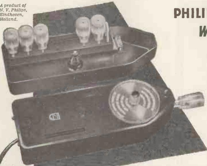
Seven plug-in coils give this useful new instrument a frequency range of 2.5-260 Mcs. Accuracy is better than 2%. A neon tube indicates resonance and there are also sockets for plugging in a head-set or valve voltmeter. Operated from 110v. or 220v. 50 c/s supply and weighing only 3 lb. the GM 3121 can also be used as a modulated or unmodulated test oscillator.
