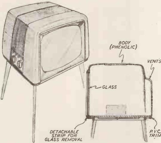
One-piece phenolic cover. Everything is there in one moulding: loudspeaker apertures, vented back, rabbit for glass with simple removal. Chassis, tube and controls mounted on plywood base. A separate centre pad in the tool could give variety in the speaker openings which could also be covered or painted to give colour changes. An extruded flexible p.v.c. trim provides a non-scratch, non-skid buffer for a polished table top and allows yet another possible colour change.
