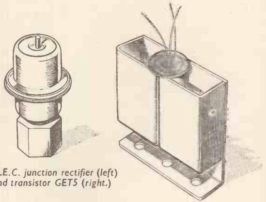
G.E.C. junction rectifier (left) and transistor GET5 (right.)
