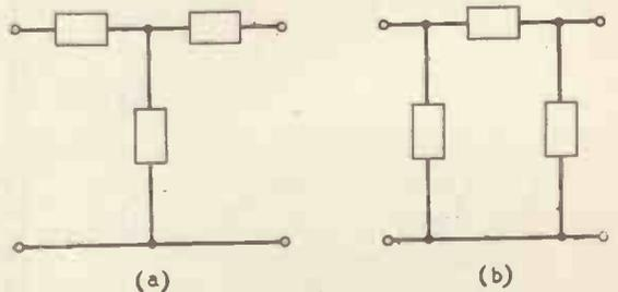
Fig. 2. These diagrams of the T (a) and  $\pi$  (b) networks are common in books on communication circuits, and of course are electrically the same as those in Fig. 1.
