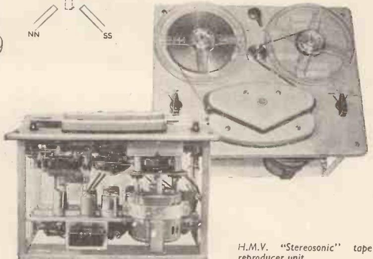
H.M.V. "Stereosonic" tape reproducer unit.
