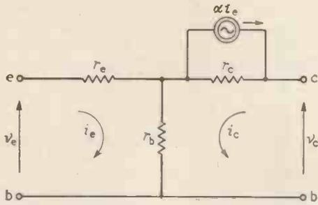
Fig. 1. Low frequency equivalent circuit.
