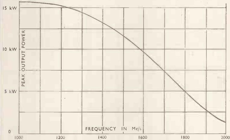
Also suitable for use as C.W. Oscillator or Amplifier giving outputs up to 15 Watts at frequencies up to 1000 Mc/s.
