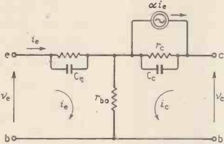
Fig. 2. High frequency equivalent circuit.
