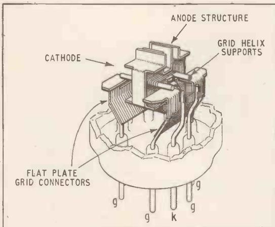
Electrode structure of Brimar 6AM4. The grid (normally earthed) is connected to five pins by flat metal sheets.
