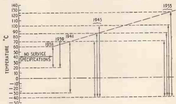
Above: Fig. 1. Increase in range of temperature specified for tests of Service equipment since 1938.
