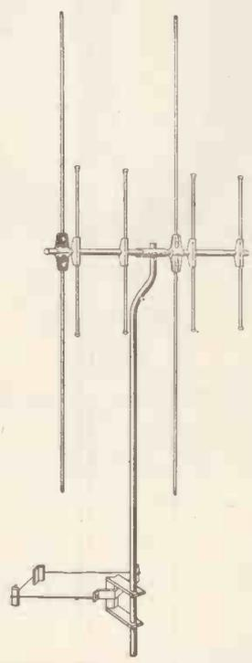
Band I "H" (Dipole and Director) Electronically coupled to 4 Band III elements for CHIMNEY MOUNTING. 17 HILO Models are available in all popular types of mounting, suitable for most areas, in any Band I|Band III channel combinations.
