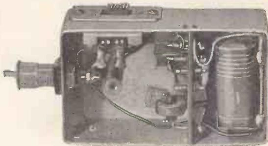
Fig. 2. Miniature crystal controlled transistor oscillator for testing v.h.f. mobile equipment (Labgear).
