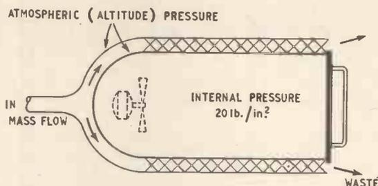
Fig. 4. Pressurized construction with annular heat exchanger.
