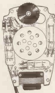
**THE COMPLETE KIT OF PARTS** includes a Type OL10 Hearing Aid (with Crystal microphone) in perfect working order with miniature earphone and moulded ear insert attached; ferrite rod, germanium diode, components, circuit diagram and full instructions.
