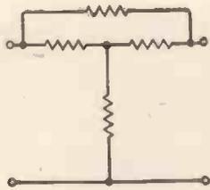
Left:—Fig. 8. This lattice circuit is just a different way of drawing the bridge—Fig. 7(a). Right:—Fig. 9. The bridged T is another network that can be simplified by the star-delta transformation.
