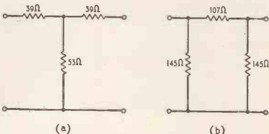
Fig. 4. These two attenuators are completely interchangeable.
