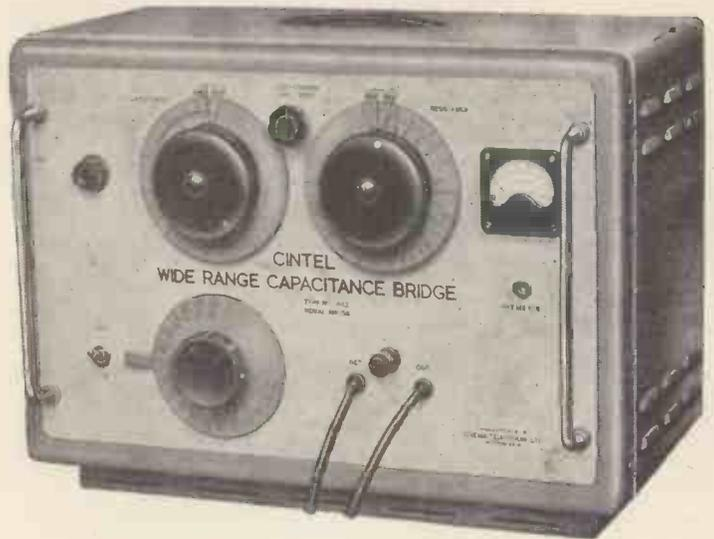
*Designed for the accurate measurement of capacitance and resistance in the range  $0.002\text{pF}$  to  $100\mu\text{F}$  and  $1\Omega$  to  $10,000\text{M}\Omega$  respectively.*
