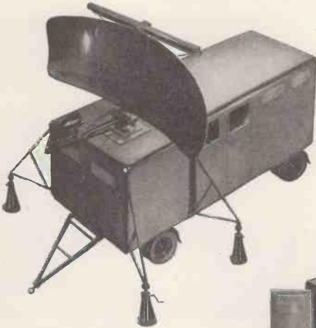
*The Aerial Head, jack-supported, is suitable for mobile, tower or roof mounting. A Secondary Radar aerial can be mounted on top of the scanner, as shown here.*
