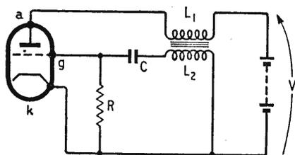
Fig. 1. Blocking oscillator circuit.
