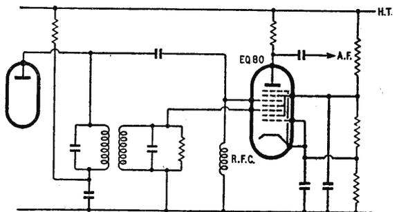
Fig. 3. Circuit for use with nonode discriminator.
