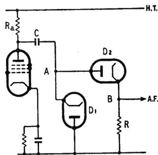
Right: Fig. 14. Basic "counter" circuit.
