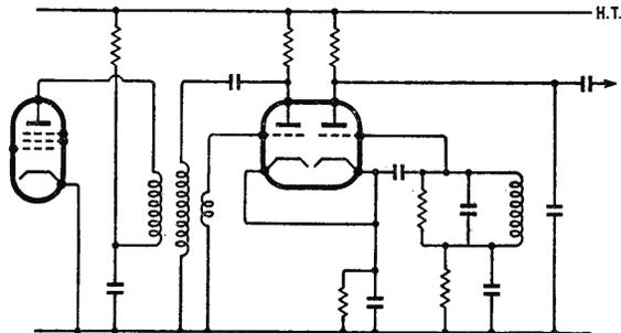
Above: Fig. 13. Practical circuit of synchro-trotor preceded by locked-oscillator limiter.
