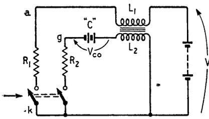
Fig. 6. The blocking oscillator circuit (Fig. 1) can be simulated quite well during its trigger phase by this working model, in which the valve is represented by  $R_1$ ,  $R_2$  and the two-pole switch.
