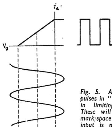
Fig. 5. Anode current pulses in "ideal" valve in limiting condition. These will have unity mark/space ratio if the input is much greater than is shown here.
