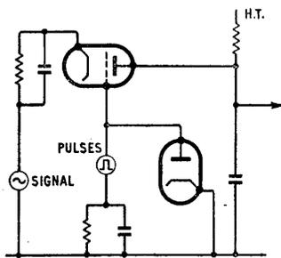
Above: Fig. 9. Basic circuit of the synchrotector.
