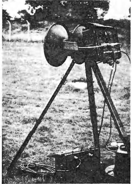
Marconi Type HP311 6.5-cm portable multi-channel communications equipment.
