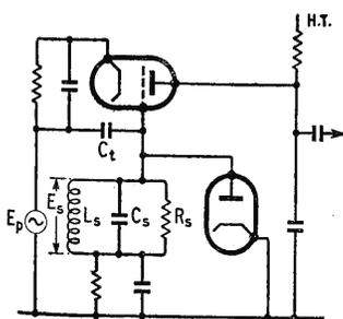
Left: Fig. 11. Circuit of synchro-trotor with sampling pulses derived from input signal.
