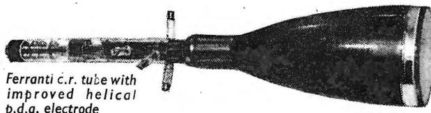
*Ferranti c.r. tube with improved helical p.d.a. electrode*
