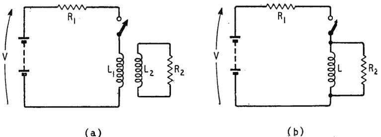
Fig. 5. The start of anode current is instantly followed by the start of grid current, converting Fig. 4 into this equivalent, shown in two forms.
