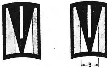
At balance, the breadth of the spot, B (right), gives some indication of the mean value of the two voltages. Actually the two deflecting electrodes form the anodes of two built-in triodes which serve to amplify the applied deflecting voltages. The tube can be operated entirely from an a.c. supply, and various other masks can be used for different applications. A full description appeared in Vol. 18, No. 8, of *Philips Technical Review*.
