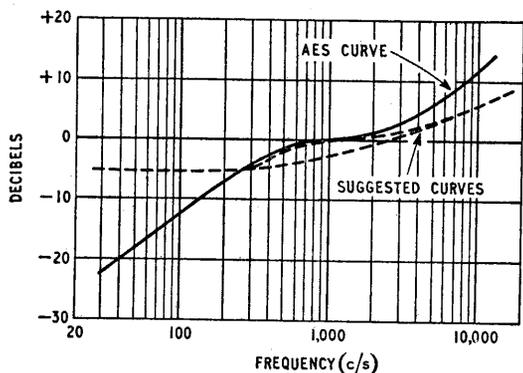
Fig. 7. Suggested revision of recording characteristics.
