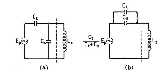
Below: Fig. 12. Thévenin's theorem applied to circuit (a) to give circuit (b).
