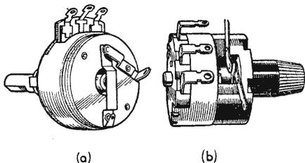
Potentiometers with press switch for flywheel sync circuits, (a) Welwyn "clutch" potentiometer and (b) A.B. Metal Products "Clarostat."
