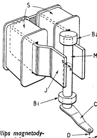
Philips magnetodynamic pickup.
