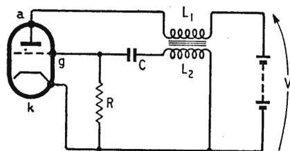
Fig. 1. Blocking oscillator circuit.
