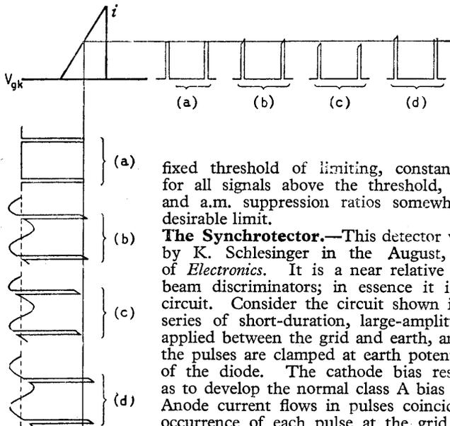
Right: Fig. 10. Showing how a.f. output from the synchrotector varies with phase angle between applied signal and sampling pulses; (a) no input signal (b) 90-degree phase shift (c) phase shift greater than 90 degrees (d) phase shift less than 90 degrees.
