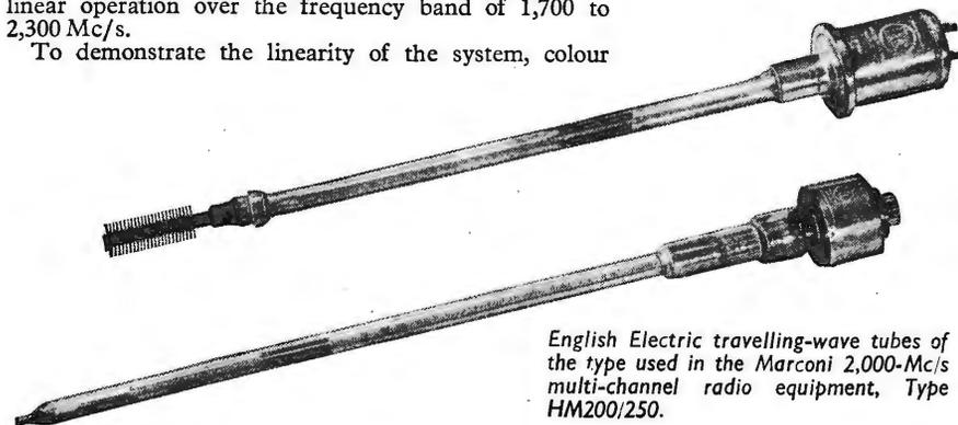
English Electric travelling-wave tubes of the type used in the Marconi 2,000-Mc/s multi-channel radio equipment, Type HM200/250.
