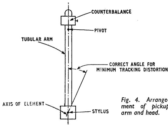
Fig. 4. Arrangement of pickup arm and head.
