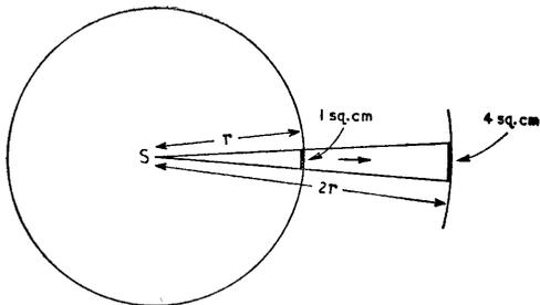
Fig. 2. S represents a source of sound, radiating equally in all directions. Knowing the total power radiated, one can easily calculate the intensity of sound at any distance from S. (It is assumed that there are no external obstructions.)
