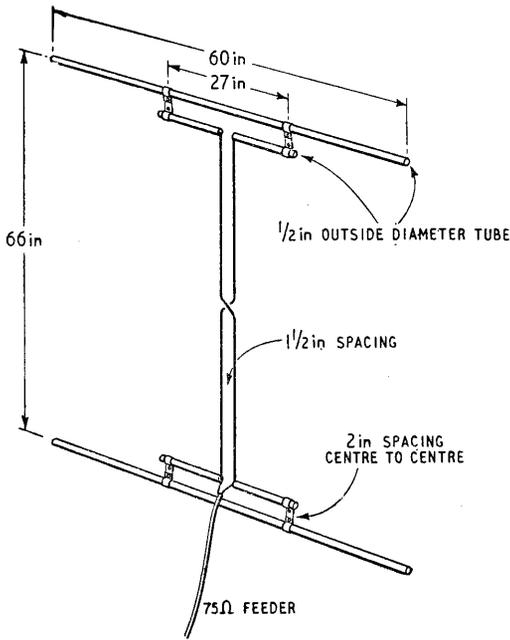
Fig. 7. Simple two-element stack using T-matched dipoles.
