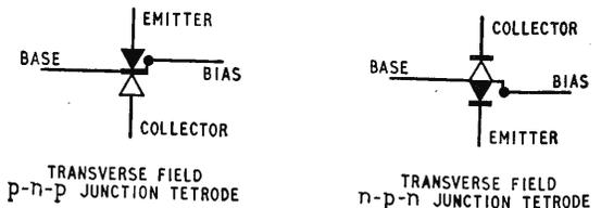
transistor with a second connection (the bias connection) to the base.
