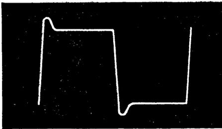
Fig. 4. Output for 5,000 c/s square wave input.
