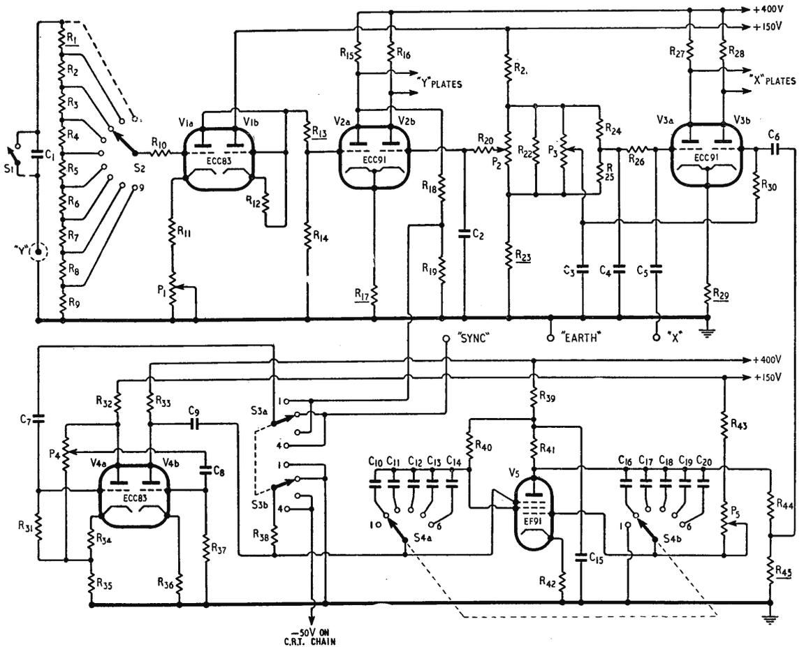
Fig. 3. Amplifier and time-base circuits.
