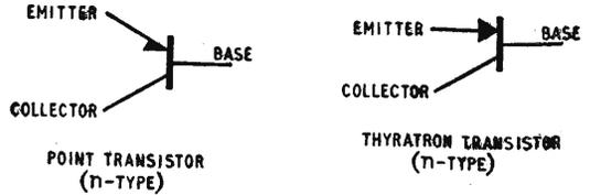
A thyatron transistor (above right), a transistor with a junction emitter and a point collector, is similar in characteristics to a point transistor.
