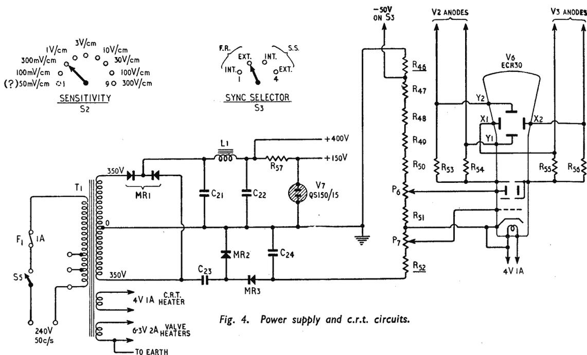
Fig. 4. Power supply and c.r.t. circuits.
