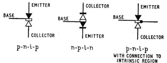
The *p*-*n*-*i*-*p* transistor may be regarded as an extreme case of the graded base *p*-*n*-*p* transistor, so a graded base transistor may be represented as above.
