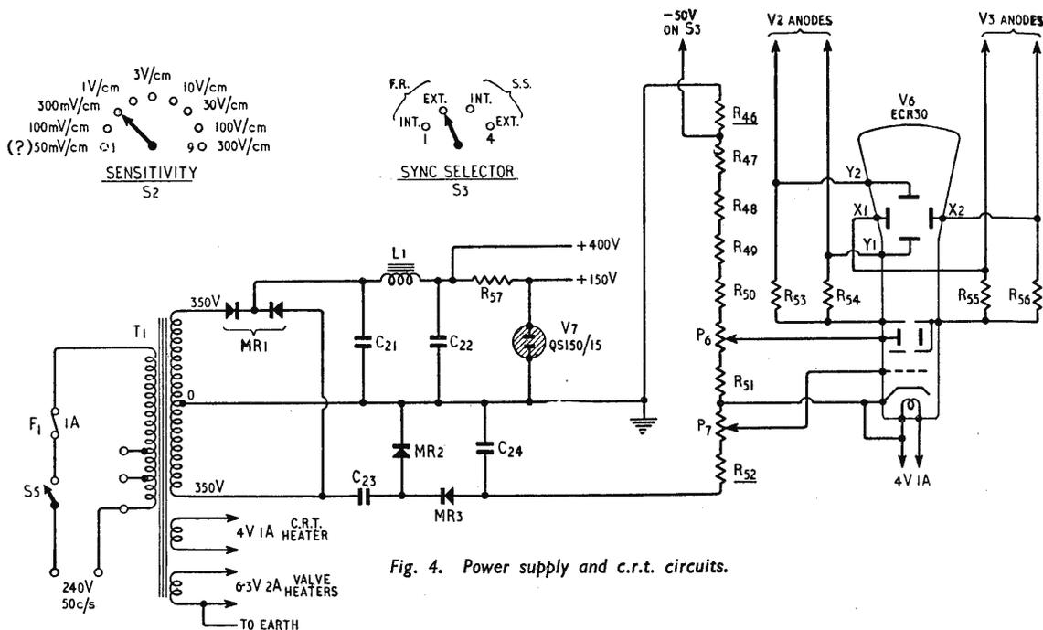
Fig. 4. Power supply and c.r.t. circuits.
