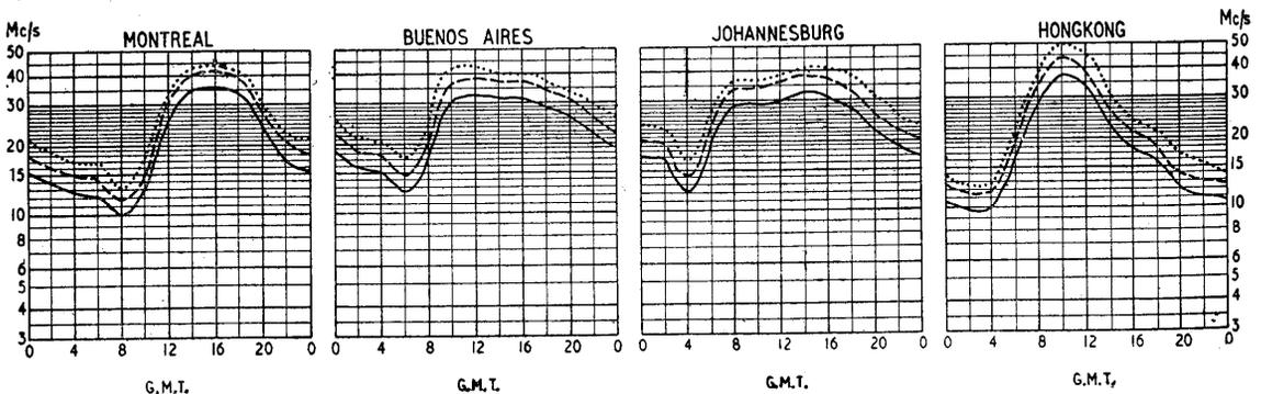
THE full curves given here indicate the highest frequencies likely to be usable at any time of the day or night for reliable communications over four long-distance paths from this country during November.
