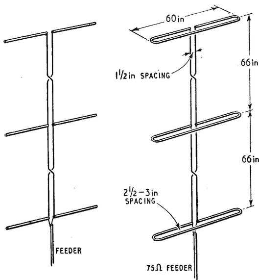
Fig. 5. Schematic arrangement of a stack of three half-wave dipoles.
