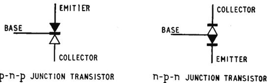
There are several types of junction triode referred to as alloyed, fused, surface barrier, grown, rate grown, diffused base, etc. Although all have their own particular characteristics they do not differ electrically sufficiently to warrant separate symbols. However, the *p*-*n*-*i*-*p* transistor has special properties, and the presence of an intrinsic layer in the base is shown by drawing the base as a narrow "box."
