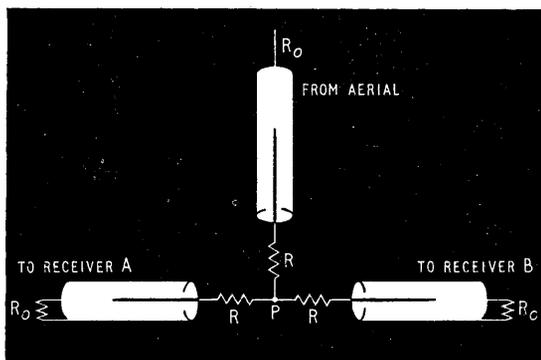
Fig. 1. A splitting network to avoid reflections.
