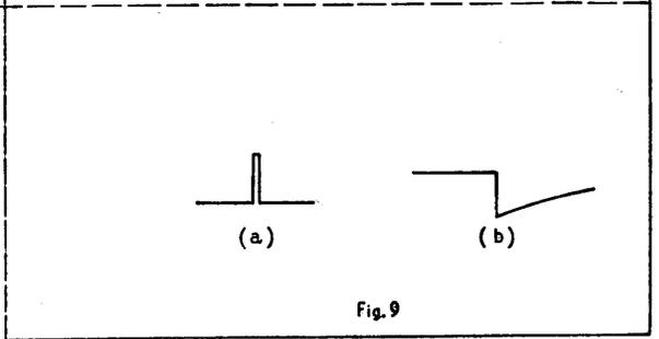
entiation is the first operation, using a critical time-constant RC network. The use of such a network is well known and forms the basis of a large group of sync separators. For the British system the maximum difference obtainable between line and frame pulses is 47% of the line pulse amplitude, and is produced with a time constant of 21.6 $\mu$ sec.
