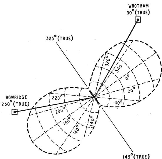
Fig. 4. The dipole's polar diagram superimposed on the plan, Fig. 1, as explained in the text.
