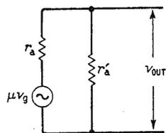
Fig. 2. Equivalent circuit of Fig. 1.
