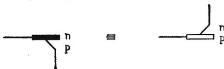
while in the Bell, R.C.A. and several other systems there is nothing about the way in which the junction is drawn which indicates which side is *p*, and which is *n*. This depends on whether the transistor is p-n-p or n-p-n.
