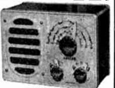
Consists of a 4 valve Superhet Receiver covering Medium Waveband 187-575 metres, and two Short Wavebands 15.6 to 136 metres. The new low consumption valves are incorporated and the whole is accommodated in an attractive robustly made case. Battery required is 90 volts and 1.4 volts (price 19/8) and is external to case.
