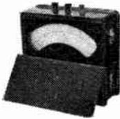
Brand new and boxed instruments by famous manufacturer housed in polished teak case. Moving iron movement reading A.C. or D.C. volts on 2 ranges. 0-160 and 0-320 volts. 8 in. mirror scale. Accuracy within 2%.
