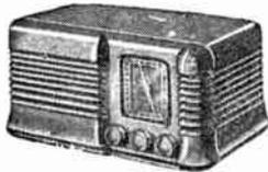
A design of a 3 valve 200-250 v. A.C. Mains L. & M. wave T.R.F. receiver with selenium rectifier. For inclusion in cabinet illustrated or walnut veneered type.
