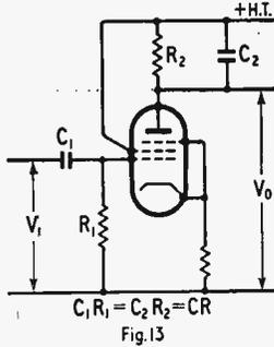
Fig. 13 Pentode isolated circuit.
