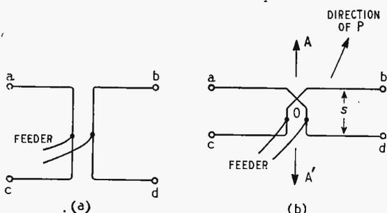
Fig. 11. With a broadside array (a) elements *ab*, *cd* are fed in phase. Maximum radiation takes place in direction at right angles to plane of the paper. "End-fire" array (b) is of the "8JK" type and elements are fed anti-phase and maximum radiation is in directions *OA*, *OA'*.
