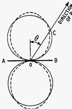
Fig. 4. Field-strength pattern of dipoles. The relative fields at P, when this point is moved round the dipole at constant range, is given by the length OC. With  $\lambda/2$  dipoles the pattern consists of two circles, or near circles (broken line)
