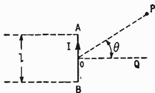
Fig. 1. Current  $I$  flowing in wire  $AB$  of length  $l$  produces field at  $P$  which is proportional to  $l \cos \theta$ .  $AB$  is assumed small compared with a wavelength and  $OP$  is large compared with  $AB$ . Maximum radiation is in the direction  $OQ$  at right angles to  $AB$ .
