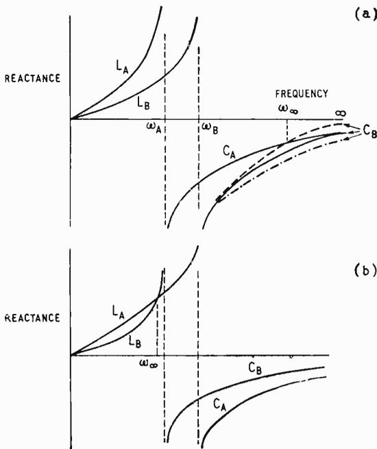
Fig. 11 Reactance diagrams for the generalized form of the lattice in Fig. 10.
