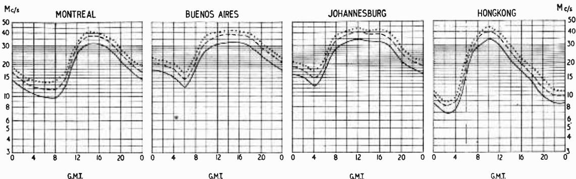
THE full curves given here indicate the highest frequencies likely to be usable at any time of the day or night for reliable communications over four long-distance paths from this country during February.
