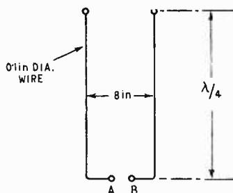
Fig. 9. Typical resonant line ( $Z_o = 600\Omega$ ). If length is changed by a small fraction  $b$  of a wavelength, or the frequency by  $4b \times 100\%$  a reactance  $2\pi b \times Z_o$  appears at AB.
