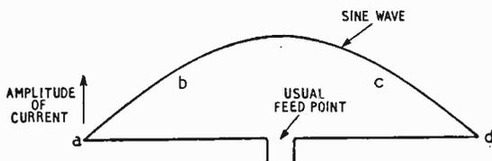
Fig. 2. Approximate current distribution in half-wave dipole. With shortened dipole (as Fig. 7) the portion  $bc$  of the sine wave occurs in the feeder and the remaining portions  $ab$ ,  $cd$  form a nearly-triangular distribution.
