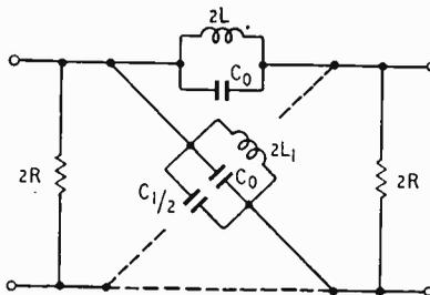
Fig. 10 Using the equivalence of Fig. 5,  $C_0$  is brought from the ends into the lattice itself.
