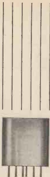
Our new Series 335 sub-miniature relay (shown here actual size) is very reliable and produces remarkably high contact pressures. Weight: Approximately  $\frac{1}{3}$  oz. Contact arrangement: D.P.C.O. Contact rating: 2A resistive load at 30V. D.C. or 115V. A.C. Nominal coil voltages: 6, 12, 24 & 48V. D.C. Max. continuous coil rating:  $1\frac{1}{2}$ W. Dimensions: 0.80" wide by 0.34" thick by 1" high, including pins. Max. coil resistance: 5000 $\Omega$ .
