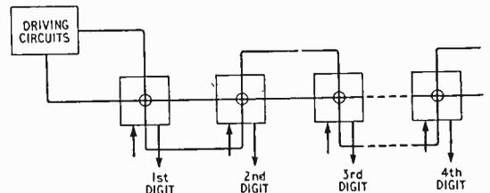
Fig. 6. Arrangement of matrix storage planes to give simultaneous access to all digits of a number.
