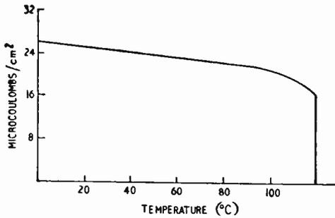
Fig. 3. Spontaneous polarization in a single domain of barium titanate, in microcoulombs per cm<sup>2</sup>.
