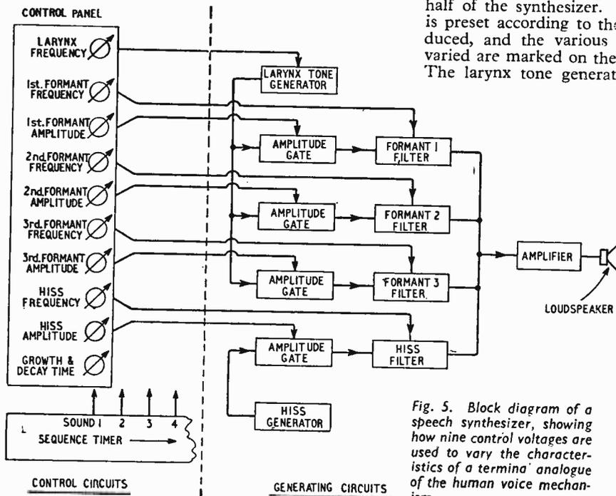
Fig. 5. Block diagram of a speech synthesizer, showing how nine control voltages are used to vary the characteristics of a terminal analogue of the human voice mechanism.
