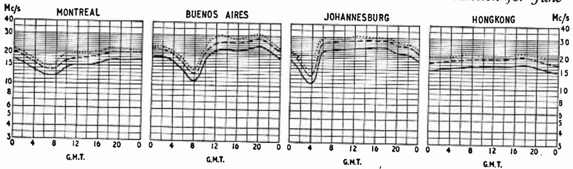
THE full-line curves indicate the highest frequencies likely to be usable at any time of the day or night for reliable communications over four long-distance paths from this country during June.
