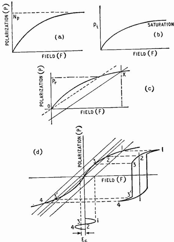
Fig. 2. Polarization and field curves. In Fig. 2 (a),  $P = Np \left( \coth \frac{pF}{kT} - \frac{kT}{pF} \right)$  for free dipoles; near 0, this is  $P \approx Np \left( \frac{pF}{3kT} \right)$ .  $k = 1.381 \cdot 10^{-16}$  erg/deg.
