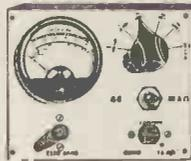
Comprising 2in. moving coil meter, scale calibrated in A.C./D.C. volts, ohms and milliamperes. Voltage range A.C./D.C. 0-50, 0-100, 0-250, 0-500. Milliamperes 0-10, 0-100. Ohms range, 0-10,000. Front panel, range switch, wire-wound pot for ohms zero setting, toggle switch, resistors and rectifier. Basic movement, 2 mA. In grey hammer finish case.
