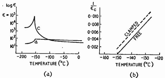
Fig. 4. Dielectric constants of potassium dihydrogen phosphate (divide e.s.u. by 900,000 to get μF.cm<sup>-1</sup>). The c direction is the ferroelectric axis.
