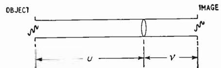
Putting  $u$  and  $v$  as positive distances, for a double convex lens
