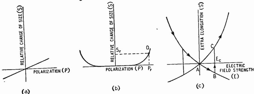
Fig. 6. Piezoelectricity in ferroelectrics.
