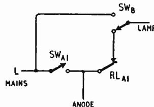
$SW_B$  having a changeover set connected as shown in the diagram.
