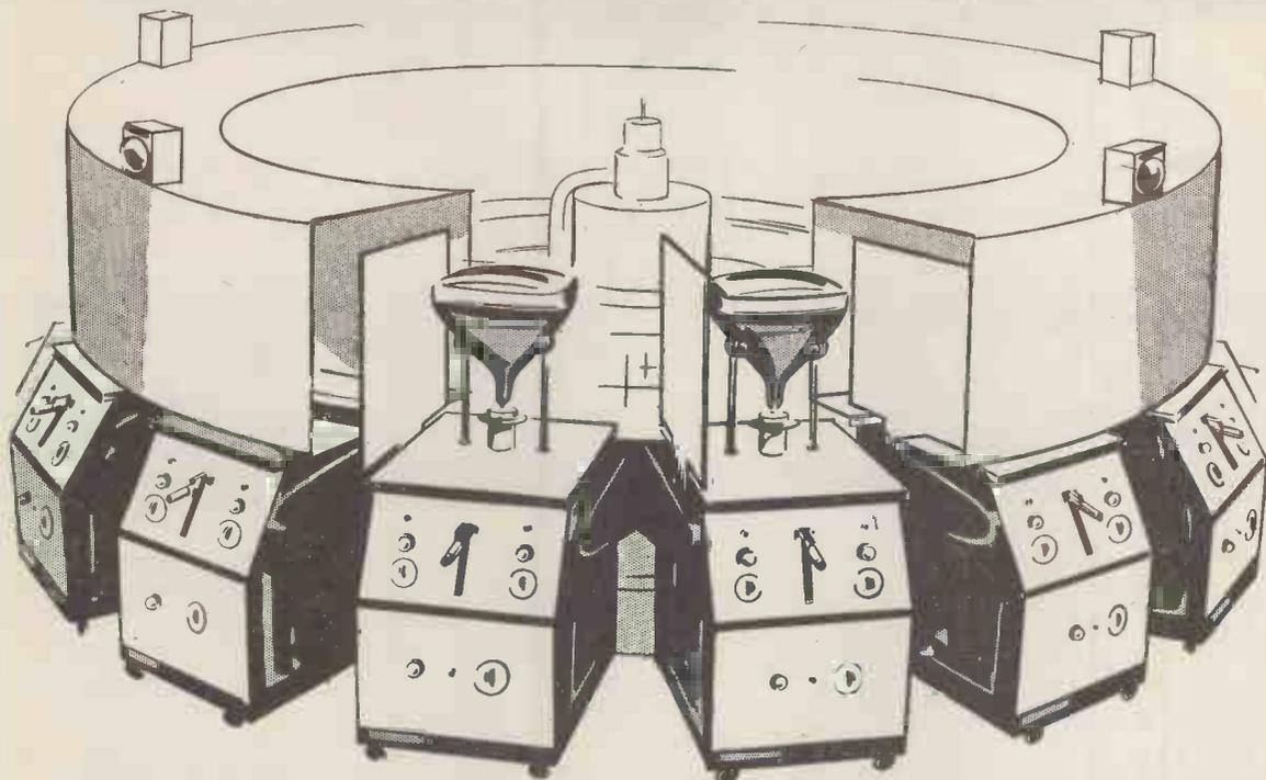
The most modern Pumping Unit manufactured. Can be used singly, 3-position automatic straight line, multi-stage rotary from 6-positions upwards, as shown.
