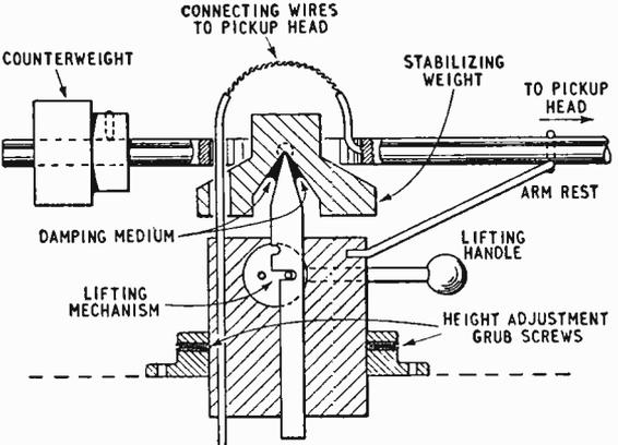
Fig. 4 Side-view sectional sketch of part of prototype arm showing stabilizing weight, damping medium, connecting wires and lifting mechanism.
