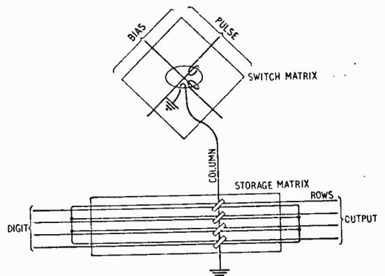
Fig. 7. Word address system with switch matrix.
