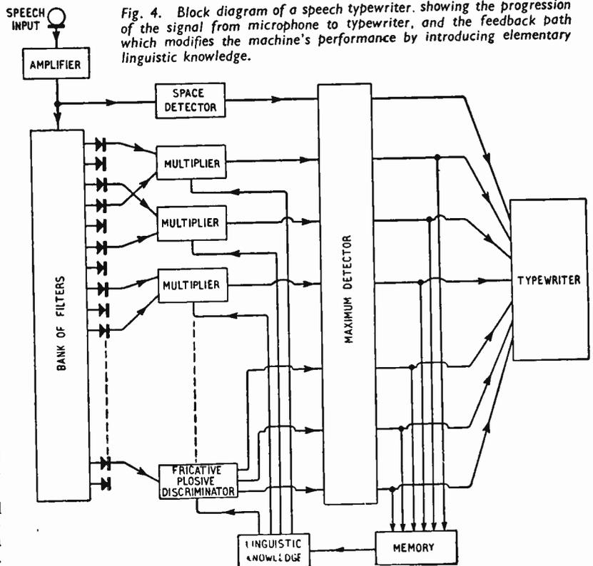
Fig. 4. Block diagram of a speech typewriter, showing the progression of the signal from microphone to typewriter, and the feedback path which modifies the machine's performance by introducing elementary linguistic knowledge.
