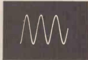
Waveform of output at 30 c/s with 4 watts input
