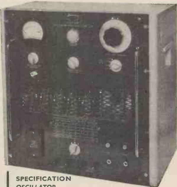
The High Power Oscillator/Amplifier is an instrument which combines an L.F. oscillator operating over the frequency range 30 c/s to 30 kc/s with a power amplifier capable of delivering up to 150 watts into a wide range of output impedances. The amplifier output is monitored by means of a built-in Voltmeter and an input socket is provided for use with external signal sources (microphones, pick-ups, signal generators, etc.).
