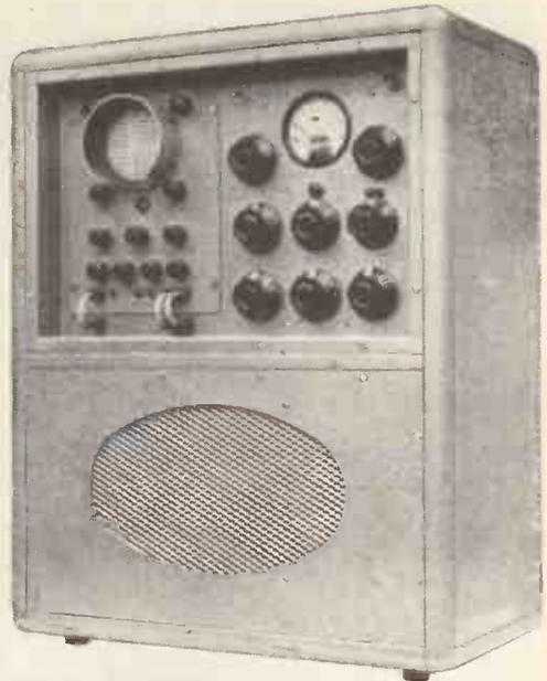
Appearance of multipath-propagation test-set developed by the B.B.C. Loudspeaker and a.f. amplifier are fitted to enable use as high-grade demonstration receiver.
