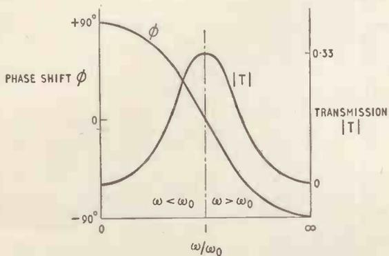
Fig. 3. Normalized transmission modulus and phase shift of a symmetrical Wien network plotted against  $\omega/\omega_0$ .
