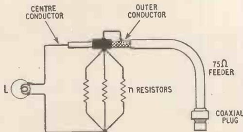
Fig. 2. Theoretical circuit of the dummy aerial.
