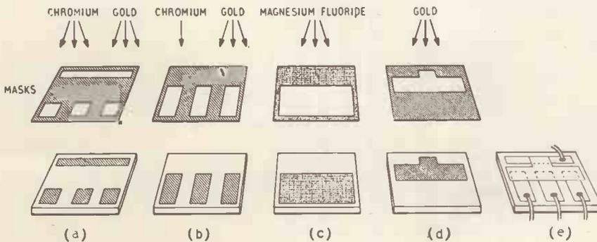
Fig. 3. Stages in production of gold-electrode, magnesium-fluoride-dielectric capacitors. (a) Chromium and gold terminals are applied by evaporation. (b) Gold electrodes are applied over chromium layer to give adhesion to substrate. (c) Magnesium-fluoride dielectric is applied and annealed at 300°C for 30 minutes. (d) Common electrode is applied to form (e) three-capacitor block.
