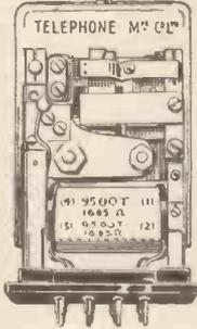
**NEW CENTER'S TYPE POLARISED RELAYS.** 2 x 9,500 turns at 1,685 ohms. Price 22/6 each. P. & P. 1/-
