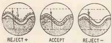
and again this is used to reject the part. The contour lines on the screen of the c.r.t. are somewhat larger than the actual parts being checked, and an optical focusing system, between the screen and the parts, reduces the image of the lines to the required dimensions.
