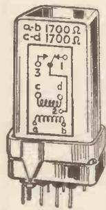
**SIEMENS H.S. RELAY.** Very latest type, sealed. H96E. 1,700 ohms plus 1,700 ohms, single C.O. contacts. Brand new with fixing clip. In maker's cartons. Price 16/6 each, plus 1/- P. & P.
