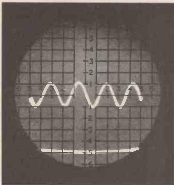
Fig. 2. Photograph of display showing one delayed signal of excess path length 8km, amplitude 20% of direct signal. The base line is recorded by a second exposure.
