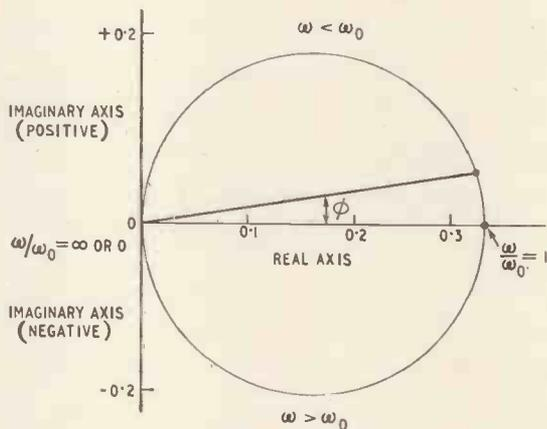
Fig. 2. Transmission of a symmetrical Wien network.
