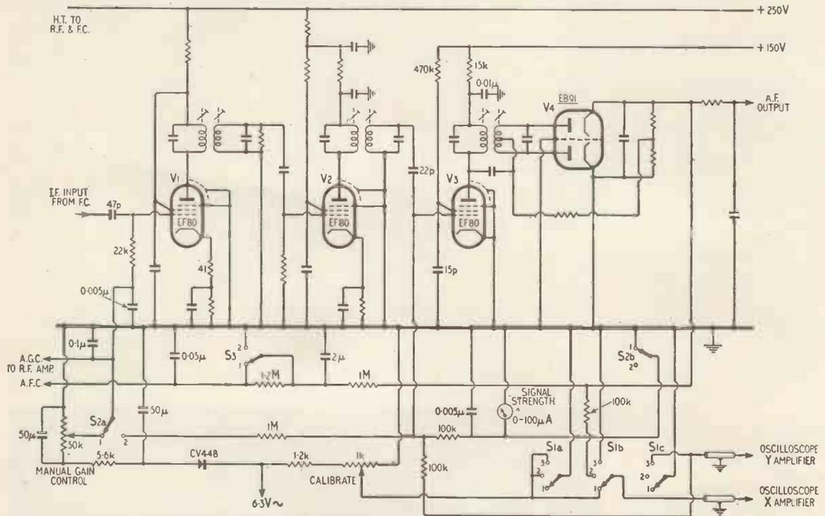
Fig. 5. Skeleton circuit diagram of modifications by B.B.C. to tuner to feed display-tube direct-coupled amplifiers. Switch functions and positions:—S1: position 1, "calibrate"; 2, "operate"; 3, "set zero"; S2: 1, "manual gain control"; 2, "a.g.c." S3: 1, "a.f.c. on"; 2, "a.f.c. off."
