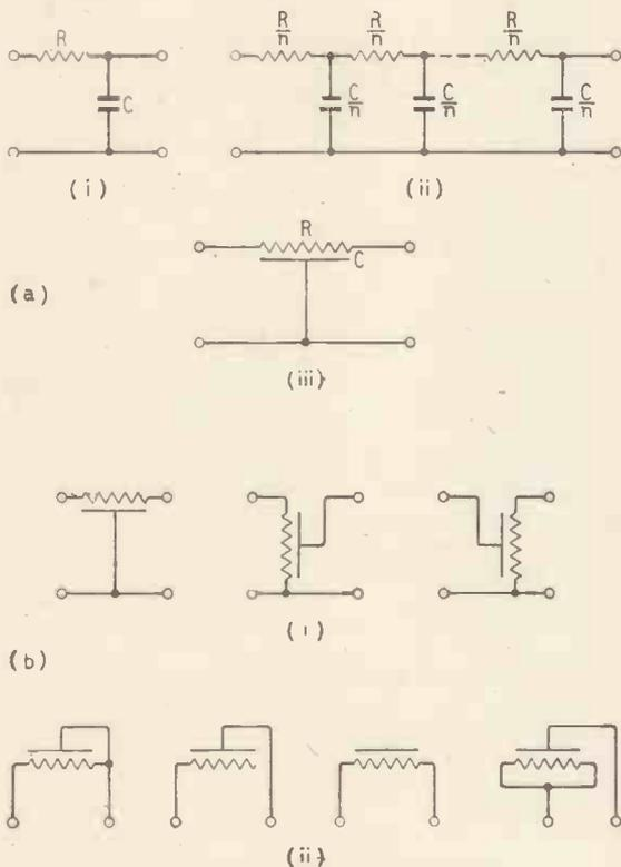
Fig. 4. (a) Evolution from (i) single R-C low-pass four terminal filter through (ii) multi-stage filter ("lumped constants") to (iii) distributed-constant type of low-pass filter. (b) Possible (i) four terminal and (ii) two terminal distributed R-C networks of the simplest type.
