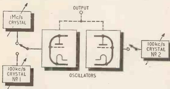
Fig. 1. One of two possible circuit arrangements for the frequency calibrator.
