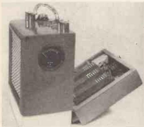
230 c/s, and the air volume in the box after the insertion of components was 26 cu in, which brought the peak up to 390 c/s. Allowing for losses in an attenuator and in the components which correct for variations of loudspeaker impedance with frequency, a maximum power of  $\frac{1}{4}$  W is needed from the transistor circuit.
