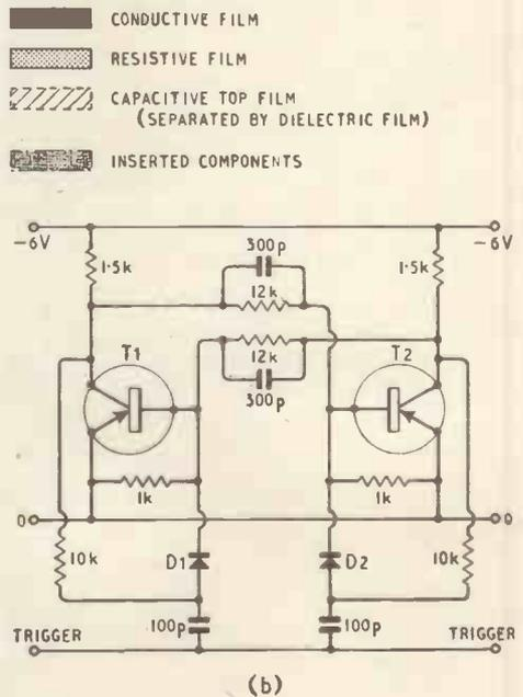
Fig. 1. Proposed layout (a) and (b) theoretical circuit diagram of binary-counter stage of flat-film form.
