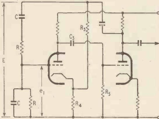
Fig. 5. Basic Wien bridge oscillator circuit.
