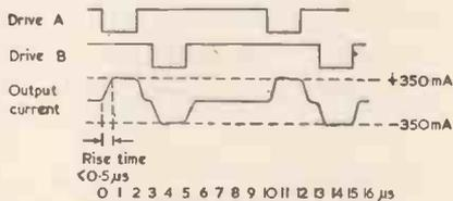
Pulse generator circuit for square loop ferrites
