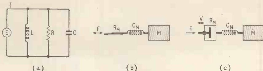
Olson's intriguing comparative diagrams. Anyway, using wholly c.g.s. units is better than the usual horrible mixture, in which various constants appear. Most of Olson's equations would be the same in m.k.s.
