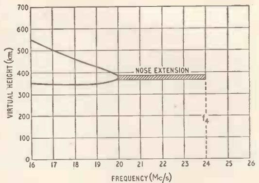
Fig. 3. Part of curve (b), Fig. 1, re-drawn and with a "nose extension" due to scattering and other processes, added for a 2,000-km transmission.
