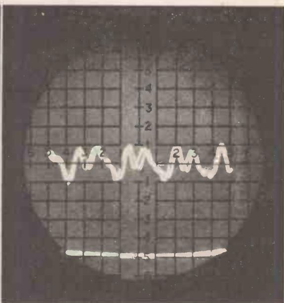
Fig. 3. Display given by complex signal with three delayed signals of path-length differences: 8km, 16km and 24km. Amplitude of each delayed signal is 10% of direct signal.
