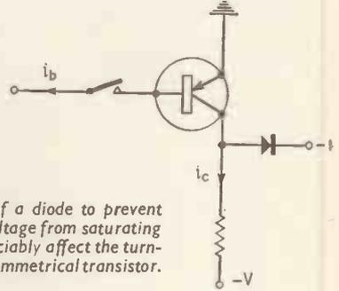
Fig. 4. Use of a diode to prevent the collector voltage from saturating does not appreciably affect the turn-off delay of a symmetrical transistor.
