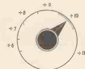
Fig. 4. Calibration of the multivibrator lock control,  $R_7$ .
