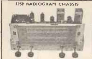
THREE WAVEBANDS S.W. 16 m.-50 m. M.W. 200 m.-550 m. L.W. 800 m.-2,000 m. 12 month Guarantee. A.C. 200/250 v., 4-way switch. Short-Medium-Long-Gram. A.V.C. and Negative Feedback, 4.2 watts. Chassis 13 1/2in. x 5 1/2in. x 2 1/2in. Glass Dial Size 10 x 4 1/2in. horizontal or vertical. 2 Pilot Lamps. Four Knobs. Walnut or Ivory, aligned and calibrated. Chassis isolated from mains.
