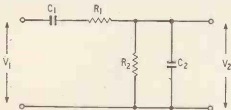
Fig. 1. Reactive section of Wien bridge.
