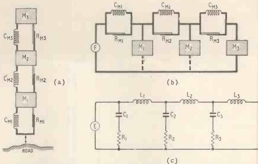
differently, we find ourselves with a parallel mechanical circuit as the analogue of a series electrical circuit.
