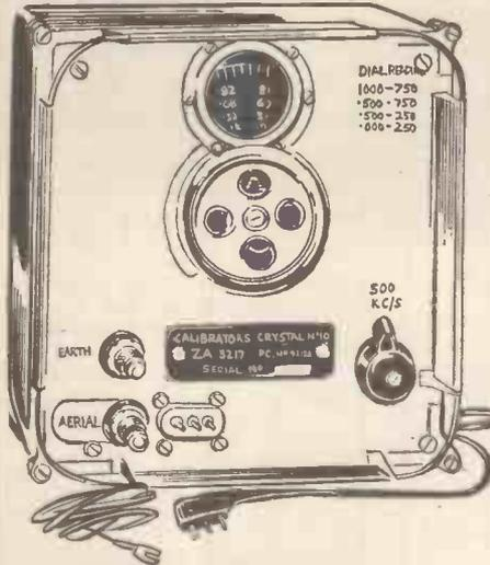
**CRYSTAL CALIBRATOR No. 10** crystal controlled 4-valve high-grade instrument in the same category as the famous B.C.221. Directly calibrated, does not require cross reference or charts—functions as follows:
