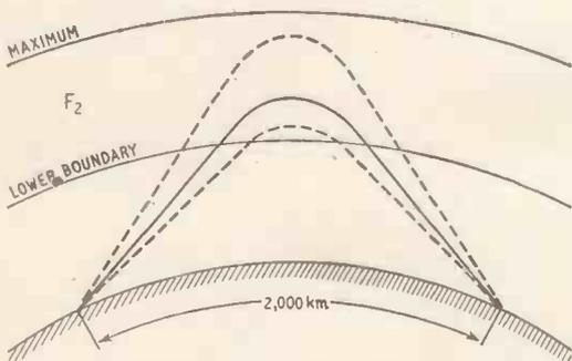
Fig. 2. Dashed-line curve shows high- and low-angle rays at 17 Mc/s; full-line curve a single ray at 20 Mc/s (see (b) Fig. 1).
