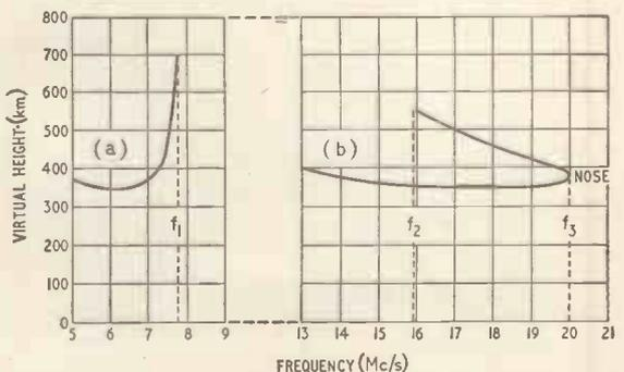
Fig. 1. Variation of virtual height with frequency ( $h'-f$ ),  $F_2$ -layer, ordinary wave only; (a) for vertical incidence; (b) for transmission over a distance of 2,000km.
