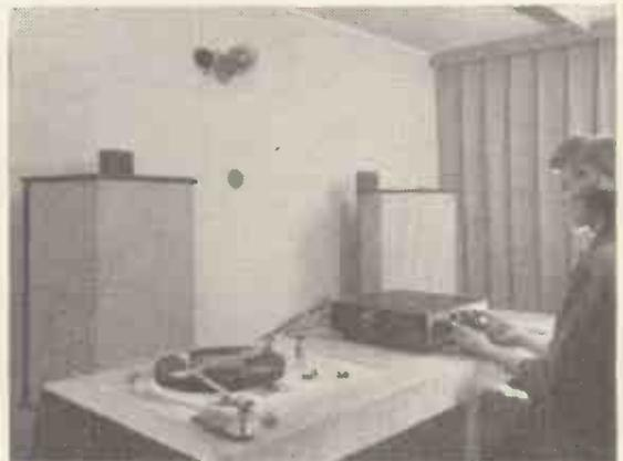
Over 50% of the production time of Beam-Echo (Avantic) equipment is devoted to testing. The photograph shows the final listening test on an SPA21 stereophonic combined pre-amplifier and 2 x 12-watt amplifier being performed in a near acoustically dead room.
