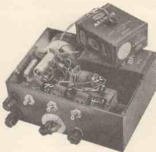
Another view of the calibrator with the l.t. battery withdrawn and showing position of the valves below  $L_1$ .
