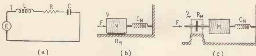
Fig. 1. Electrical series circuit (a) and mechanical equivalent according to (b) Olson and (c) Bloch.
