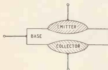
Fig. 1. Cross-section of a symmetrical transistor.
