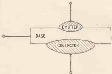
Fig. 6. Cross-section of a high-speed transistor.
