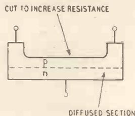
Fig. 5. (a) Appearance and (b) equivalent theoretical circuit of distributed-type element made by diffusion processes for solid-circuit techniques.
