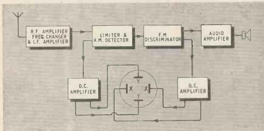
Fig. 1. Block-schematic diagram of equipment for test-set as arranged by B.B.C.
