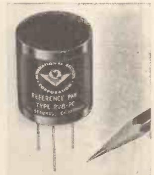
Miniature reference-voltage encapsulated unit for mounting on printed-circuit boards. (International Rectifier Co.)
