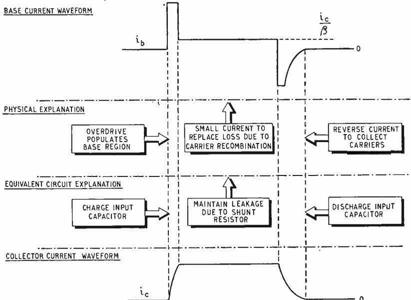
Fig. 5. Diagram to illustrate the accelerated switching of a transistor.
