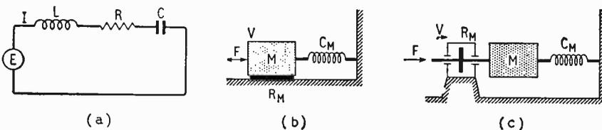
Fig. 1. Electrical series circuit (a) and mechanical equivalent according to (b) Olson and (c) Bloch.
