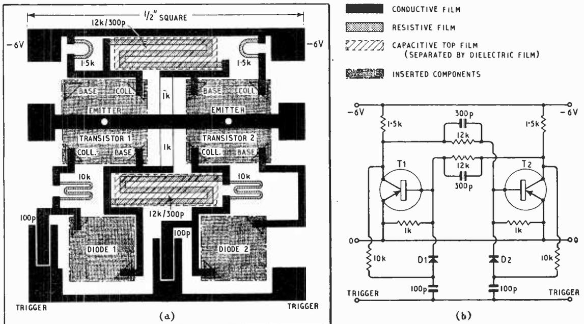
Fig. 1. Proposed layout (a) and (b) theoretical circuit diagram of binary-counter stage of flat-film form.
