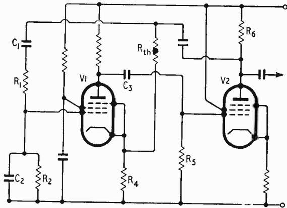
Fig. 7. Theoretical circuit diagram of Wien bridge oscillator used as basis for design procedure.
