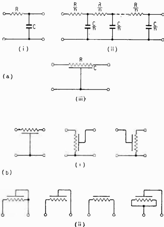
Fig. 4. (a) Evolution from (i) single R-C low-pass four terminal filter through (ii) multi-stage filter ("lumped constants") to (iii) distributed-constant type of low-pass filter. (b) Possible (i) four terminal and (ii) two terminal distributed R-C networks of the simplest type.
