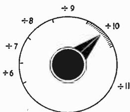
Fig. 4. Calibration of the multivibrator lock control,  $R_7$ .
