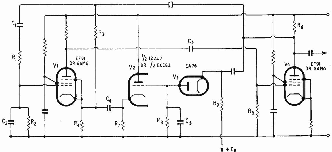
Fig. 6. Possible method of stabilizing the amplitude of a Wien bridge oscillator.
