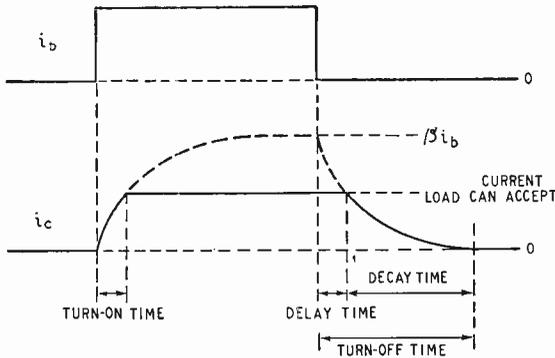
collector might be very different, as shown in Fig. 2 (d), and it is the total output charge which is  $\beta$  times the total input charge. This is consistent with the d.c.  $\beta$  of the transistor, as can be seen by regarding the base current as the succession of a lot of separate charges, then the collector current is this succession multiplied by  $\beta$ .
