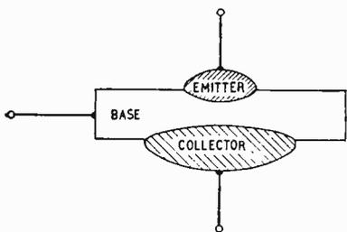
Fig. 6. Cross-section of a high-speed transistor.
