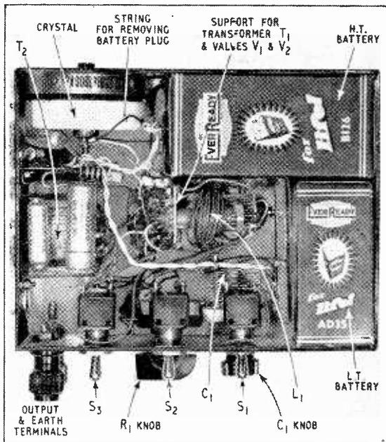
Plan view (with lid removed) of the crystal calibrator. Circuit identifications relate to Fig. 3.
