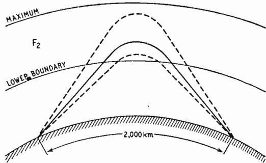
Fig. 2. Dashed-line curve shows high- and low-angle rays at 17Mc/s; full-line curve a single ray at 20Mc/s (see (b) Fig. 1).
