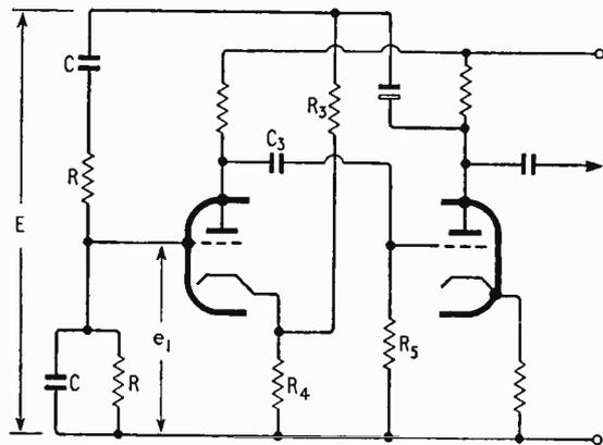
Fig. 5. Basic Wien bridge oscillator circuit.
