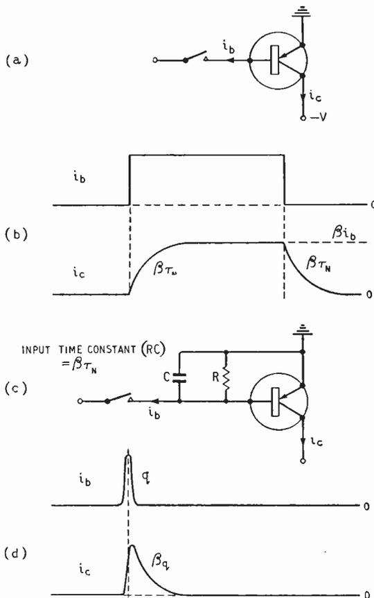
Fig. 2. Derivation of the charge concept in transistor switching: (a) transistor being switched by current pulse, (b) base and collector current waveforms, (c) equivalent circuit for producing the collector waveform, (d) base and collector current waveforms illustrating the charge concept.
