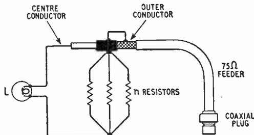
Fig. 2. Theoretical circuit of the dummy aerial.
