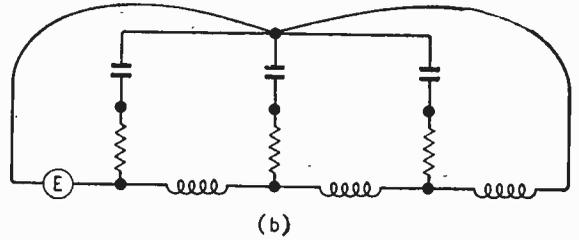
Fig. 6. For the sake of the weaker brethren the metamorphosis from Fig. 5(b) to (c) is here eased by intermediate stepping stones. At (a) the mechanical elements have been changed to electrical with the same (now incorrect) connections. Changing these over from series to parallel and vice versa, with the help of the black dots, we get (b), which in tidier layout is Fig. 5(c).
