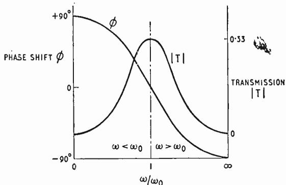
Fig. 3. Normalized transmission modulus and phase shift of a symmetrical Wien network plotted against  $\omega/\omega_0$ .
