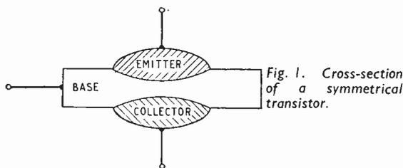
Fig. 1. Cross-section of a symmetrical transistor.
