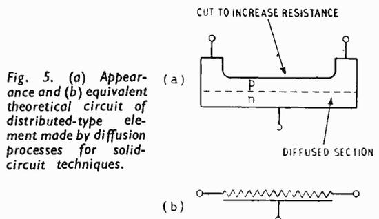
Fig. 5. (a) Appearance and (b) equivalent theoretical circuit of distributed-type element made by diffusion processes for solid-circuit techniques.
