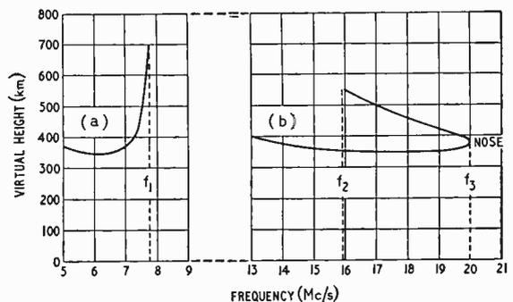
Fig. 1. Variation of virtual height with frequency ( $h'-f$ ),  $F_2$ -layer, ordinary wave only; (a) for vertical incidence; (b) for transmission over a distance of 2,000km.
