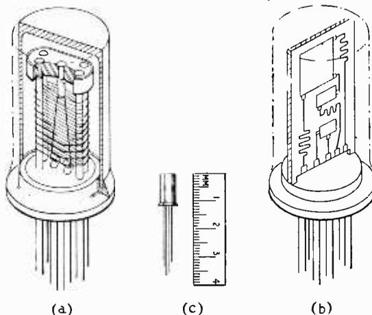
Fig. 6. Comparison of (a) micro-miniature thermionic valve with (b) component-assembly hermetically sealed in similar envelope; also shown (c) is size of envelope relative to scale calibrated in mm.
