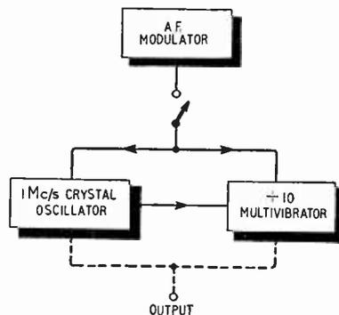
Fig. 2. The alternative circuit arrangement discussed in the text.
