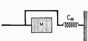
Fig. 3. The mass ( $M$ ) and compliance ( $C_M$ ) in Fig. 1 are not, as might be supposed, in series, but in parallel, as can be seen by re-drawing thus.
