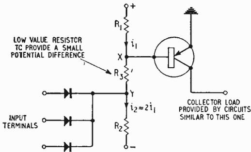
Fig. 8. Example of "low level logic" switching circuit.
