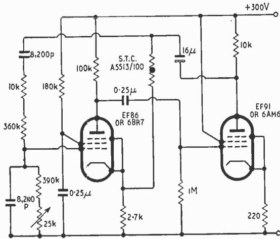
Fig. 8. Practical circuit of a thermister-stabilized Wien bridge oscillator.
