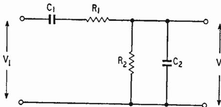
Fig. 1. Reactive section of Wien bridge.
