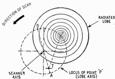
Fig. 2. Cross-section of a conical scan.
