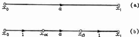
Fig. 5. Introducing test points in a signal-flow diagram.
