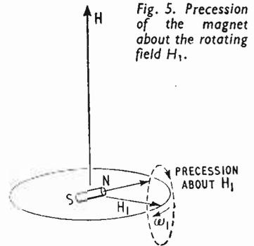
Fig. 5. Precession of the magnet about the rotating field  $H_1$ .
