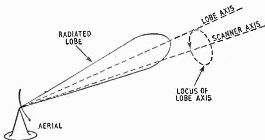
Fig. 1. Production of a conical scanning pattern.
