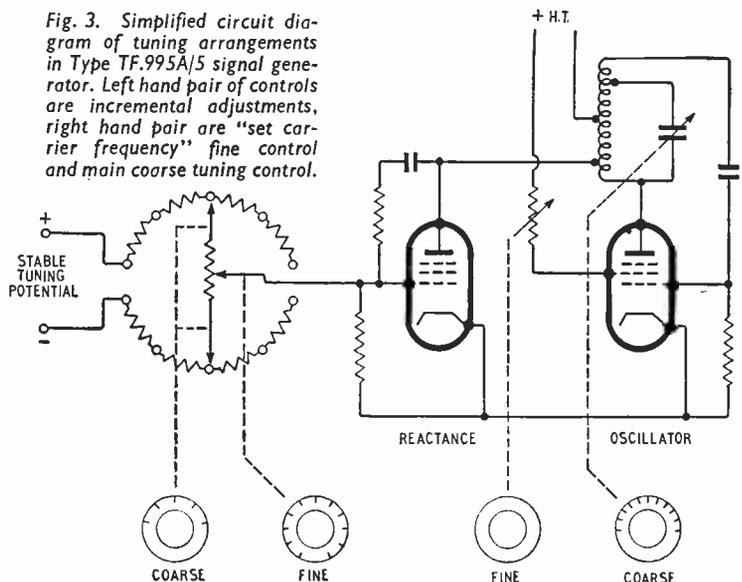
Fig. 3. Simplified circuit diagram of tuning arrangements in Type TF.995A/5 signal generator. Left hand pair of controls are incremental adjustments, right hand pair are "set carrier frequency" fine control and main coarse tuning control.
