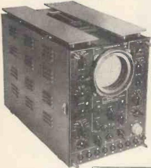
Made for the Ministry by leading manufacturers (e.g., Erskine & Hartley Electromotives) this fine instrument is suitable for the examination of waveforms from two cycles to ten megacycles. It is extremely well designed and incorporates such desirable features of construction as potted "C" core transformers and paper smoothing capacitors for complete reliability. No electrolytic condensers are used.
