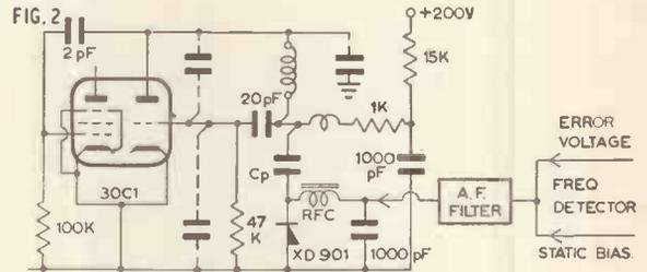
The diode series resistance  $r_s$ , which is not frequency sensitive, dissipates some available oscillator power. The grid circuit resistance of an oscillator is inherently low and to some extent this masks the damping effect that the diode series resistance may have on the circuit. But to ensure a low loss even at 250 Mc/s, the series resistance of the XD901 has been reduced to 5 ohms.
