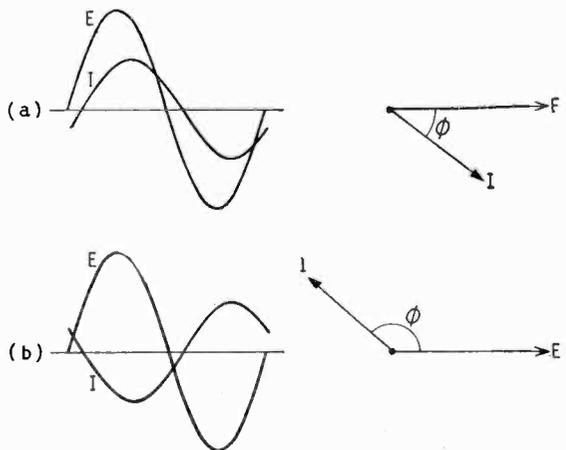
Fig. 6. Unless an a.c. is exactly in phase or antiphase with the e.m.f. there are parts of every cycle when it is flowing with and against the e.m.f., whichever way the net power flows.
