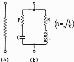
Fig. 1. (a) is a particular kind of impedance that is obviously independent of frequency. Though this is less obvious with (b), it too amounts to exactly the same thing.
