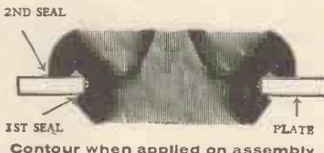
This grommet provides a thoroughly efficient seal. Around the panel hole the first seal is effected, while a good, tight second seal around the top periphery is set up by tension. In the grommets designed for cable entry the internal seal is applied within the conical section. All grommets can be fitted to various panel thicknesses—thus reducing the range.
