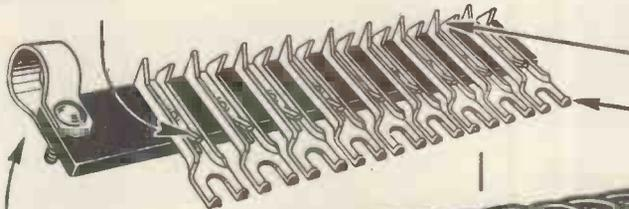
(c) Cable secured by crimping
