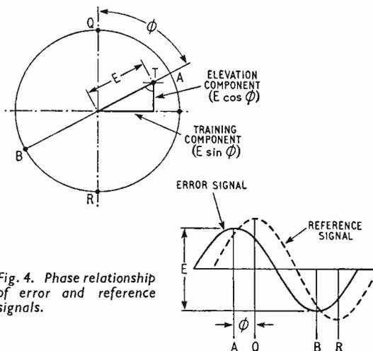
Fig. 4. Phase relationship of error and reference signals.
