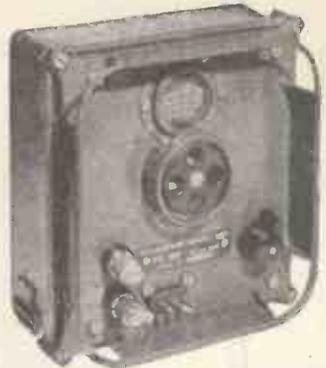
**BRAND NEW CRYSTAL CALIBRATOR No. 10**. (Battery powered 1.4 v. valves.) Complete with full working instructions, circuit diagram, carrying haversack, connecting lead and spare valves. Frequency range: 1.5 to 10 Mc/s. (Nominal) but can actually be used up to 30 Mc/s. Weight 5lb. Size 7in. x 7 1/2in. x 4in. A miniature B.C.221 in every respect. A must for every laboratory, etc. ONLY £4/19/6. P. & P. 2/6.
