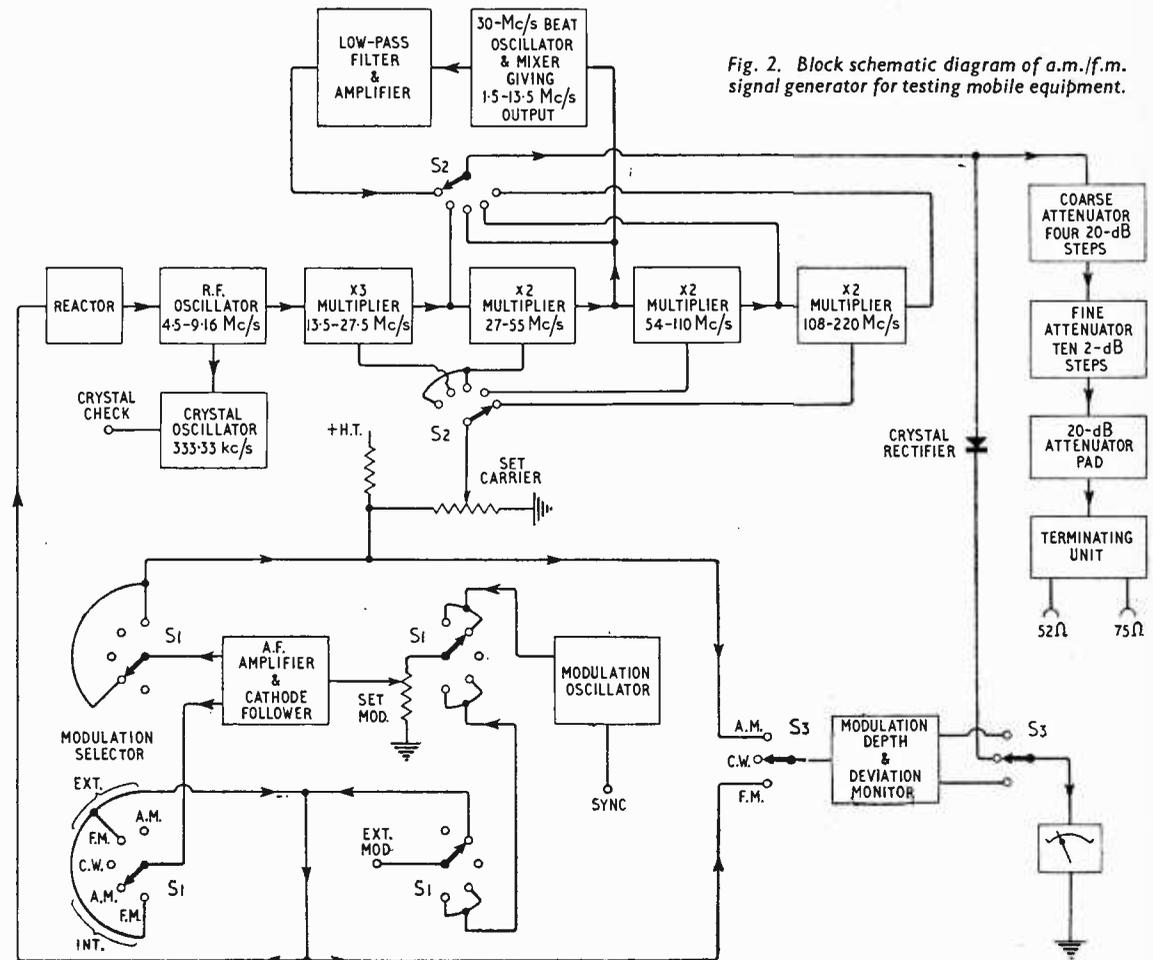
Fig. 2. Block schematic diagram of a.m./f.m. signal generator for testing mobile equipment.
