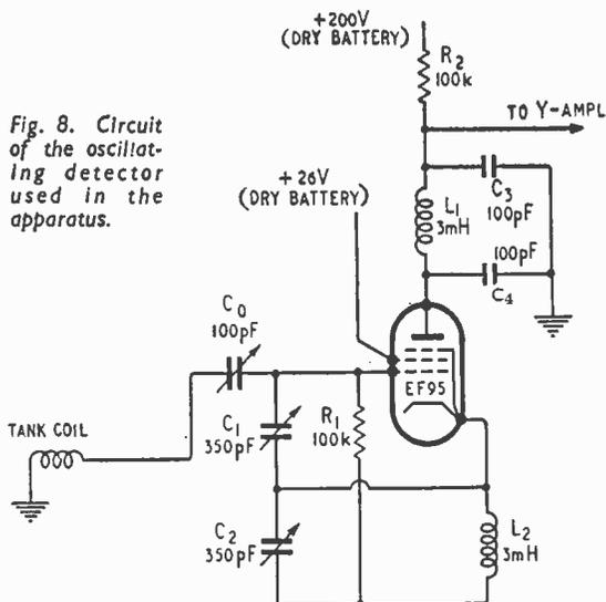
Fig. 8. Circuit of the oscillating detector used in the apparatus.
