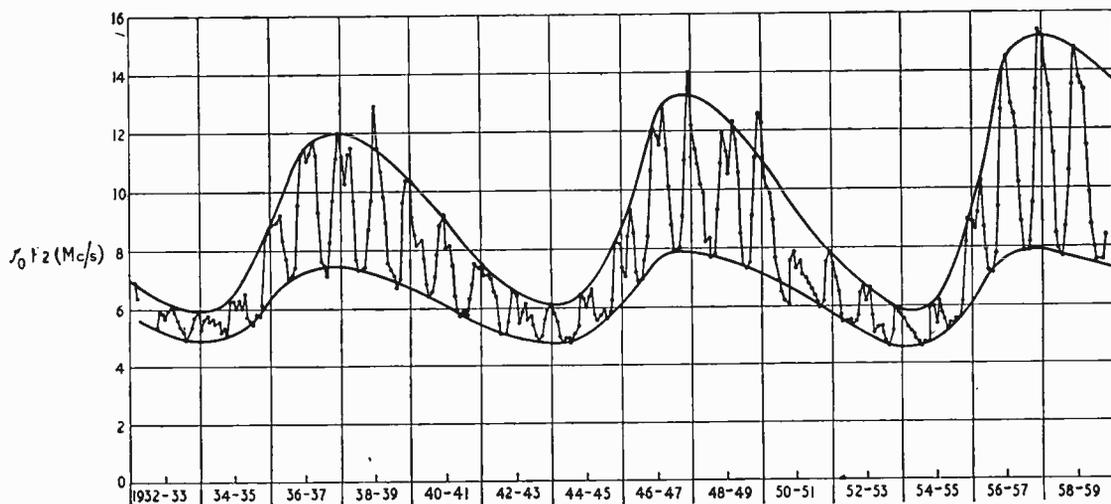
Fig. 2. Measured noon values of  $f_oF_2$  at Slough, 1932-1959
