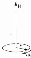
Fig. 4. Showing how the second magnetic field  $H_1$  rotates relative to  $H$ .
