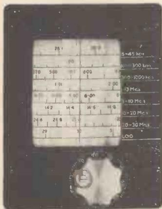
*Main tuning control showing a portion of the seven frequency scales, the coarse and fine logging scales and the movable cursor.*
