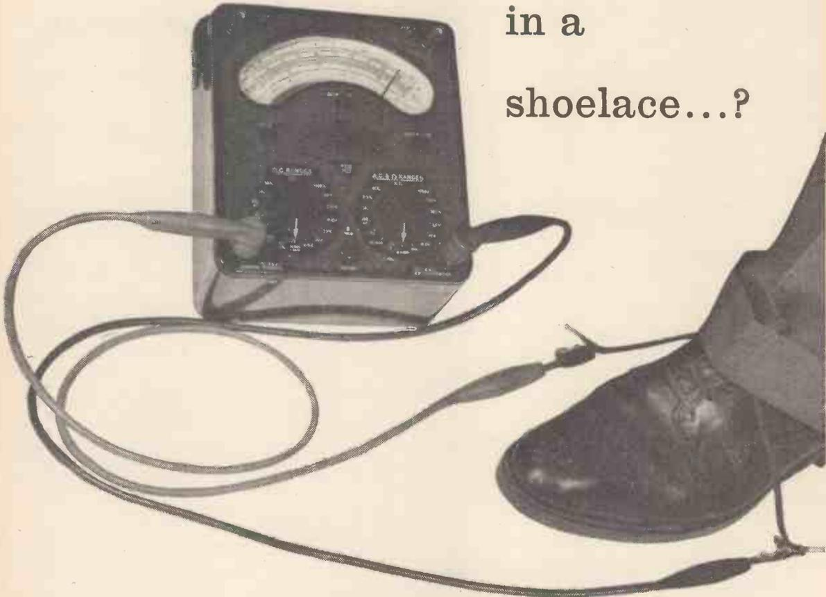
Fanciful? No, because as our photograph proves, a shoelace can be made electrically conducting by impregnating it with "dag"\* colloidal graphite.
