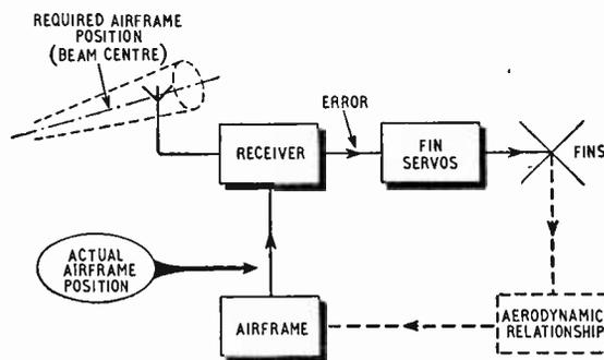
Fig. 6. The beam rider as a servomechanism.
