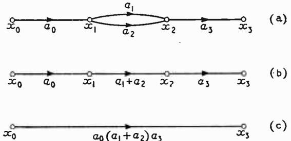
Fig. 3. Simplification with series and parallel branches.
