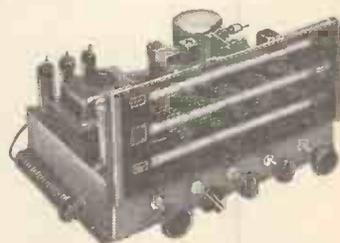
An AM/FM chassis with nine valves and two diodes with push-pull output stage providing 6 watts. Full VHF, medium and long wavebands with automatic frequency control on FM and ferrite aerial on AM. Tape record and playback facilities.
