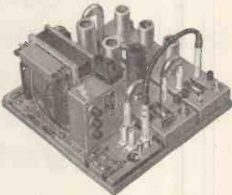
**WIDE BAND REPEATER** Type 12/5A with Repeater Type 5FM incorporated (covering together Bands 1 and 2)
