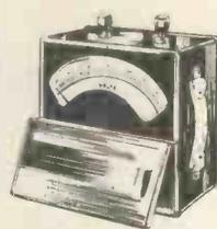
**LABORATORY PRECISION VOLTMETER.** Brand new in polished teak case. Moving iron instrument reading D.C. or A.C. 0-160 volt on 8 in. mirror scale. Accuracy 2% £4/19/6 each. P. & P. 3/6.
