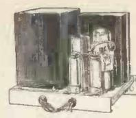
**MAINS POWER SUPPLY UNITS** Potted and sealed transformer and choke by famous maker. Mounted on metal chassis 6 1/2 x 7 1/2 in., complete with 5Z4 rectifier valve and full smoothing.
