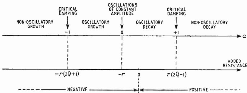
If we take a practical case, for instance a tuned circuit having a Q of 50 and resonating at 1 Mc/s when the capacitance is 150 pF, the resistance required for dead-beat growth of current has to be more negative than (-2000) ohms.
