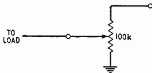
Fig. 9. Coefficient-setting potentiometer
