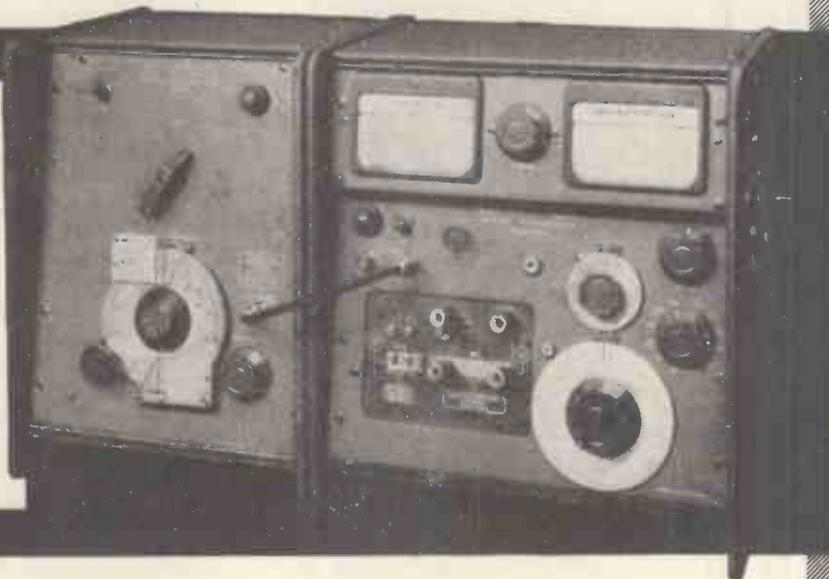
HERE FOR THE FIRST TIME is a single Q Meter covering the range a.f. to v.h.f. Q is directly indicated from 5 to 500 by a 3-range transducer-stabilized valve-voltmeter, and a second meter shows Q multipliers from  $\times 0.9$  to  $\times 2$ . Minimum test-circuit capacitance is  $7.5\mu\text{F}$  at all frequencies.
