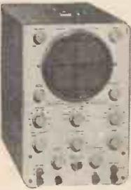
Laboratory quality at utility oscilloscope price and ease of assembly make this kit of outstanding value. Vertical frequency response 3 c/s to 5 Mc/s.,  $\pm 1.5$  dB.  $-5$  dB., sensitivity 10 mV. per cm. at 1 kc. Horizontal frequency 1 c/s. to over 400 kc. ( $\pm 1$  dB. up to 200 kc.). The Heath patented sweep circuit functions from 10 c/s to 500 kc. In five ranges giving five times the usual sweep of other 'scopes.
