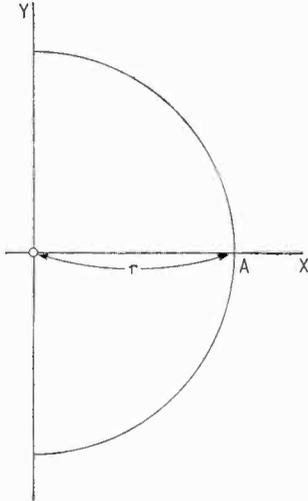
Below: Fig. 5. When  $x$  exceeds  $r$ , that part of the graph is "imaginary," but with the aid of a  $j$  takes this form, with a mirror image symmetrically on the left.
