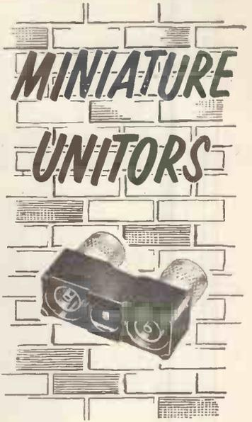
"Belling-Lee" Miniature Unitors have been designed round a "brick" of unit area (0.990" x 0.366"), having a central fixing point. A number of "standard bricks" is available employing different arrangements of contacts of two basic sizes, rated at 5 and 10 amp. respectively, for working voltages up to 2,000 V. peak. A common feature is the central earthing connector which also acts as a polarising key, as well as providing the fixing to chassis. Contacts are silver or gold plated.
