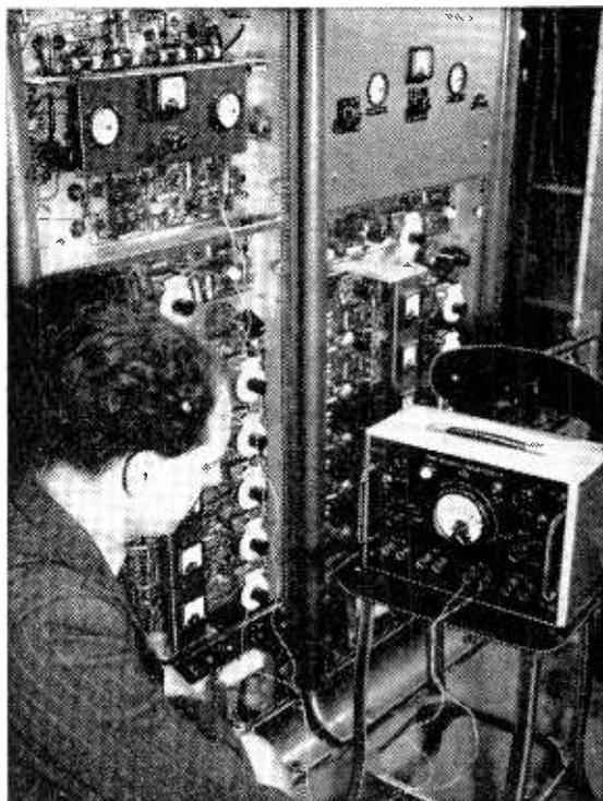
Fig. 4. Using the Airmec time interval meter to measure the duration of the 60 millisecond transmission at  $6f + 60$  c/s on the Master station. The Airmec timer is triggered by the anode circuit of the appropriate drive valve.
