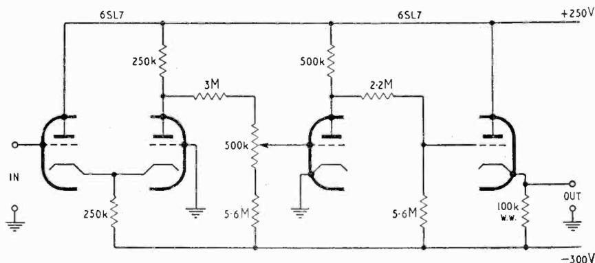
Fig. 7. Connections for using an operational amplifier as a summing element.
