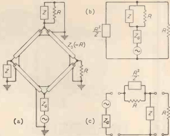
An article in the April issue of **ELECTRONIC TECHNOLOGY** describes v.h.f. and higher-frequency filter networks employing closed rings of transmission line or waveguide. The theory is developed enabling them to be related in a simple way to lumped-impedance networks and to provide a method of analysing well-known arrangements and designing new networks.
