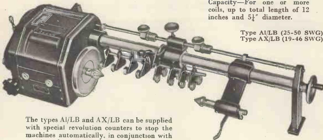
The types A1/LB and AX/LB can be supplied with special revolution counters to stop the machines automatically, in conjunction with a solenoid mechanism on the A.C. motor, when the required number of turns have been wound.
