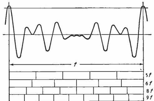
Fig. 2. The combination of all four frequencies sent out by each station in turn generates this lane identification pulse at the receiver. The main peaks, at  $f$ , create a coarse navigational pattern to reduce ambiguity.
