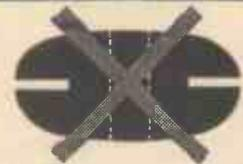
In the conventional grommet, only one thickness of plate and only one size of cable can be accommodated. No effective seal is afforded by the parallel groove.
