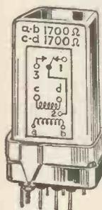
**MINIATURE MOVING COIL DIFFERENTIAL RELAY.** Two coils 350 ohms each. Operating current minimum 140 microamp., nominal 400 microamp, maximum 8 millamp. One pole two way, or centre stable. Two way contact current 100 mA. at 50 V. A.C. or D.C. Size 1 1/4 x 1/2 x 3/8 in. Price 22/6 each.
