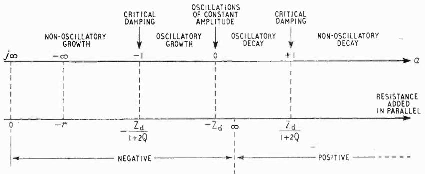
Thus, as for the case of the series-tuned circuit, we can summarize the behaviour in the diagram above.
