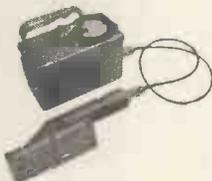
Model PAC-15. Alpha Counter-Scintillation Type. Designed for surveying alpha contamination over a wide range of activity levels and under wide temperature variations. Consists of a probe, a single conductor 36 inch shielded cable, and rate meter. All units waterproof. Controls and scale selector, etc., are conveniently grouped around handle and can be operated by one finger of the carrying hand even when wearing protective gloves.
