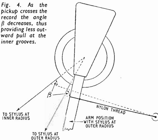
This is useful as a rough guide to the weight needed at a given distance from the pivot or to the distance from the pivot needed for a given weight.
