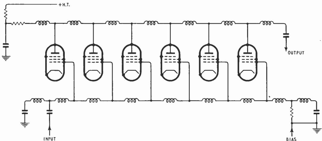
Fig. 9. Part of circuit of Cossor distributed amplifier. Output feeds similar circuit to give gain of 20dB from 40 to 220Mc s.
