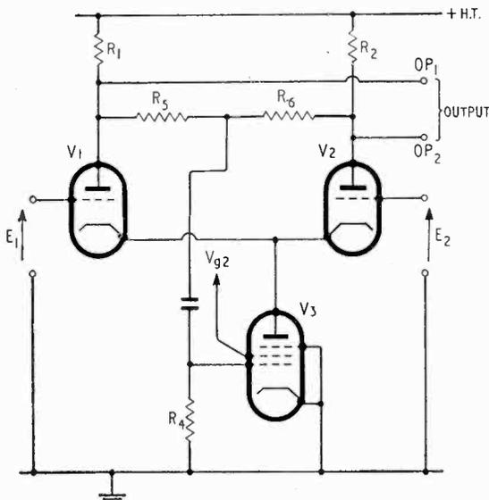
Fig. 3. Long-tailed pair with feedback.
