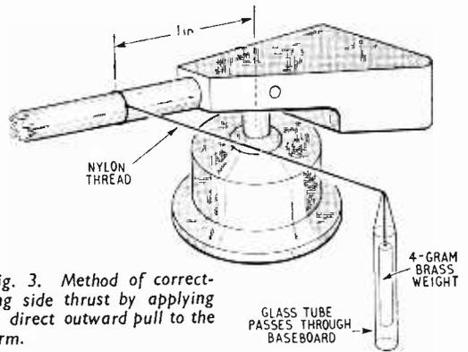
Fig. 3. Method of correcting side thrust by applying a direct outward pull to the arm.
