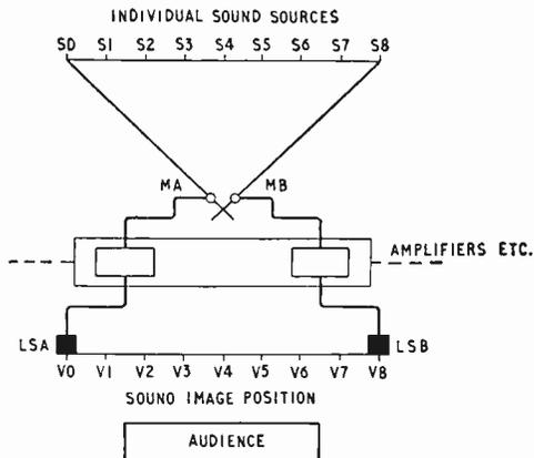
Fig. 20. Simplified requirement of a two-channel system.
