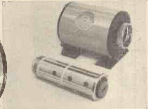
BA16-10 demounted from electromagnet focusing system
