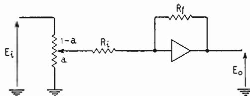
Fig. 3. Potentiometer used for multiplication by a constant.
