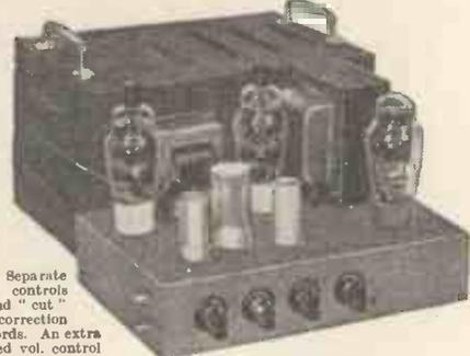
Separate Bass and Treble controls give both "lift" and "cut" with ample tone correction for long playing records. An extra input with associated vol. control is provided so that two separate inputs such as mike and gram, etc. can be simultaneously applied for mixing purposes. AN OUTPUT SOCKET WITH PLUG IS INCLUDED FOR SUPPLY OF 300 v. 20 mA. and 6.3 v. 1.5 A. FOR A RADIO FEEDER UNIT. Price in kit form with easy-to-follow wiring diagrams.
