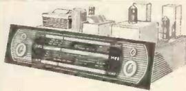
VHF/FM 87-101 Mc/s., Valve line-up ECC85, ECH81, EF89, EM61, EABC80, EL84, suitable for use on 200/250 v. A.C. mains. Dimensions 15 1/2 wide, 12 in. high, 4 1/2 in. deep.
