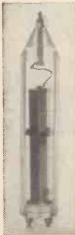
Left: Brush 2-kV piezoelectric transformer.
