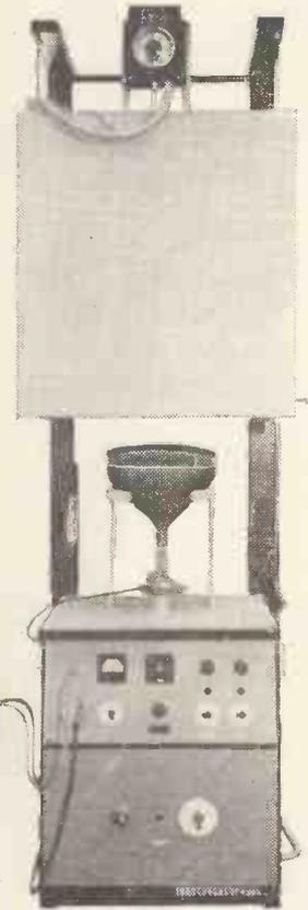
Single position C.R.T. Pumping Unit complete with vacuum reading, automatic controls, electric seal-off, etc.
