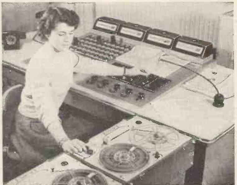
Right: Control centre at Rotterdam, where programmes are selected and monitored. Level indicators for each of the four programmes are at the back of the control desk.
